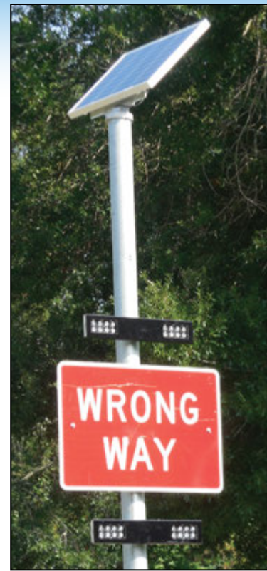
Wrong-way sign with light-emitting diode display.
