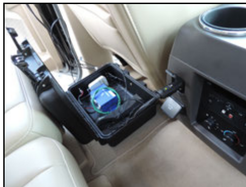
OBU integrated in a small case for easy installation.
