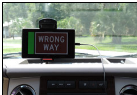
Alert to vehicle driving in the wrong direction.
