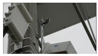
During the TERL's first and second performance tests, a small camera was temporarily installed on the same pole as the detection devices and real-time video of traffic was recorded across the six lanes of traffic. An accurate determination of volume, occupancy, and speed was the goal as the test was setup. The evaluation purpose is to verify conformance with
