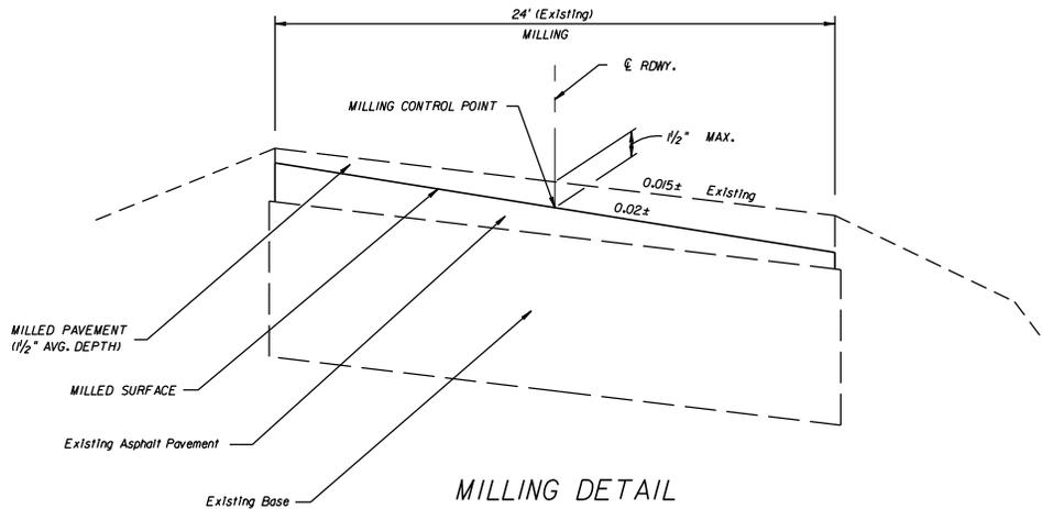
WHEN CROSS SLOPE CORRECTION IS NECESSARY SPECIAL MILLING AND LAYERING DETAILS MUST BE PROVIDED TO SUPPLEMENT TYPICAL SECTION. THE NEED FOR AND LOCATION OF PROFILE GRADE POINTS WILL DEPEND ON SITE SPECIFIC CONDITIONS.
