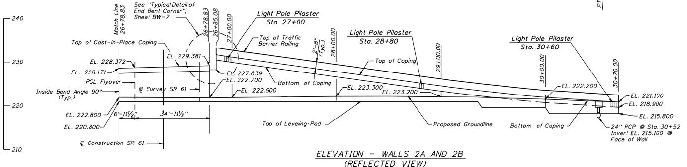
**ELEVATION - WALLS 2A AND 2B (REFLECTED VIEW)**
