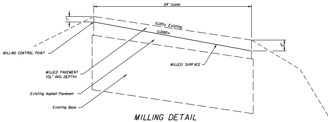
WHEN CROSS SLOPE CORRECTION IS NECESSARY SPECIAL MILLING, OVERBUILD AND LAYERING DETAILS MUST BE PROVIDED TO SUPPLEMENT TYPICAL SECTION. THE NEED FOR AND LOCATION OF PROFILE GRADES POINTS WILL DEPEND ON SITE SPECIFIC CONDITIONS.
