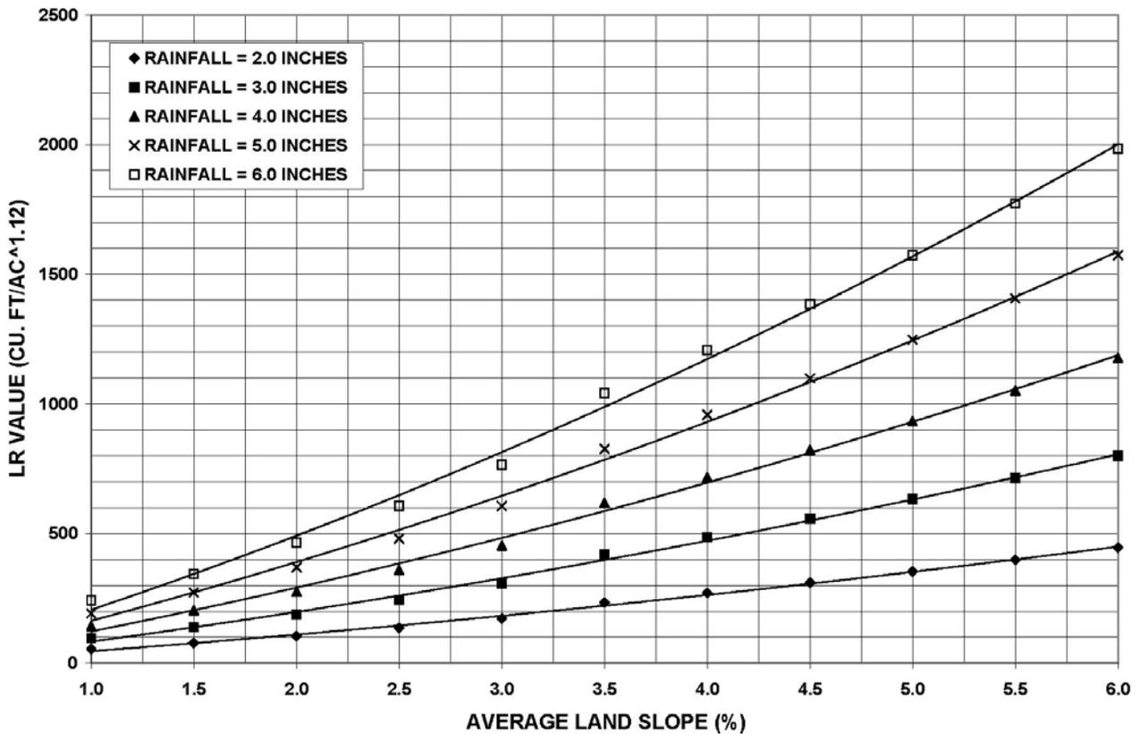
Figure IV-11: Hydrologic Type D Soils Loading Ratio Graph
