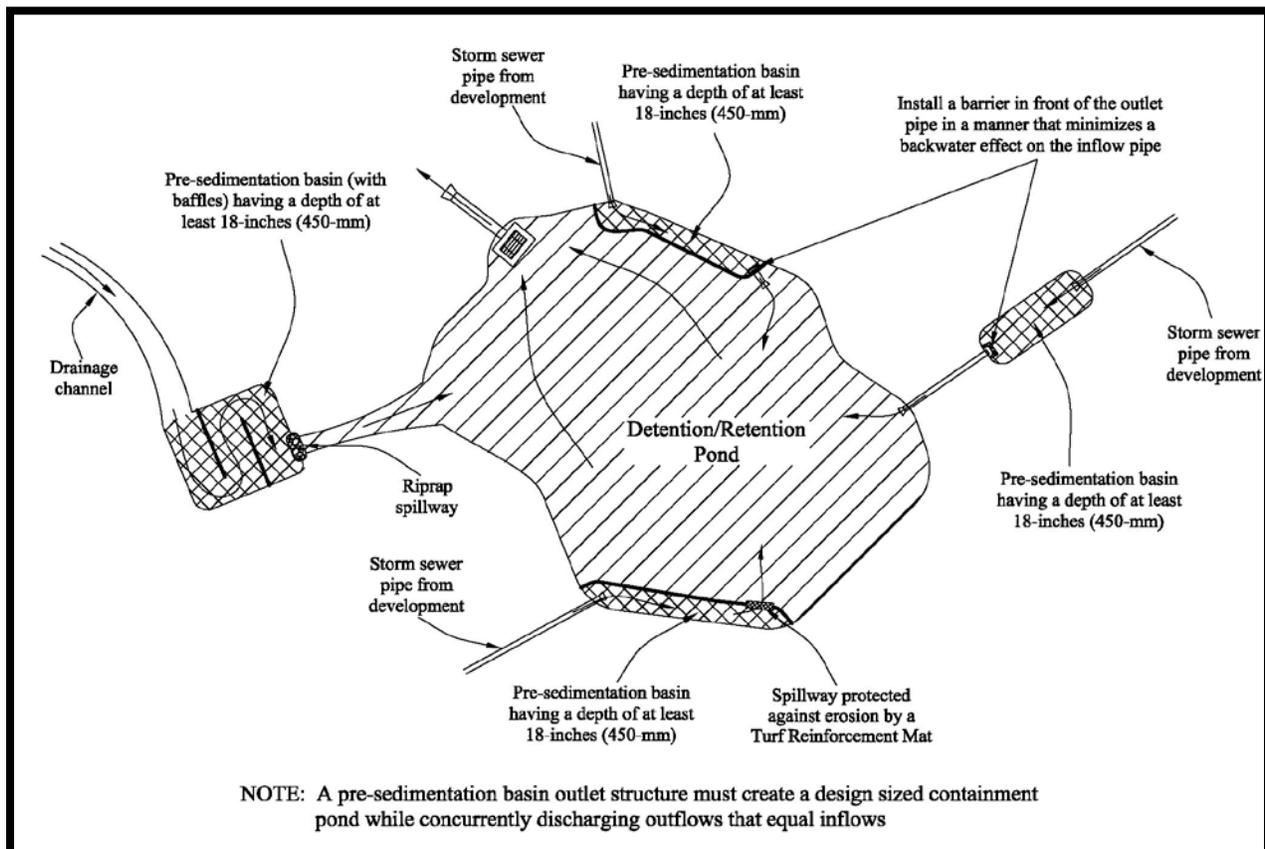
**Figure IV-7: Conceptual Pre-Sedimentation (a.k.a. Forebay) Basins (No Scale)**
