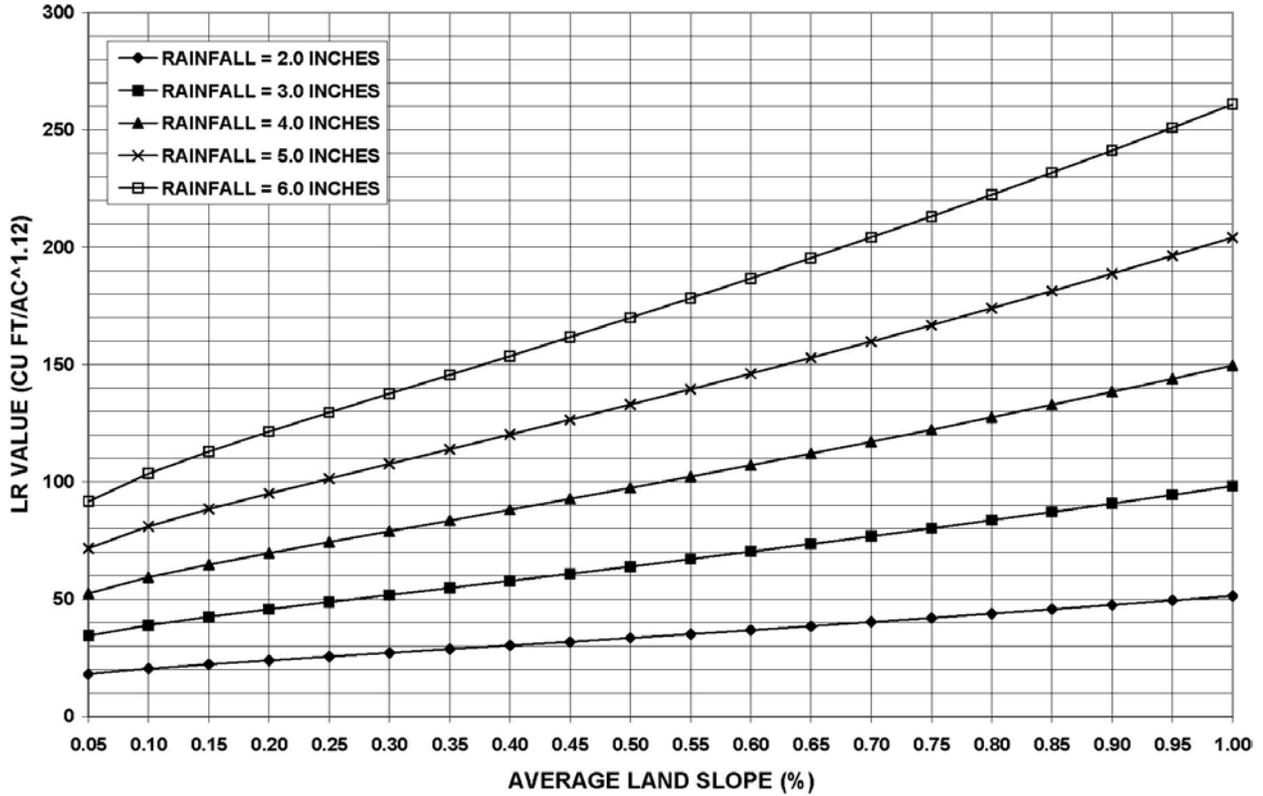
HYDROLOGIC TYPE C SOIL LOADING RATIO VALUES WHEN K = 0.43 AND CN = 91
