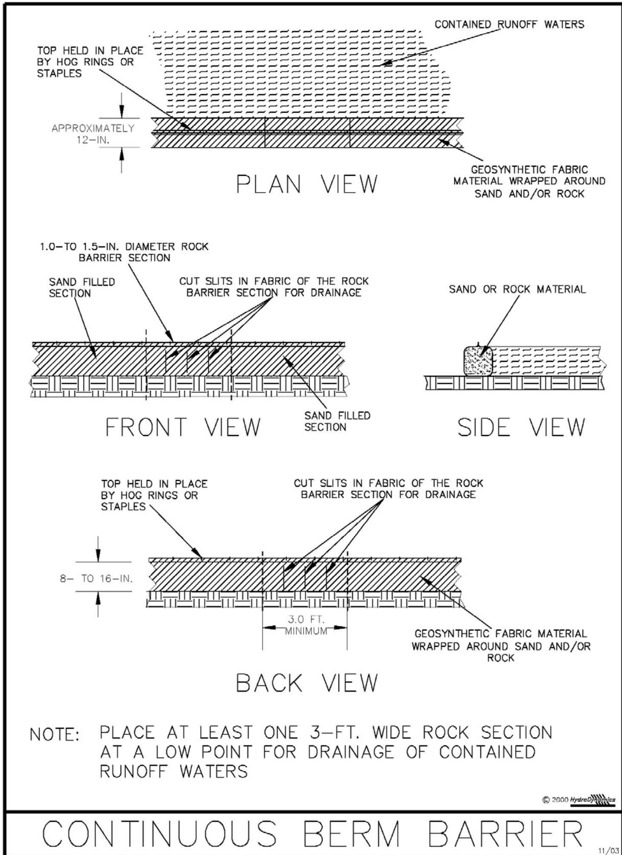
**Figure V-7: Illustration of a Continuous Berm Barrier**
