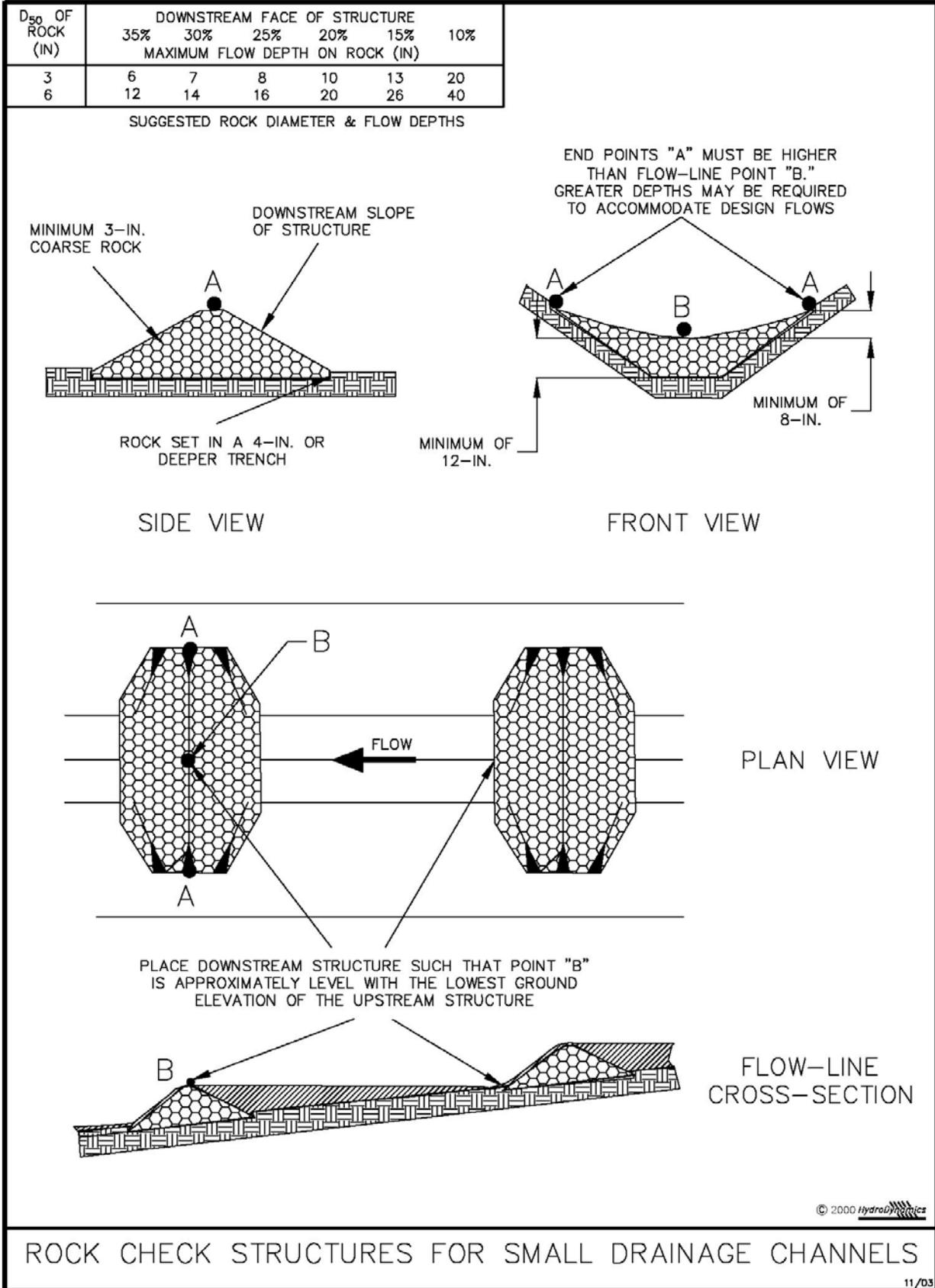
**Figure III-11: Rock Check Structures in Small Drainage Channels**
