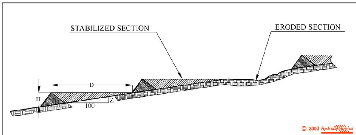
**Figure III-8: Placement of Check Structures for Channel Stability**
