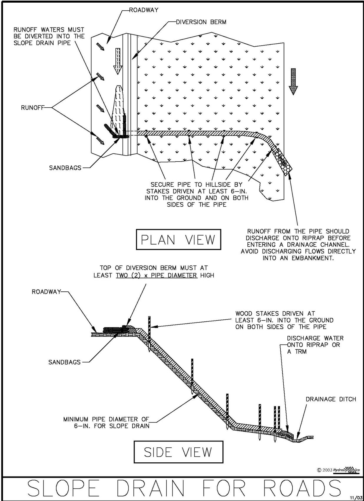
Figure III-6: Installing a Slope Drain for Road Embankments
