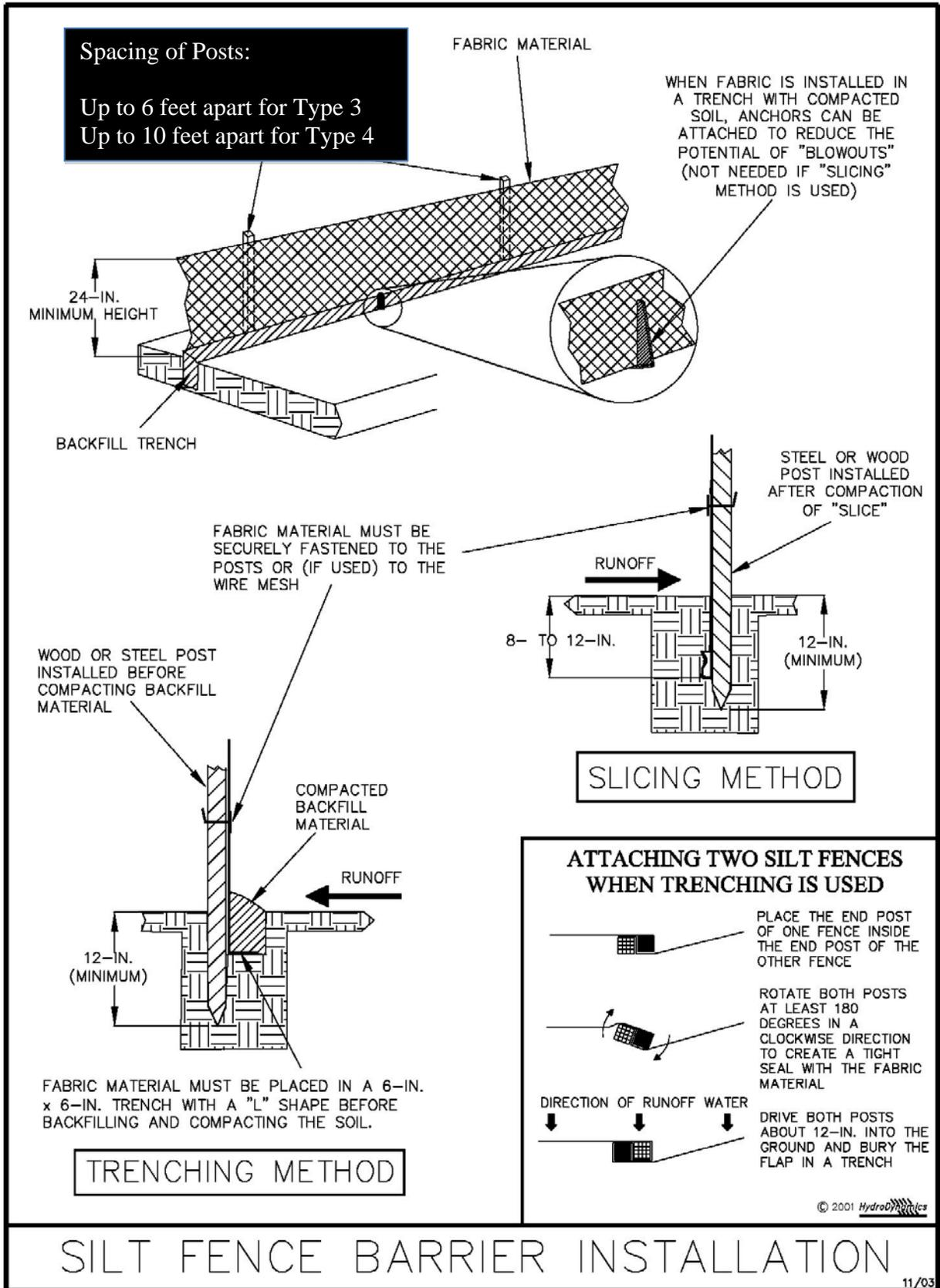
Figure V-2: Illustration of a Silt Fence Barrier
