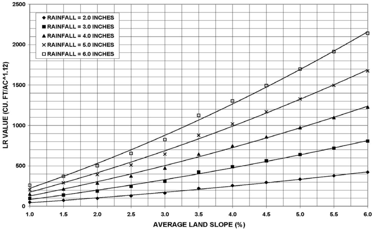
Figure IV-10: Hydrologic Type C Soils Loading Ratio Graph
