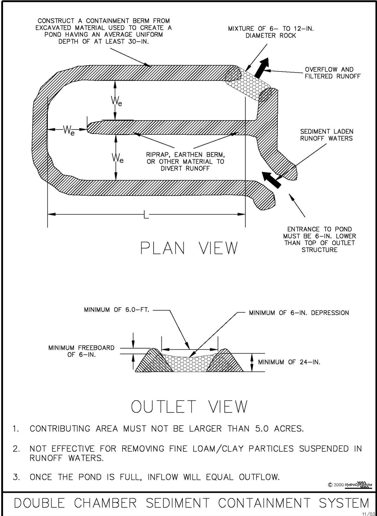
Figure IV-14: Illustration of a Double Chamber SCS
