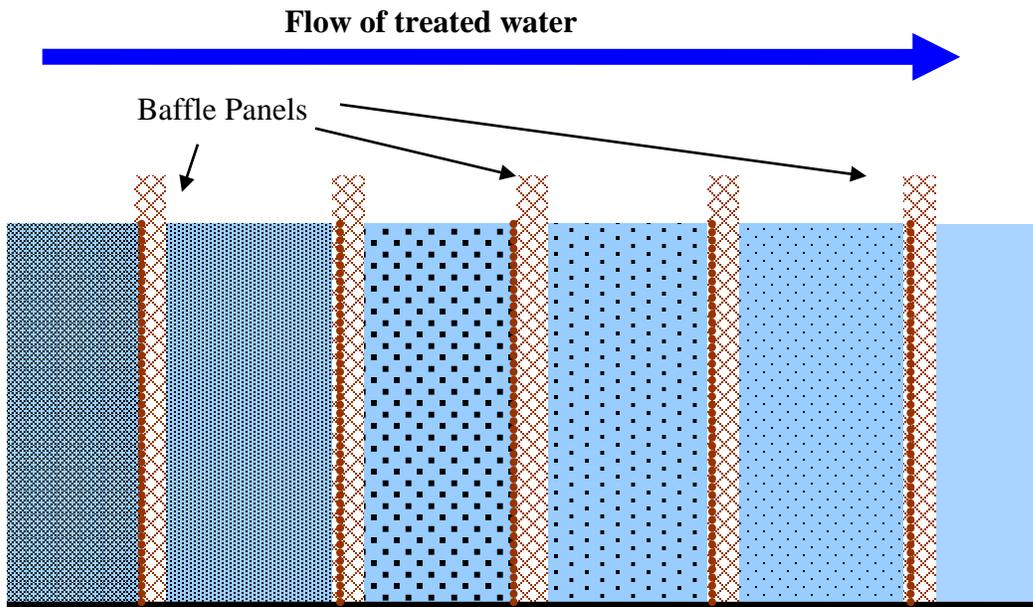
Figure AIII-23: Polymer-enhanced Baffle Grids.
