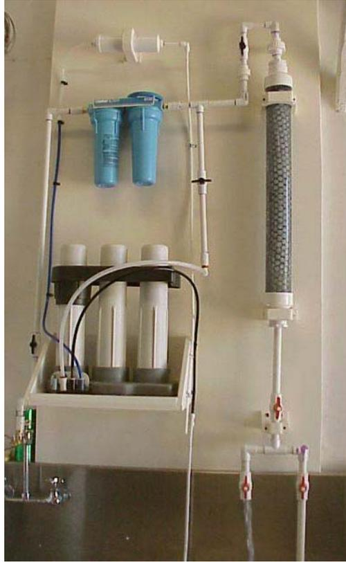
Figure AIII-1: Polymer Log dosage sampling device.
