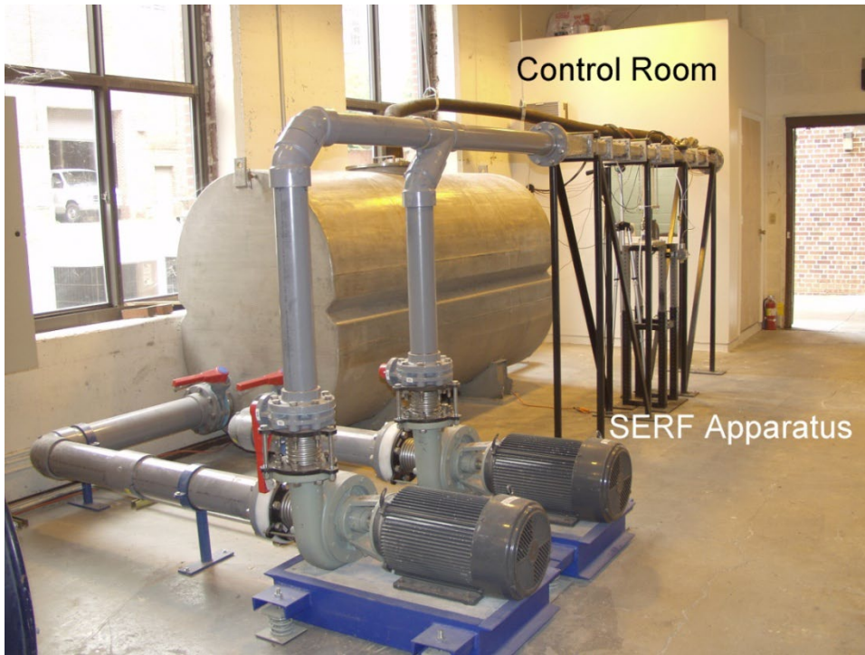
Figure 5-4 S ediment E rosion R ate F lume (SERF) located in a Civil Engineering Laboratory at the University of Florida.
