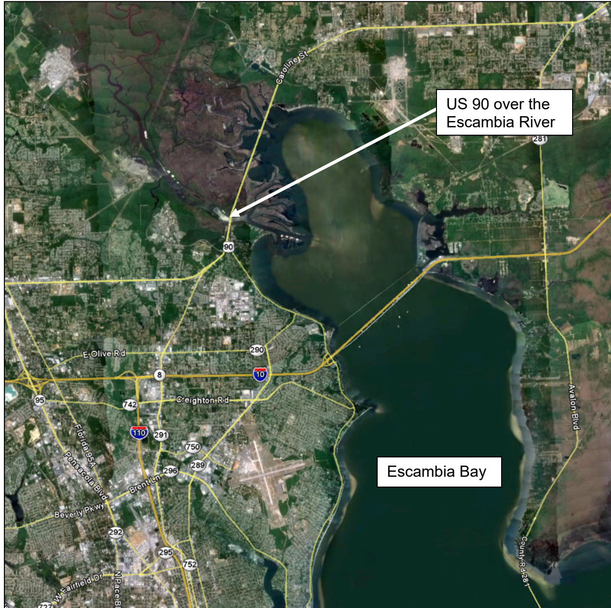
Figure 5.1-2: Example of a Bridge Requiring both Riverine and Tidal Analyses (US-90 over Escambia Bay)
