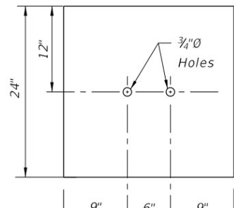
**1/4" Steel Plate, Galvanized SOIL PLATES**
