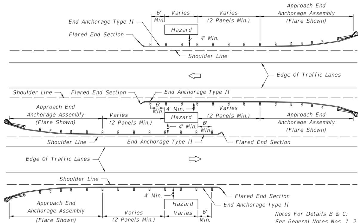
Median Guardrail Applications Shown Are For Locations Where Approach End Anchorage Assemblies Are Outside Of The Opposing Roadway Clear Zone.
