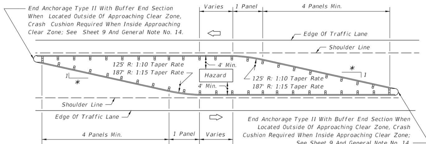
This Guardrail Configuration Applies Where Approach End Anchorage Assemblies Cannot be Located Outside Of The Opposing Roadway Clear Zone.
