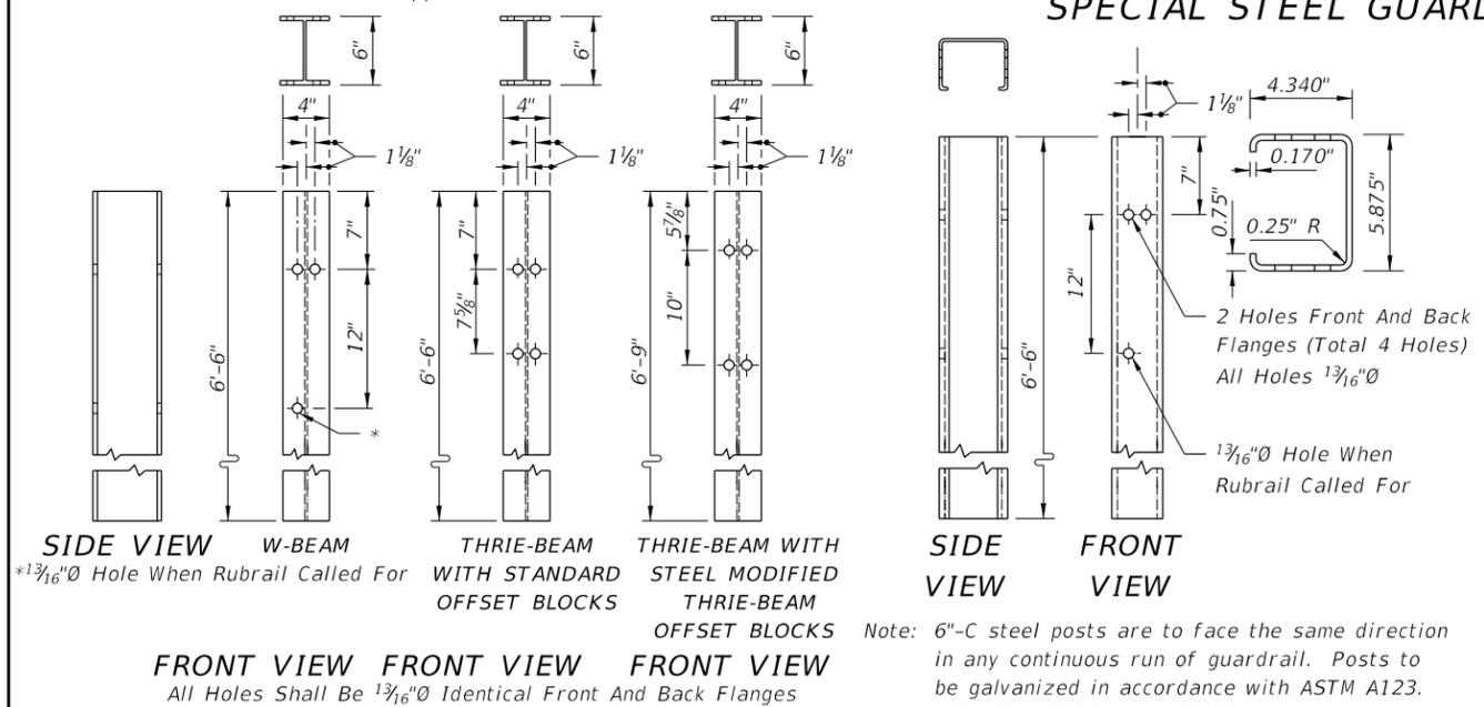
Note: W6x8.5 or W6x9 steel posts may be either rolled or welded structural shapes conforming to or exceeding the design properties of ASTM A6/A6M. Welding shall be in accordance with the requirements of ASTM A769/A769M. Posts shall be cut to length and the ends seal welded between web and flange before galvanizing. Posts to be galvanized in accordance with ASTM A123.
