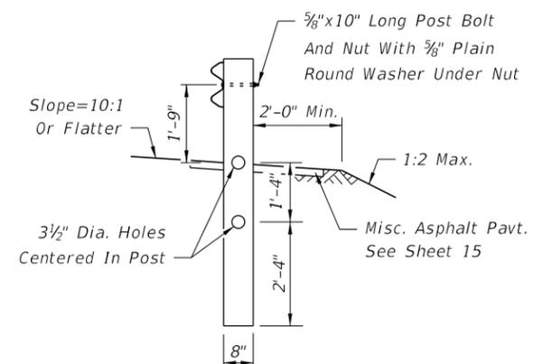
Note: To be constructed when flares and transitions or standard radial returns can not be applied. See Sheet 12.
