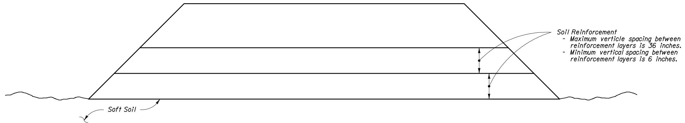
GEOSYNTHETIC REINFORCED FOUNDATIONS CONSTRUCTED ON SOFT SOILS
