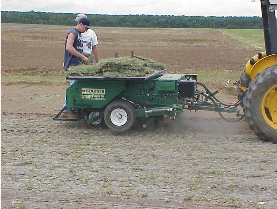
Figure 12. Sprigging of turfgrass using a sod-to-sprig machine.
