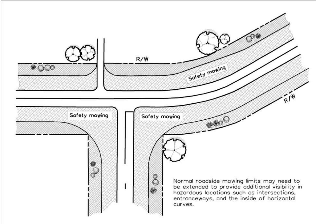
Figure 24. Safety mowing limits.
