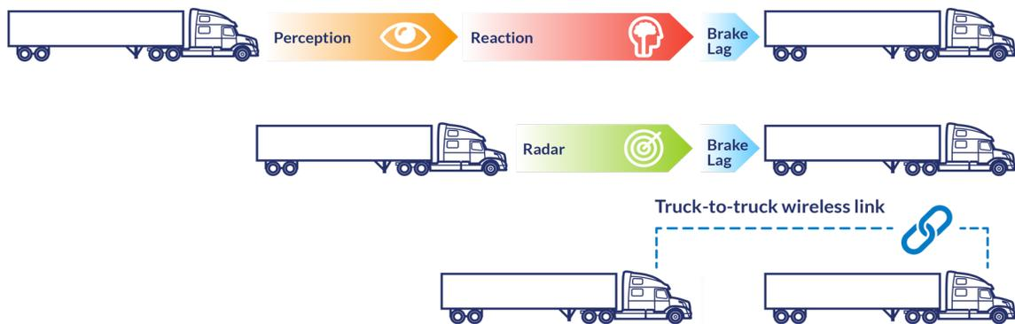
Figure 4: Brake Application Timing w/ Coordinated V2V Operation
