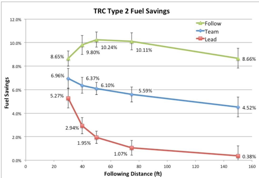
Figure 5: Percent Fuel Saved from TRC Type II Fuel Economy Testing (Bevly et al., 2017)
