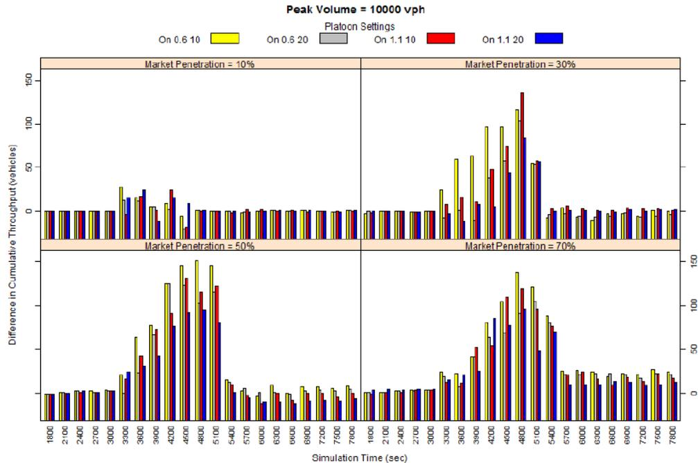
Figure 8: TTI Traffic Simulation Results for Truck Platooning (Kuhn et al., 2017; Figure 21 in original report)
