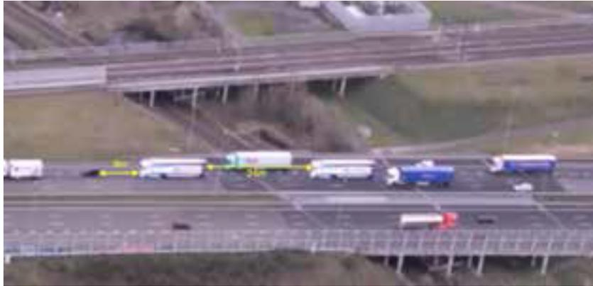
Figure 10: EPTC Overhead Video: Platoon Decouples and Creates a Larger Gap
