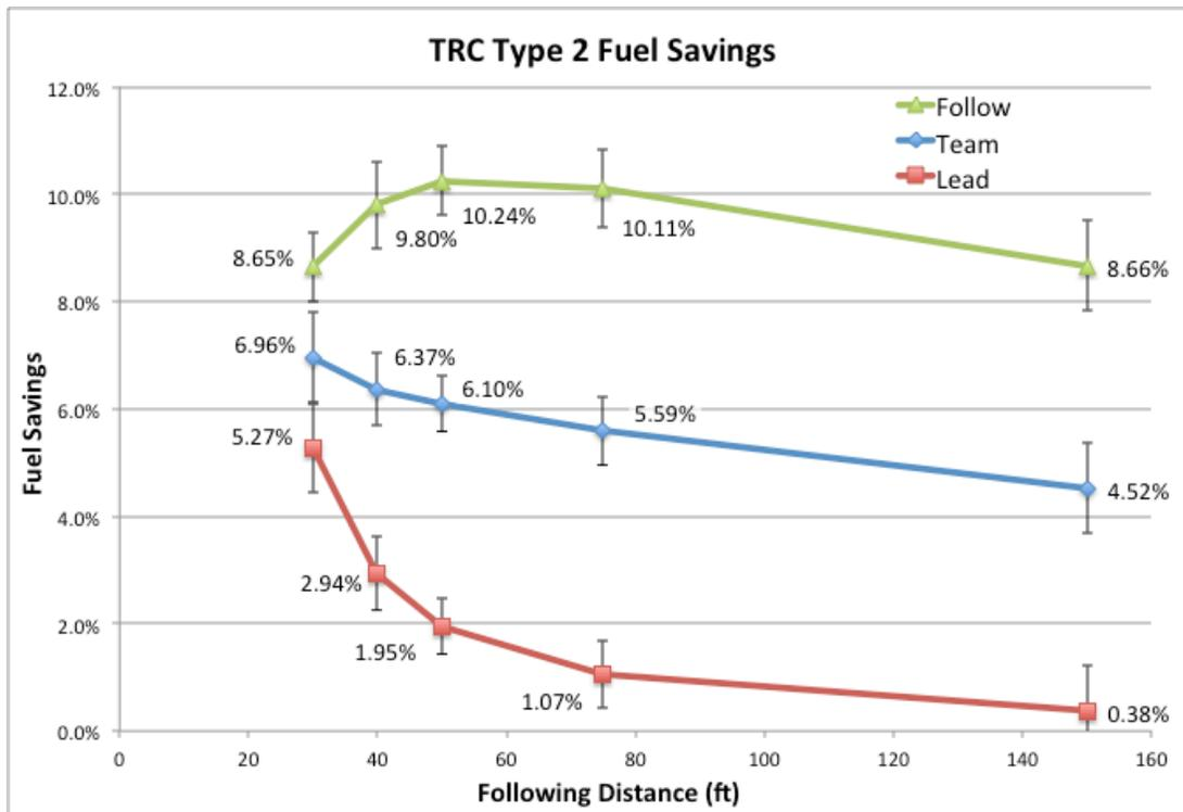
Figure 5: Percent Fuel Saved from TRC Type II Fuel Economy Testing (Bevly et al., 2017)
