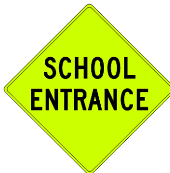
Figure 15-2 School Entrance Warning Sign (FTP 33-06)
