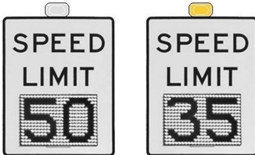
Figure 10-1 Example VSL Speed Limit Signs Under Normal Condition (Left) and Reduced Speed Condition (Right)
