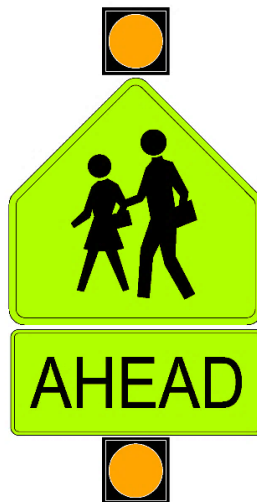
Figure 15-10 School Advance Crossing Sign with Flashing Beacon Assembly Used for Additional School Zone Warning on Multilane Roadways
