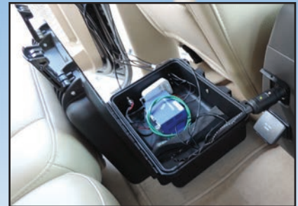
OBU integrated in small case for easy use.
