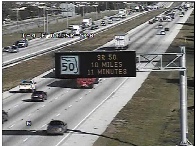
Color DMS as shown through a video feed. (Photo courtesy of FDOT District Five)
