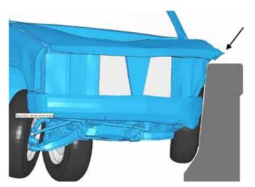
This image from the simulation shows the model truck during impact with the traffic railing. The arrow shows the Zone of Intrusion, the region beyond the plane of the traffic railing into which the impactdeformed vehicle intrudes. The profile of the traffic railing is characteristic of the F-shape barrier.
