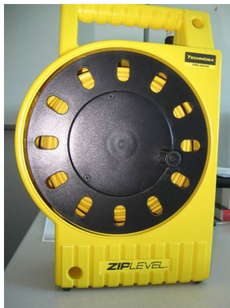
Figure 1. ZipLevel Pro 2000 High-Precision Model
