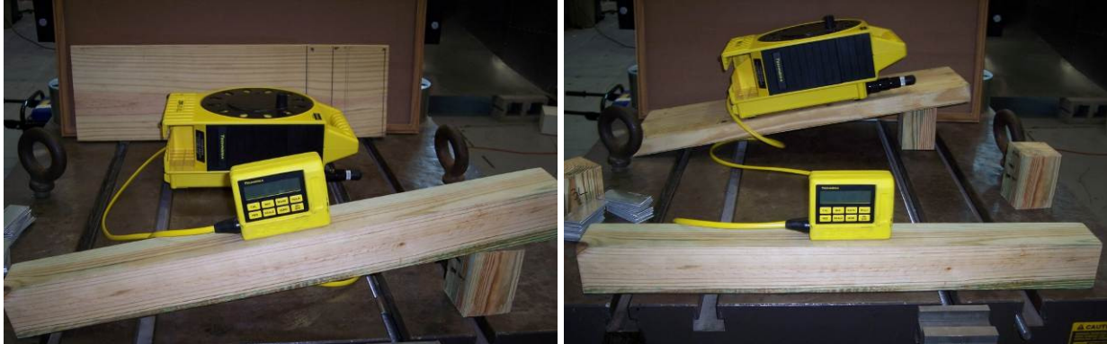
Figure 13. Test B1 (left): the measurement module is raised at a fixed angle, Test B2 (right): the base module is raised at a fixed angle.
