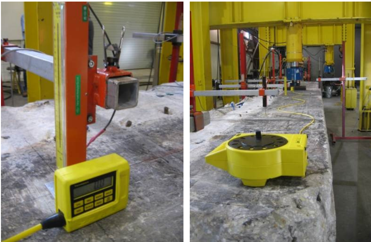
Figure 22. Placement of the measurement module (left) and the base module (right) in the experiment
