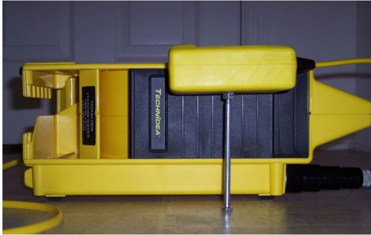
Figure 7. Temperature calibration: to raise the module against a flat surface
