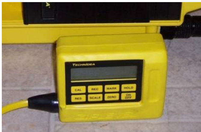
Figure 6. Initial orientation of the measurement module when calibrating for the temperature change
