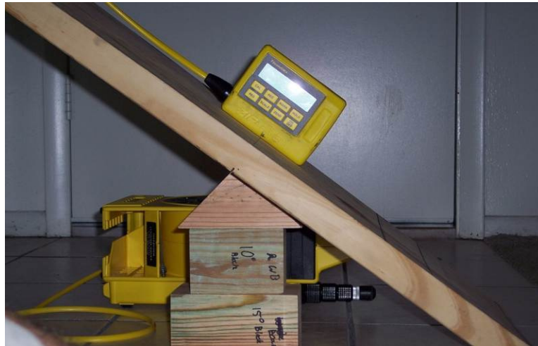
Figure 17. Test C: rotational testing set-up (rotated right). The base module was rotated similarly.
