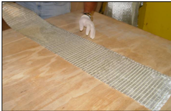
Figure 52 – Glass mat cut to size
