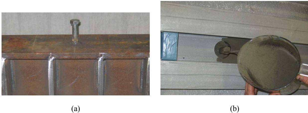
Figure 41 – Specimen A_N (a) stud and beam assembly and (b) grout pour into pocket
