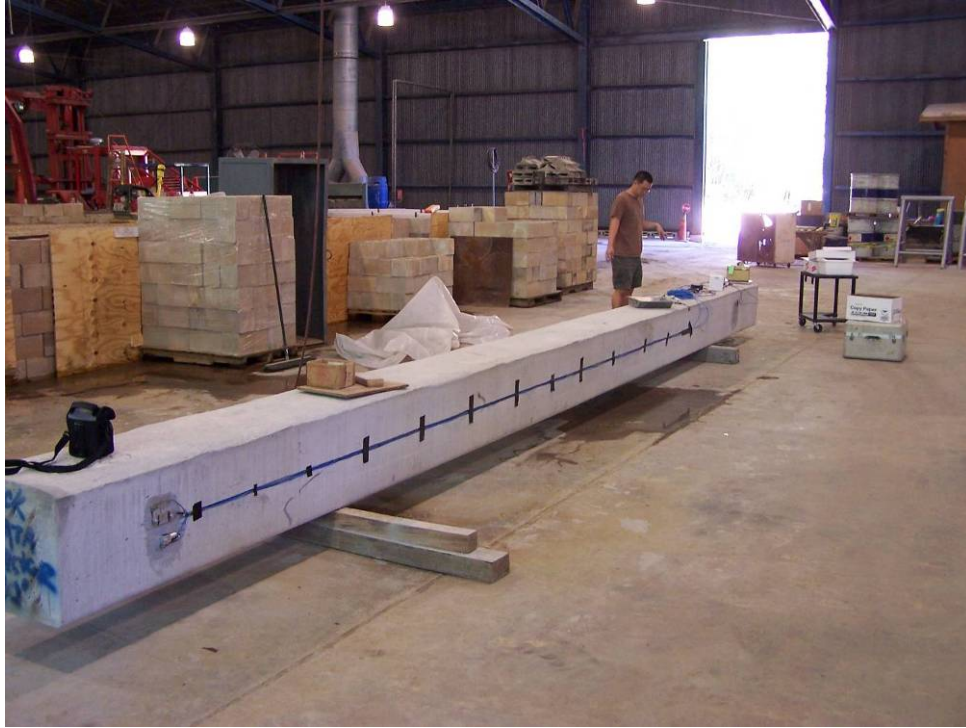
Figure 5-4. 18-in \times 18-in \times 30-ft internally and externally instrumented pile at top and bottom.
