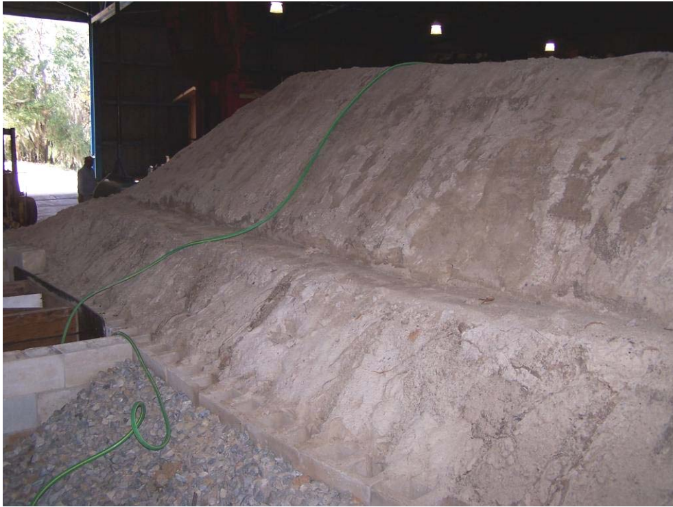
Figure 5-5. 18-in \times 18-in \times 30-ft embedded horizontally in 15-ft high by 45-ft long sand embankment.
