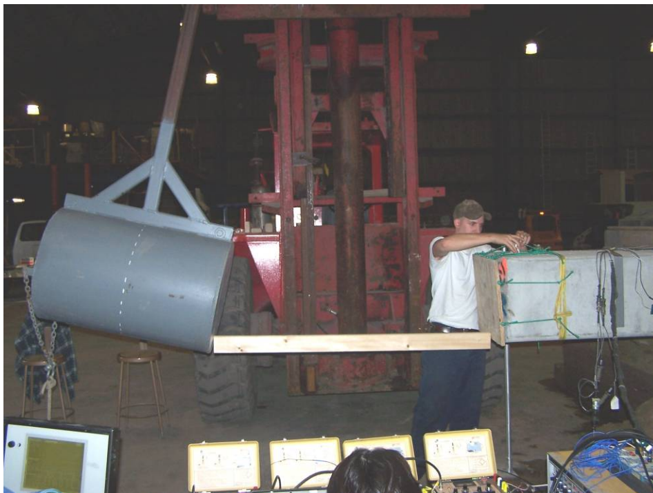
Figure 3-8. Setting up for dynamic impact of 18-in \times 18-in \times 30-ft embedded pile.
