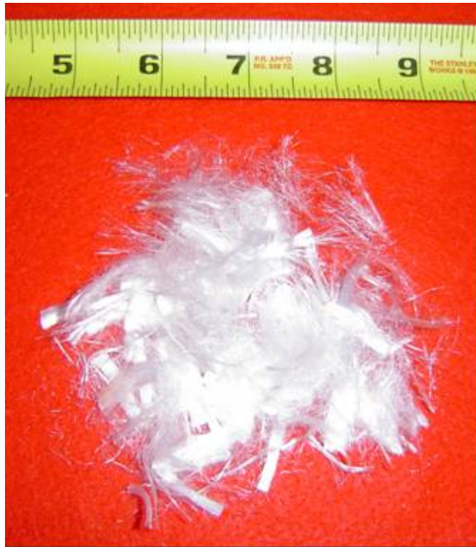
Figure 28. Synthetic fibers used in BND topping
