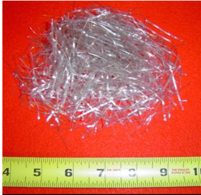
Figure 27. Synthetic fibers used in SYN topping
