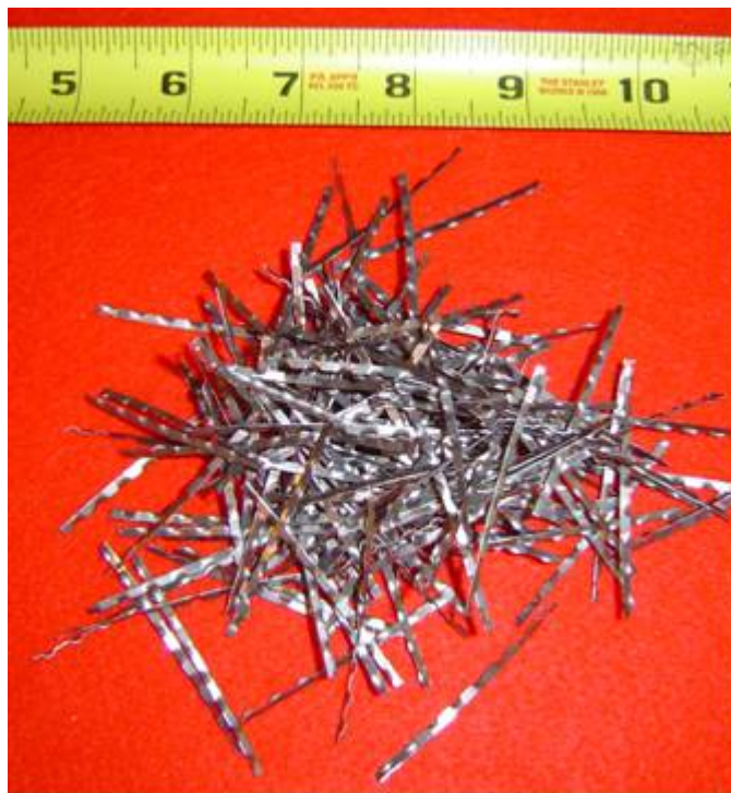
Figure 29. Steel fibers used in BND and STL toppings
