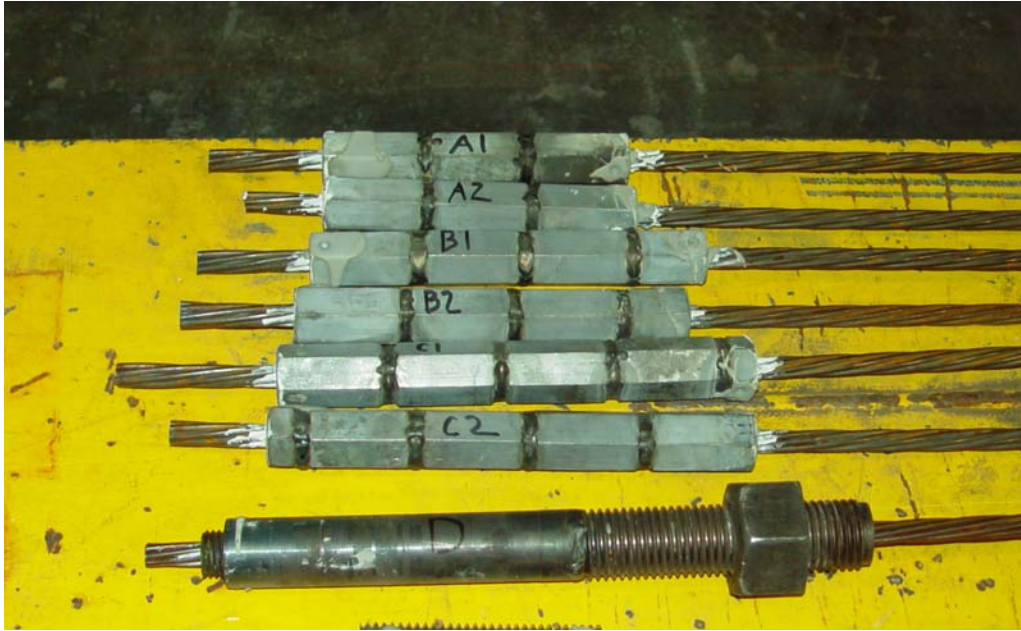
Figure 3: Anchor Device after Grouting - Test 1 Series
