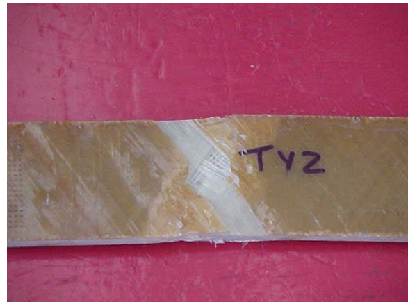
Figure 4.5 Failure Modes of White and Yellow Coupons in Tension
