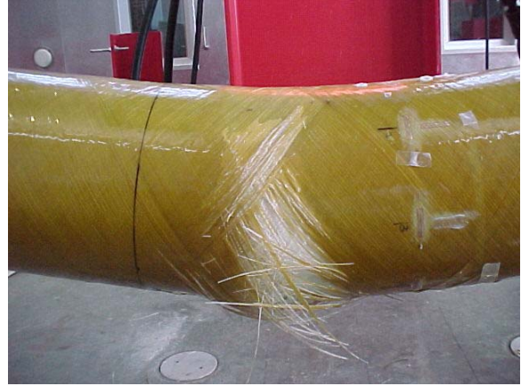
Figure 4.4 Failure Modes of White and Yellow Tubes
