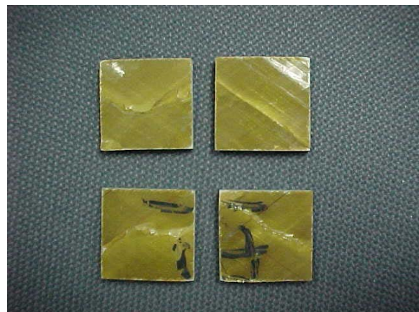
Figure 4.6 Failure Modes of White and Yellow Coupons in Compression
