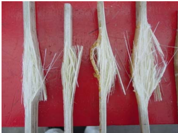
Figure 4.5 Failure Modes of White and Yellow Coupons in Tension
