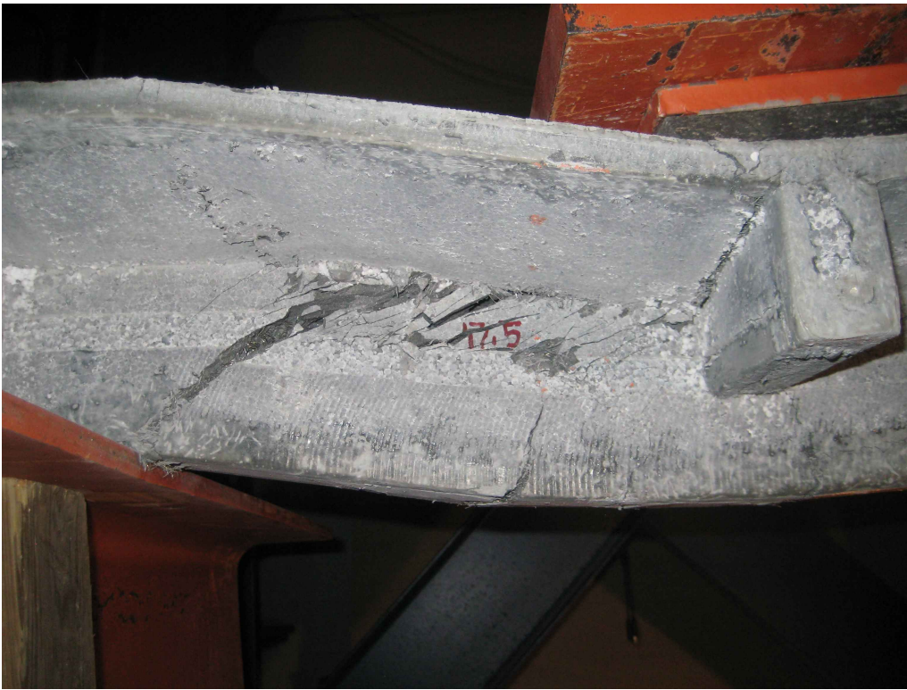
Figure 3.40 Shear Cracks in Specimen 1T1S with Tapered Flange
