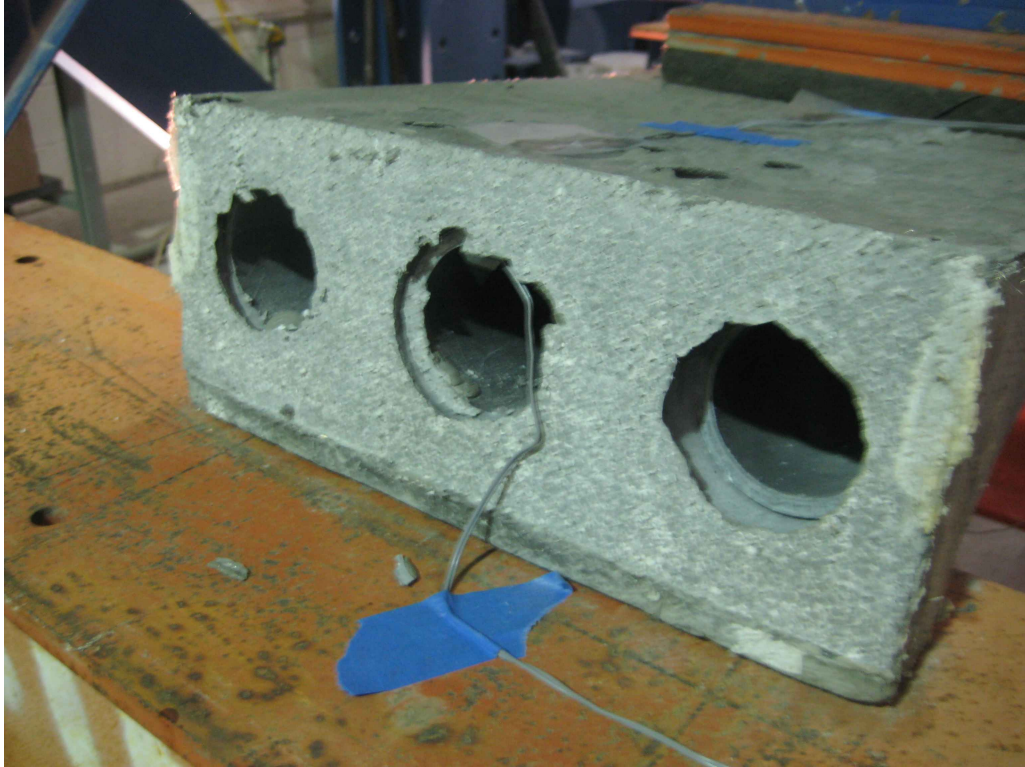
Figure 4.20 Slippage of FRP Tubes in Tapered Section Ductal®-FRP Deck Specimen
