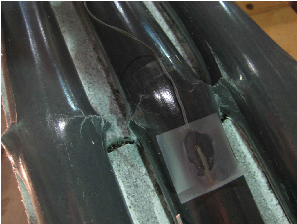
Figure 4.19 Un-cracked Tension Face of Tapered Section Ductal®-FRP Deck Specimen
