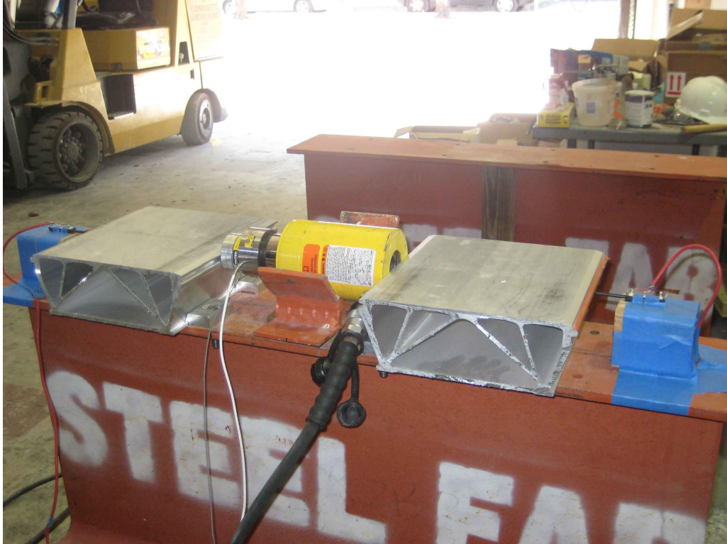
Figure 2.23 Test Setup for the Clamps Shear Test
