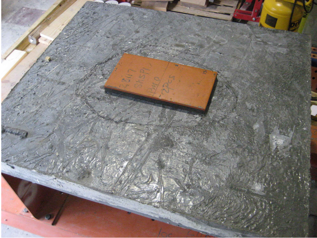
Figure 3.66 Top View of Punching Shear Pattern in Specimen 4T1S
