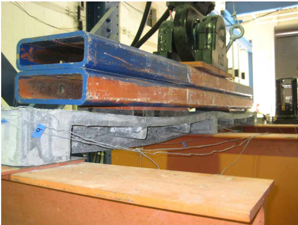
Figure 3.75 Deformed Shape of Specimen 1T2S at 55 kips
