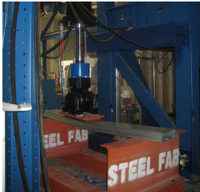
Figure 2.16 Test Setup for Simple-Span Inverted Panel
