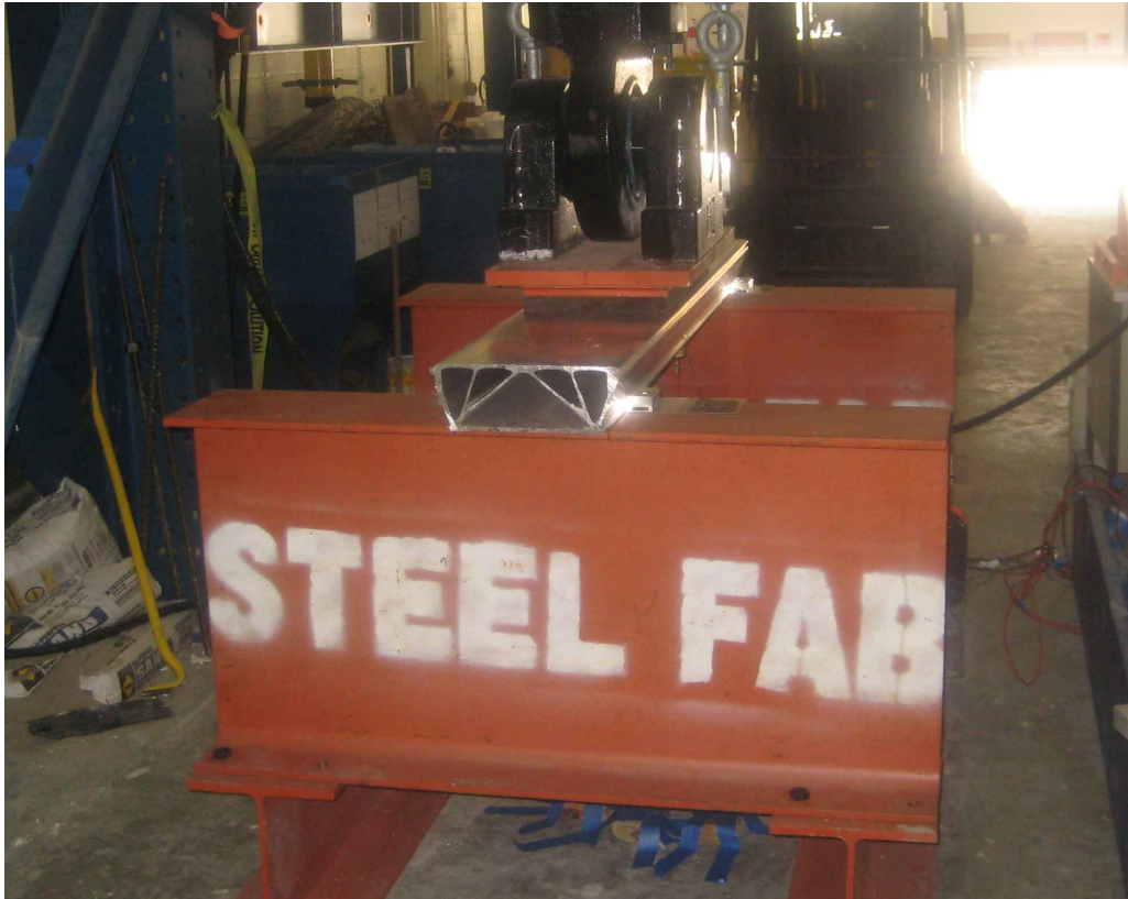
Figure 2.7 Test Setup for Simple-Span Panel
