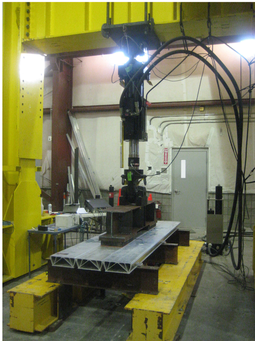
Figure 2.38 Fatigue Test Setup at FDOT Structures Lab
