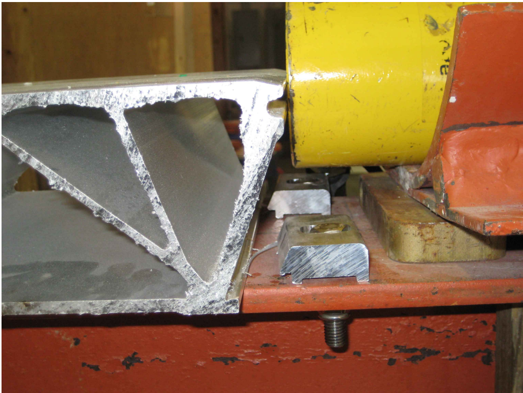
Figure 2.24 Failure of Aluminum Deck Edge
