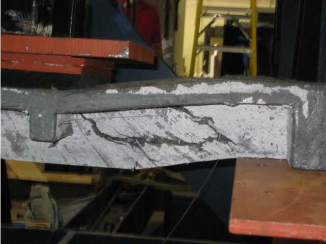
Figure 3.28 Pure Shear Failure of Specimen 1T1S with 180° Hook
