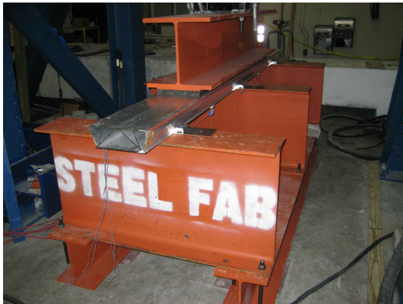
Figure 2.11 Test Setup for Two-Span Continuous Panel
