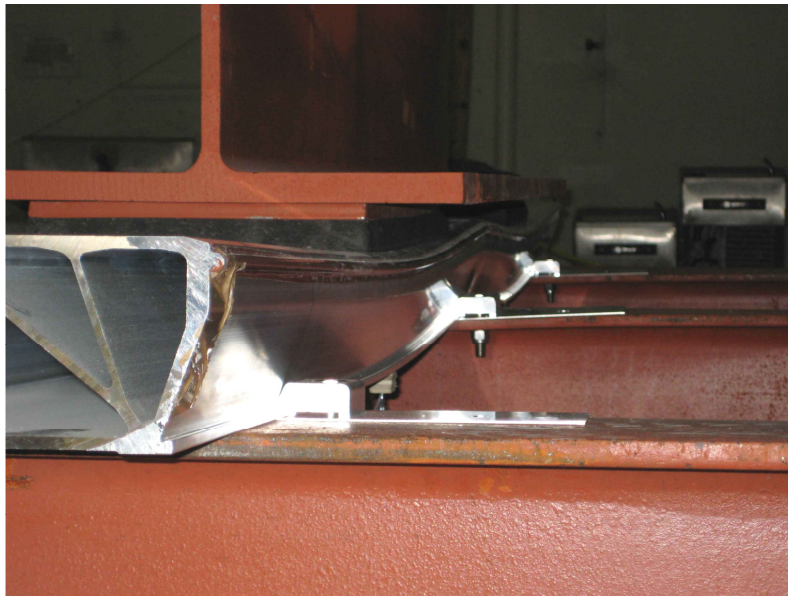
Figure 2.12 Deformed Shape of Two-Span Continuous Panel at Ultimate Load
