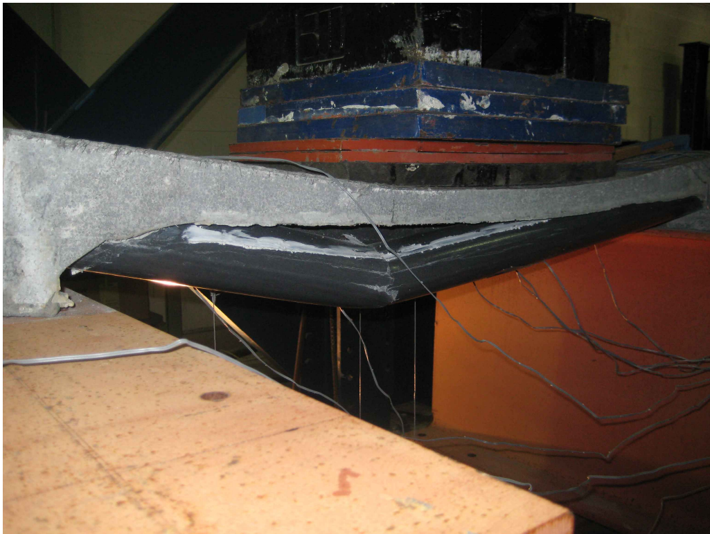
Figure 4.17 Failure Pattern of Tapered Section Ductal®-FRP Deck Specimen
