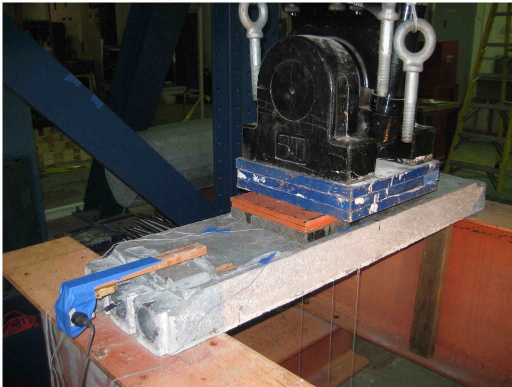
Figure 4.10 Test Setup for the Uniform Section Ductal®-FRP Deck Specimen
