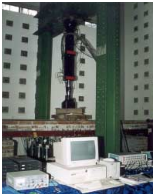
Fig. 5.13 Static Loading Setup of the Model Bridge.
