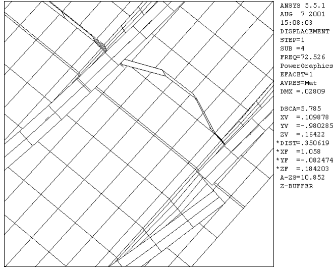
Fig. 4.28 the FE Model of Crack in the Girder (under Vibration).
