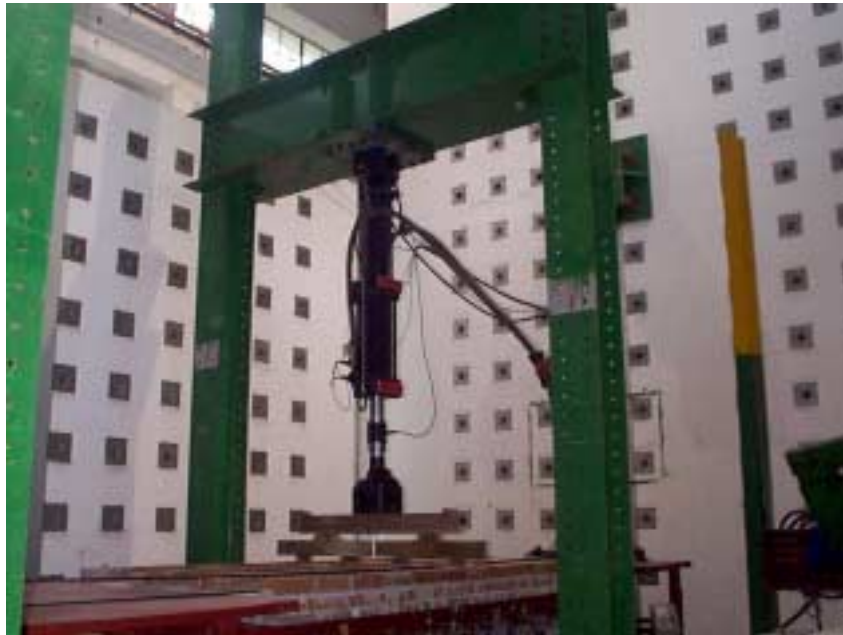
(c) Static Loading on the Model Bridge.
