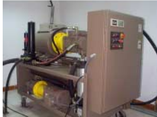
(b) Power Station of MTS.
