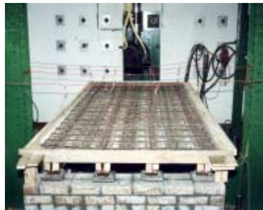
Fig. 4.12 Reinforcement of the Model.
