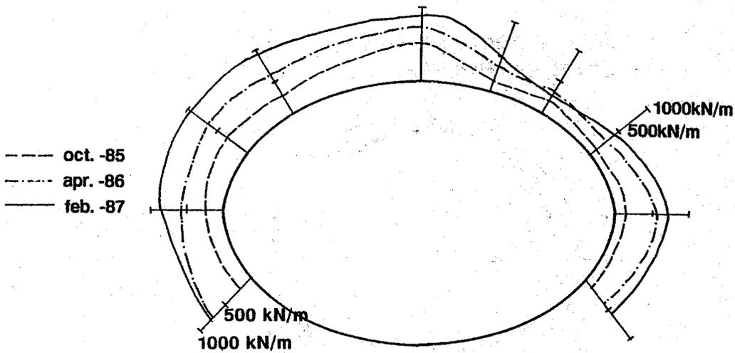
Fig. 1.8.4 Measured Thrust Force in the Steel Structure (Dovre)
