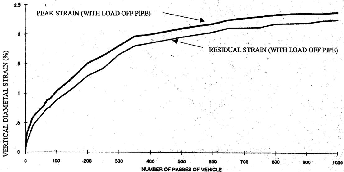
**Figure 1.6.6 Increase in Vertical Diametrical Strain for A Twin-Wall Pipe in A Trodden Sand Surround Under Repeated Loading in the Field Test**
