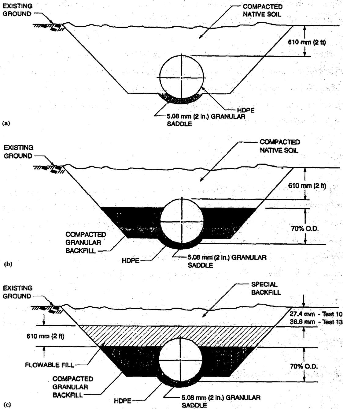
**Fig. 1.2.15 Cross Sections of Backfill Envelopes Used in Field Tests: (a) Tests 7 and 8; (b) Tests 9, 11, and 12; (c) Tests 10 and 13**
