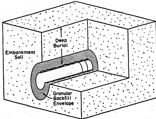
**Fig. 1.7.14a Exposed View Showing the Deeply Buried Pipe**
