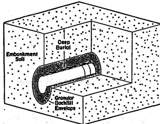
**Fig. 1.8.20 Typical Buried HDPE Pipe**
