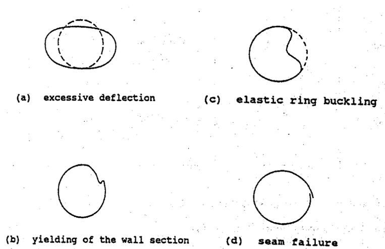
**Fig 1.1.2 Potential Failure Modes**
