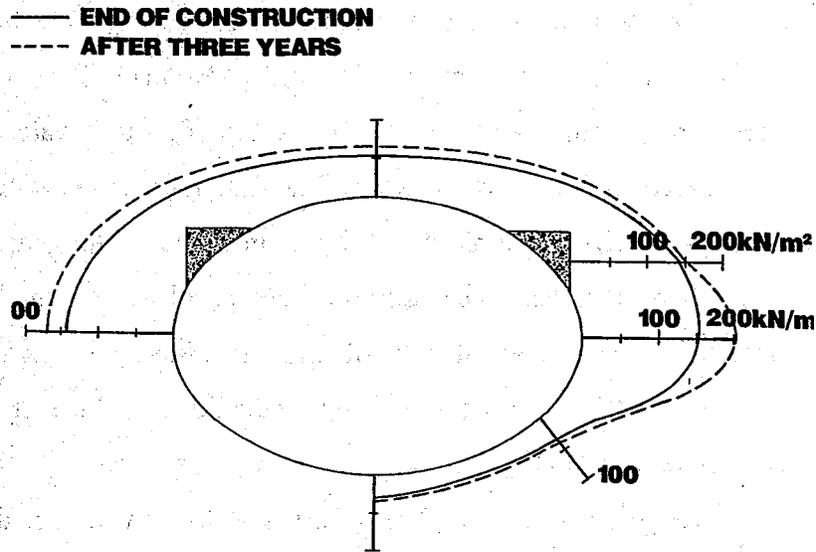
**Fig. 1.8.5 Measured Earth Pressure around the Structure (Dover)**
