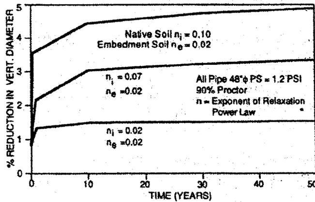
**Fig.1.8.14 Variation of Pipe Vertical Deflection over Time**
