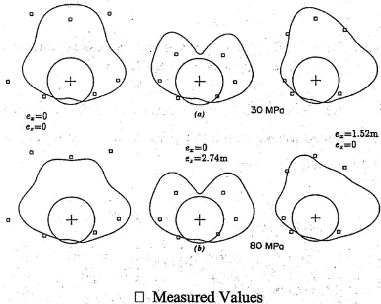
**Fig. 1.7.11 Thrust Distribution for Deux Rivieres Culvert (a)  $E' = 30 \text{ MPa}$  (b)  $E' = 80 \text{ MPa}$**
