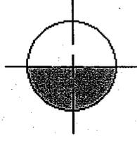
b) Flow at 50% of pipe diameter
