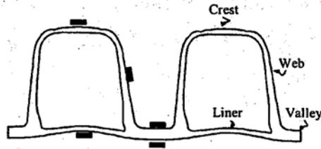
**Fig. 1.2.8 Pipe Profile and Location of Strain Gauges**
