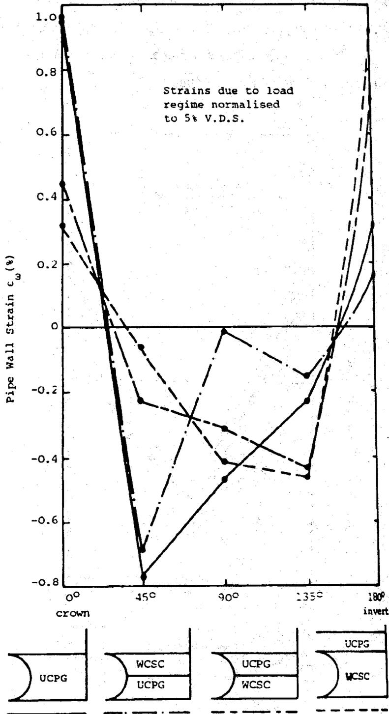
**Fig. 1.6.11 Pipe-Wall Strain Profiles Under 55 kN Static Load Using Four Combinations of Gravel and Clay**
