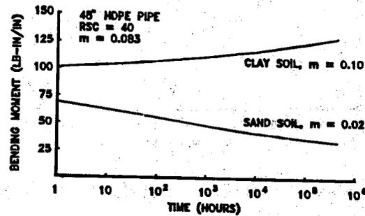
**Figure 1.8.19. Crown Bending Moment vs. Time for HDPE Pipe in Clay and in Sand**
