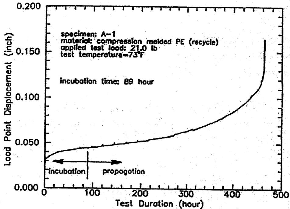
**Fig. 1.9.8 Raw SCG Test Data for Recycle Sample A-1. The Point of Inflection at 89 Hours Denotes Transition from Incubation to Crack Propagation**
