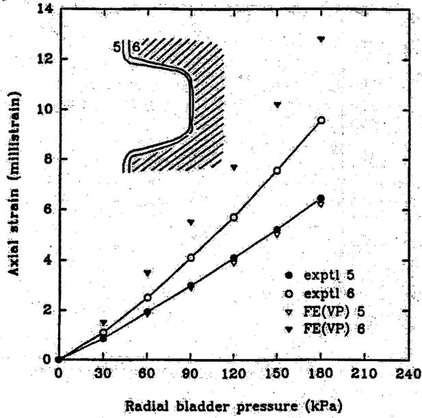
**Fig. 1.7.5 Axial Strain at Corrugation Valley: Finite Element Estimates and Experimental Measurements**
