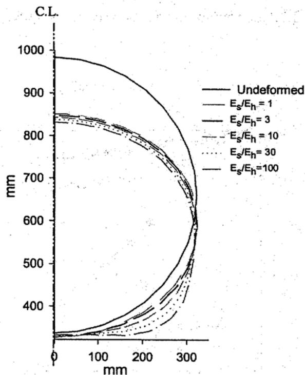
**Fig. 1.2.12 Deformed Shape of the Pipe for Different Soil Support (Deflection x 5)**
