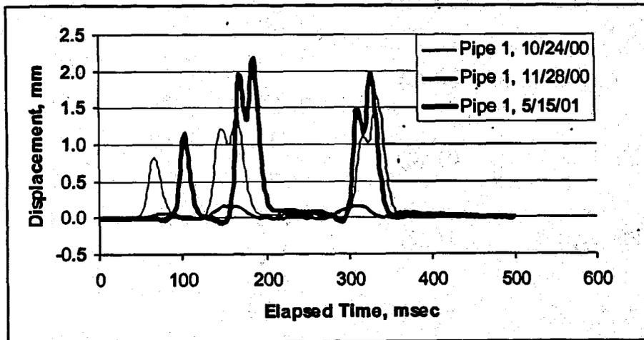
**Fig. 1.2.23 Typical Dynamic Response, 0.3 m (1 ft) Cover, 107 kN Axle Load Truck**
