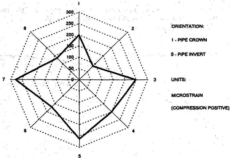
Strain distribution for a twin-wall pipe with uniform support from heavily compacted sand surround.
