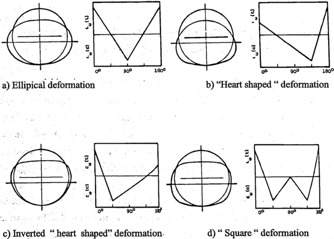
**Fig. 1.6.12 Types of Deformation and Associated Strain Profiles**
