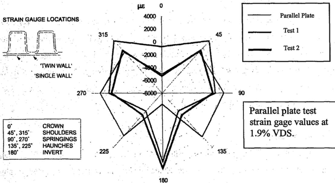
**Fig. 1.6.3 Twin Wall Strains Caused by the Complete Stress Sequence (End of Test Minus Installation) and Parallel Plate Testing**
