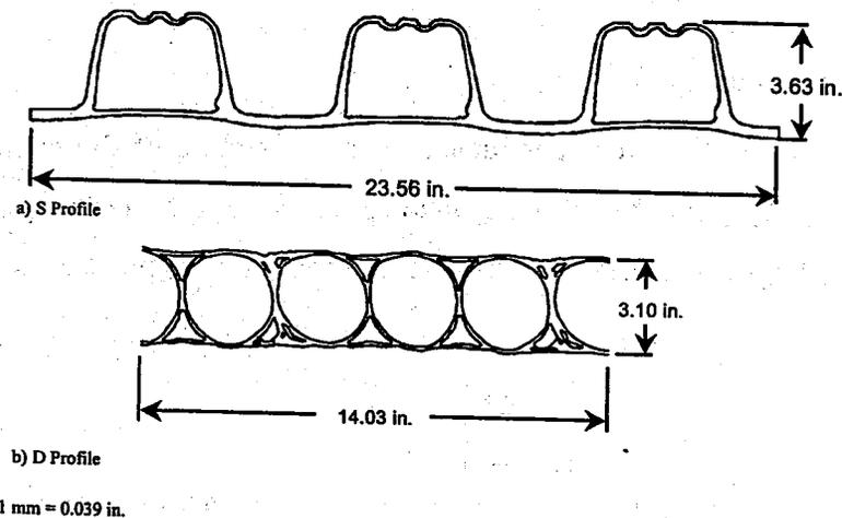
**Fig. 1.2.21 Actual Corrugated PE Wall Profiles**
