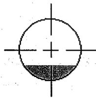
a) Flow at 25% of pipe diameter
