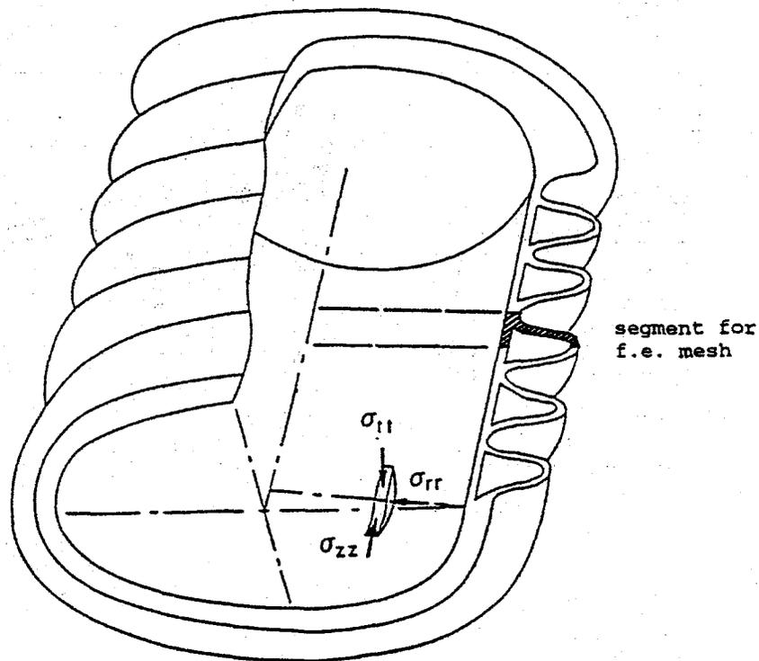
**Fig.1.7.14b Detail of the Pipe with Annular Corrugation and Smooth Internal Liner**
