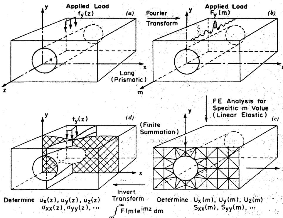
**Fig.1.7.8 Semianalytic Finite-Element Model for Shallow Buried Culvert**
