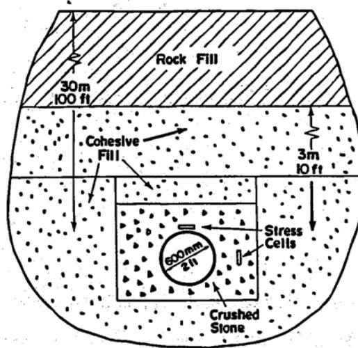
**Fig.1.8.25 Field Installation for Deeply Buried HDPE Pipe<sup>1</sup>**
