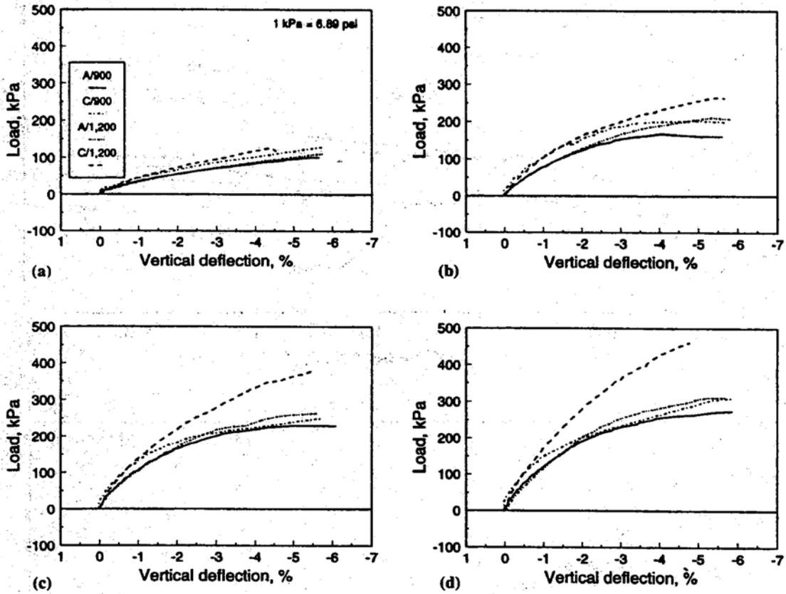
**Fig. 1.2.18 Vertical Deflection of Pipes with Varying Levels of Backfill: (a) No Backfill, (b) Backfill to Springline of Pipe, (c) Backfill to 70 Percent of Outside Diameter, (d) Backfill to Crown of Pipe**
