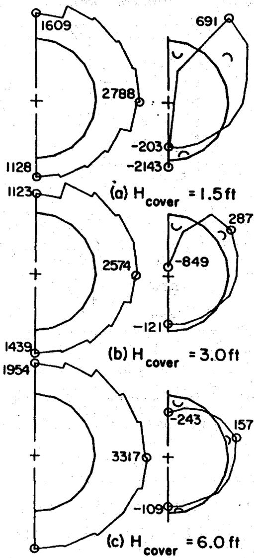
Fig. 1.2.14 Thrusts and Moments: 60-inch Pipe with HS-20 Surface Load
