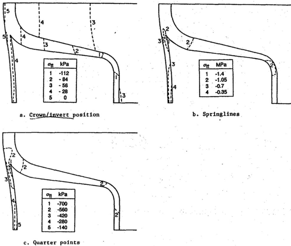
Fig.1.7.16 Circumferential Pipe Stresses at Crown/Invert, Springlines and Quarter Points
