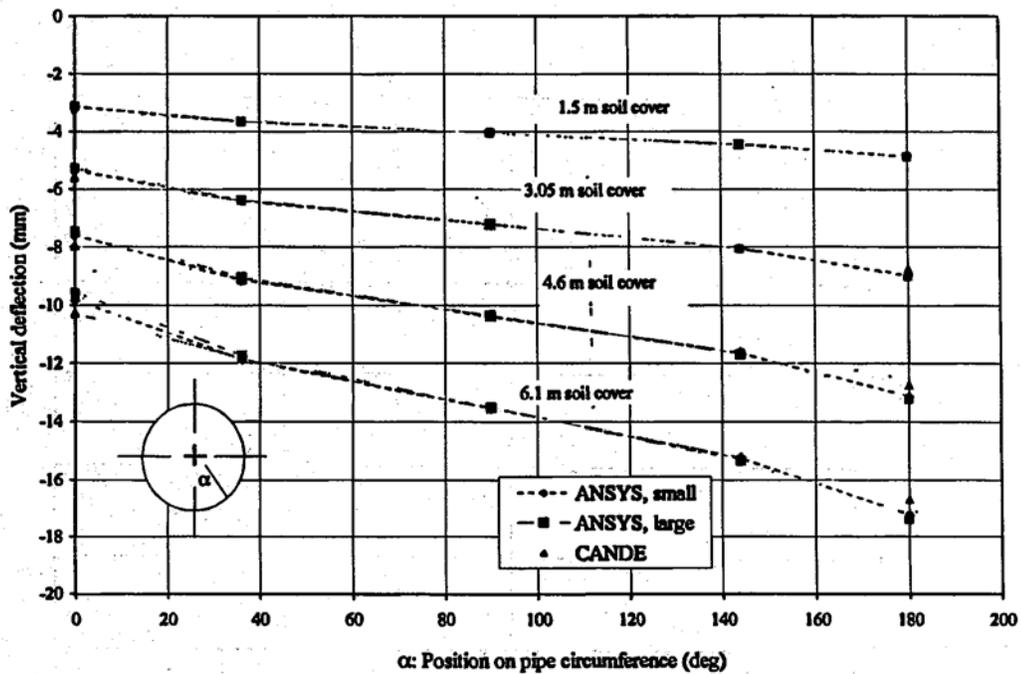
**Fig. 1.7.19 PE Pipe Crown Vertical Deflection with Respect to Position on Pipe Circumference for Different Height of Soil Covers (1 foot = 0.305m, 1 inch = 25.4mm)**
