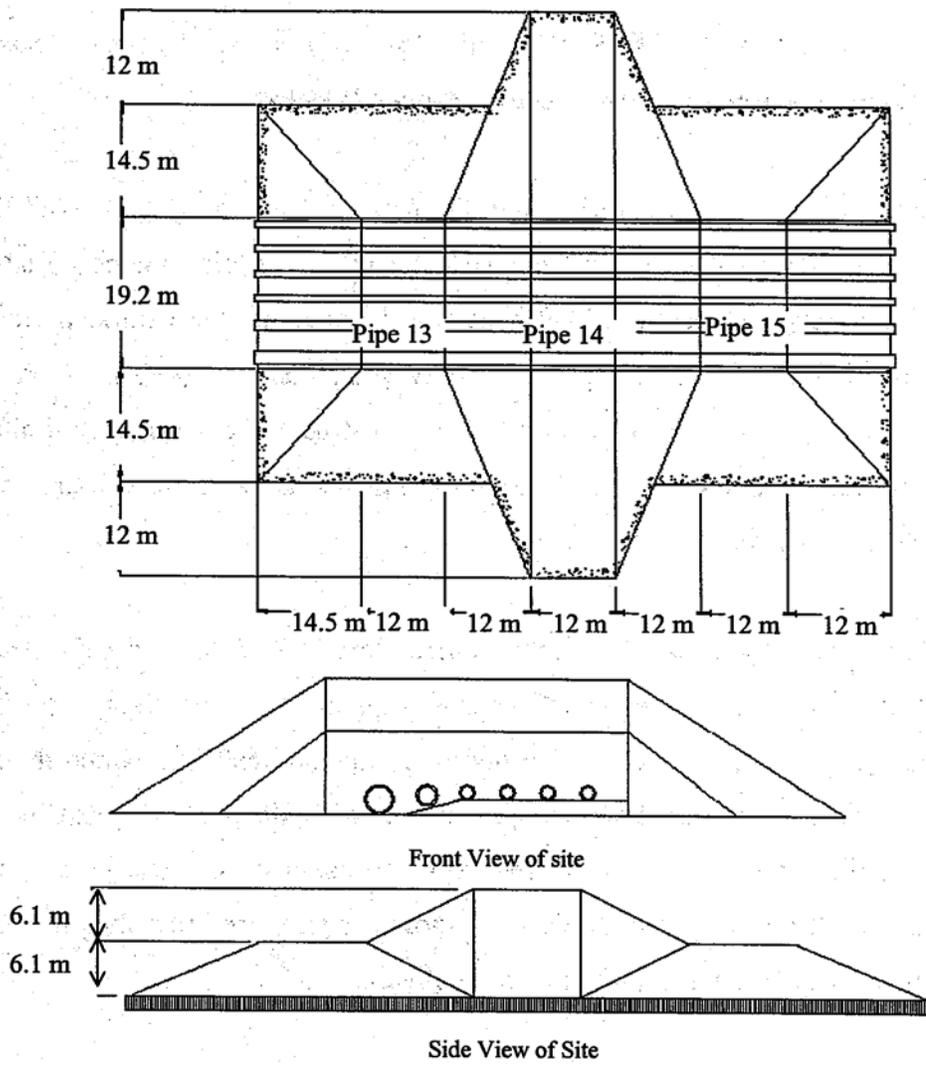
**Fig. 1.2.3 Overall Layout of Thermoplastic Pipes at Deep Burial Test Site**
