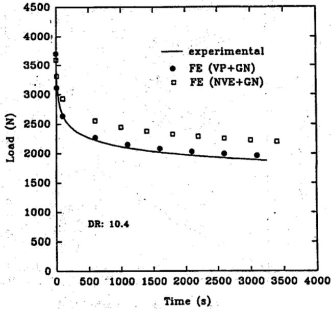
**Fig. 1.7.3 Load Relaxation with Time for Plain at Fixed Vertical Deflection after Abrupt Change Deflection Rate: Measurements and Nonlinear Finite Element Predictions**
