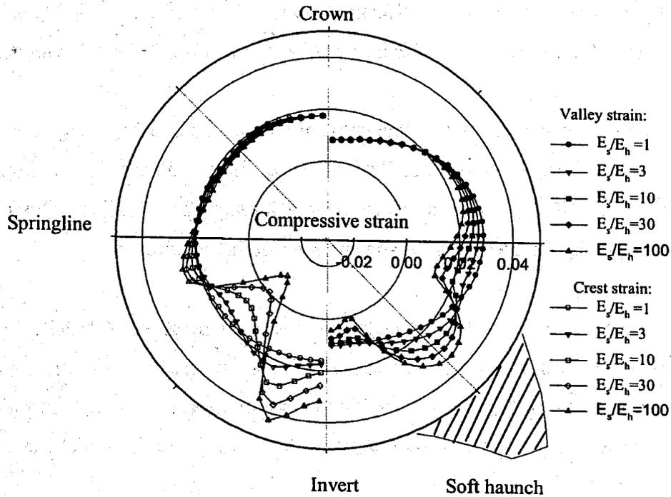
**Fig. 1.2.13 Distribution of Circumferential Strains on HDPE Pipe**
