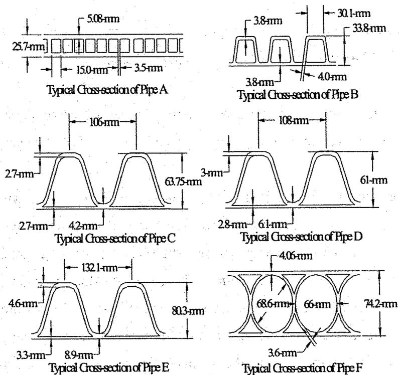
**Fig.1.8.1 Cross-Sections of The Test**
