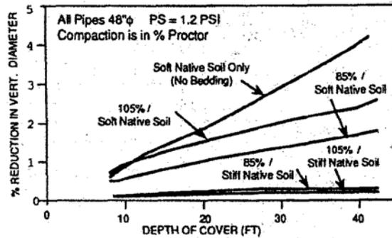
**Fig. 1.8.8 Vertical Deflection of Pipes in Different Soils**
