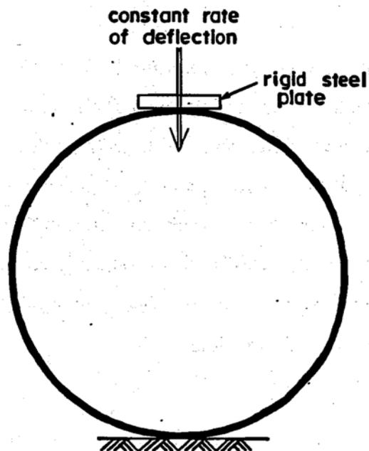
**Fig. 1.8.23a. Loading Conditions for the Parallel Plate Test**
