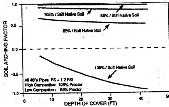
**Fig.1.8.10 Arching Factor of A Soil-Pipe System in Different Soils**
