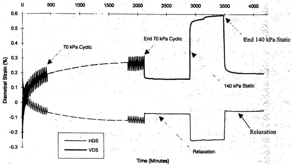
**Fig. 1.6.2 Diametral Strains due to Installation and 70-Kpa Cyclic and 140-Kpa Static Stress Phases**
