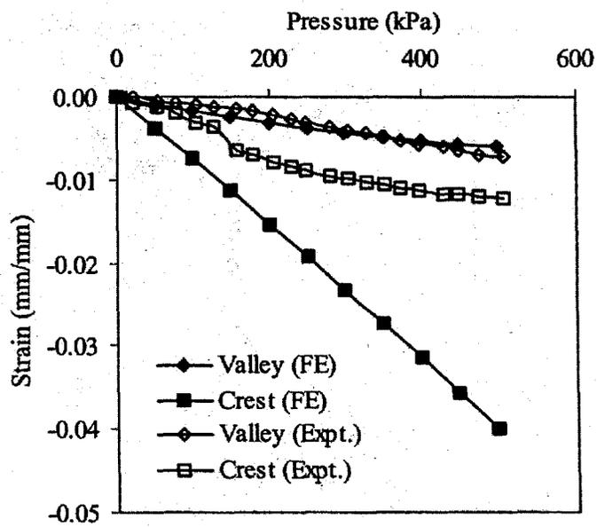
Fig. 1.2.11 Circumferential Strain at the Crown
