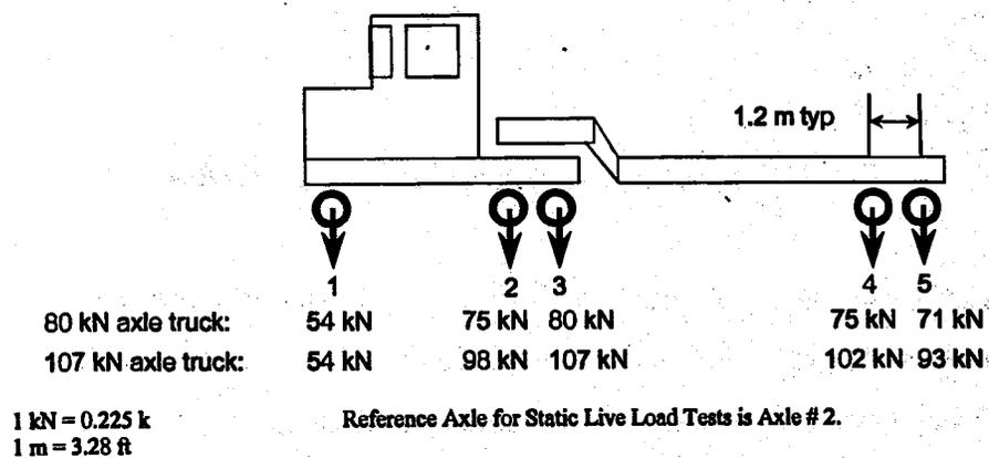
**Fig. 1.2.22 Truck Configuration and Axle Loads**
