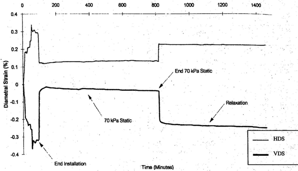
**Fig.1.6.1 Diametral Strains due to Installation and 70-Kpa Static Stress Phases**
