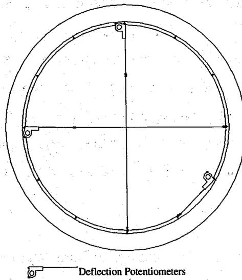
**Fig. 1.2.2 Orientation of Potentiometers**
