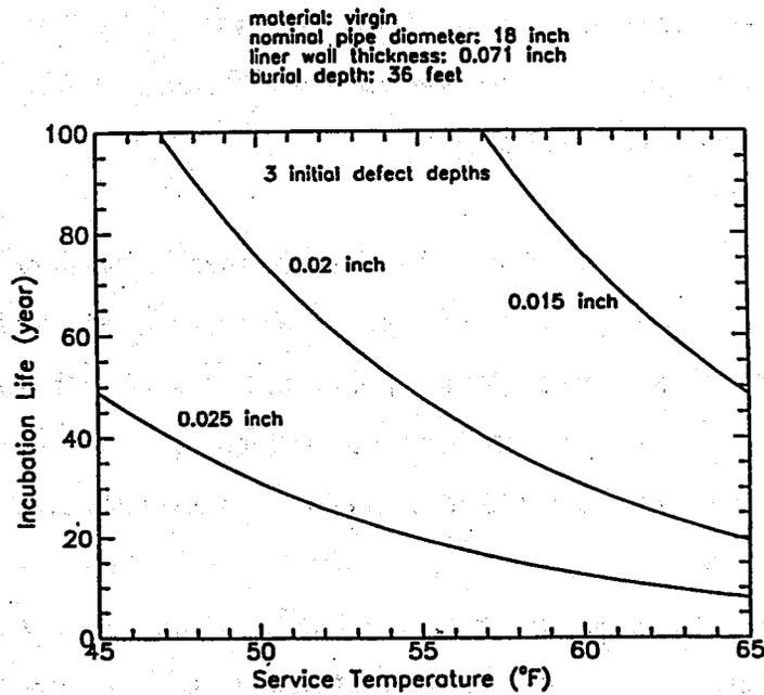
**Fig. 1.9.10 Estimated Lifetime of 18 Inch Diameter Virgin Pipe Buried at A Depth of 36 Feet versus Service Temperature for Three Defect Depths**
