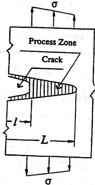
**Figure 1.9.1 Schematic Presentation of Crack Layer in PEs**
