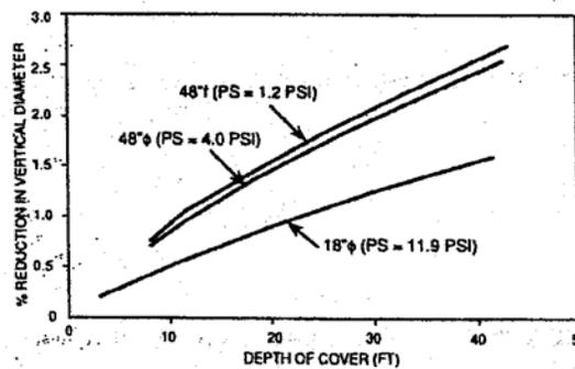
**Fig. 1.8.7 Vertical Deflections for Pipes of Different Stiffness**
