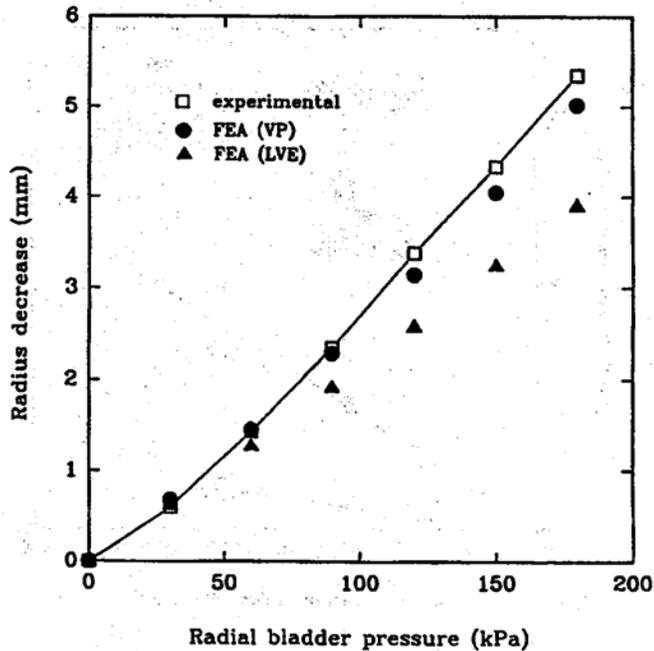
**Fig. 1.7.4 Radius Decrease Versus Air Bladder Pressure: Test Measurements and Finite Element Predictions**
