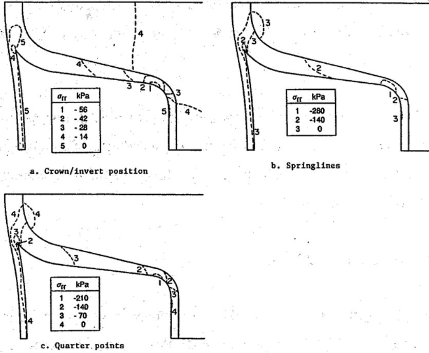
**Fig.1.7.17 Radial Pipe Stresses at Crown/Invert, Springlines and Quarter Points**
