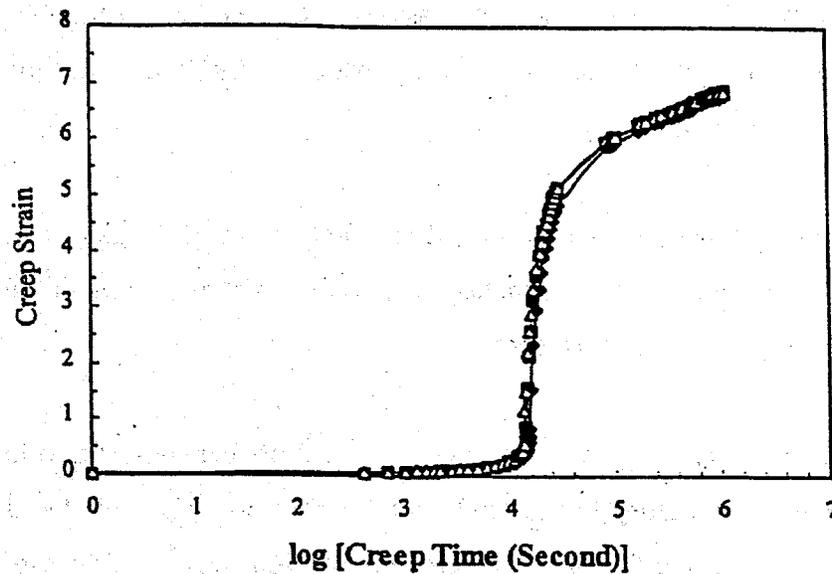
**Figure 1.9.6 Creep Behavior of a HDPE Material Under the Stress of Drawing Stress**
