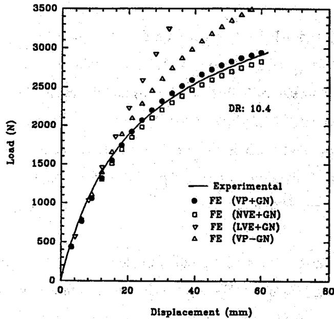
**Fig. 1.7.1 Load Deflection Response for Plain Pipe at 12-Mm/Min Vertical Deflection Rate Until 20 Percent Decrease in Vertical Diameter: Measurements and Finite Element Predictions**
