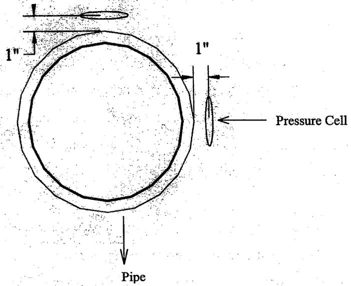
**Fig. 1.2.1 Pressure Cell Configuration**
