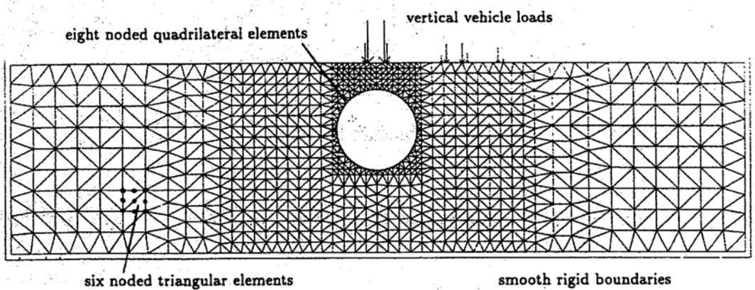
**Fig.1.7.10 Finite Element Mesh to Model Deux Rivieres Culvert**
