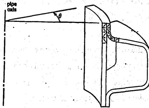
**Fig.1.8.21 Finite Element Model for Axisymmetric Pipe Analysis**
