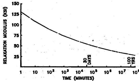
**Figure 1.8.18 Stress Relaxation Modulus vs. Time for HDPE**
