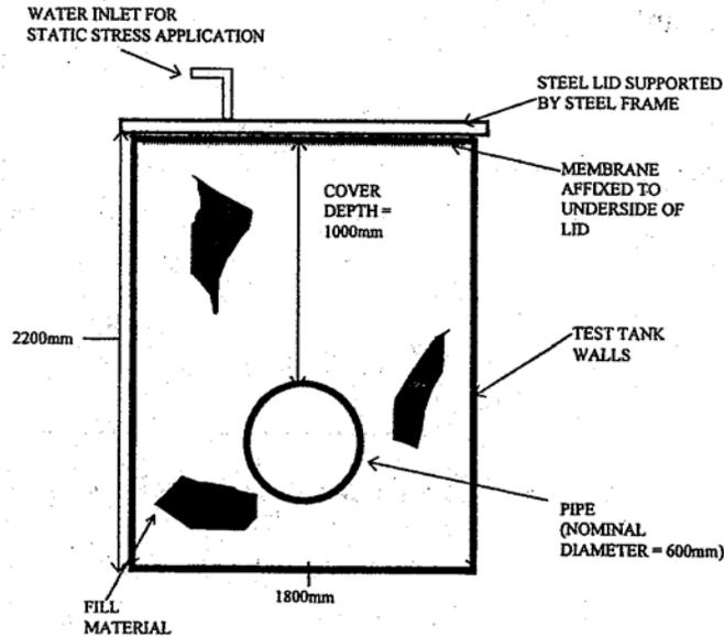
**Fig. 1.3.1 Cross Section Through Test Apparatus**
