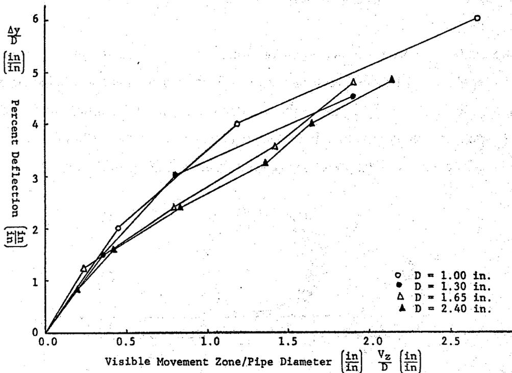
**Fig. 1.4.3 Visible Movement Zone/Pipe Diameter  $V_z/D$  for Small Diameter Pipes
