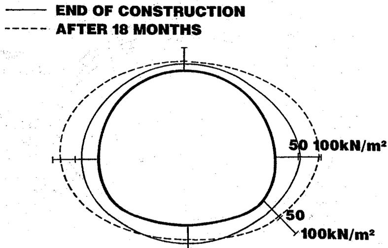
**Fig. 1.8.2 Measured Earth Pressure Around the Structure (Tolpinrud)**
