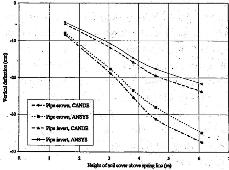
**Fig. 1.7.20 PE Vertical Deflection using Duncan Chang Model for both ANSYS and CANDE (1 foot = 0.305m, 1 inch =25.4 mm)**
