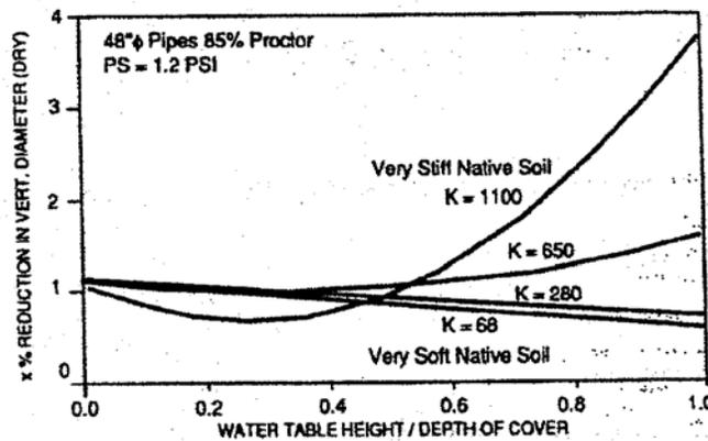
**Fig. 1.8.11 Effects of Groundwater on Pipe Deflection**
