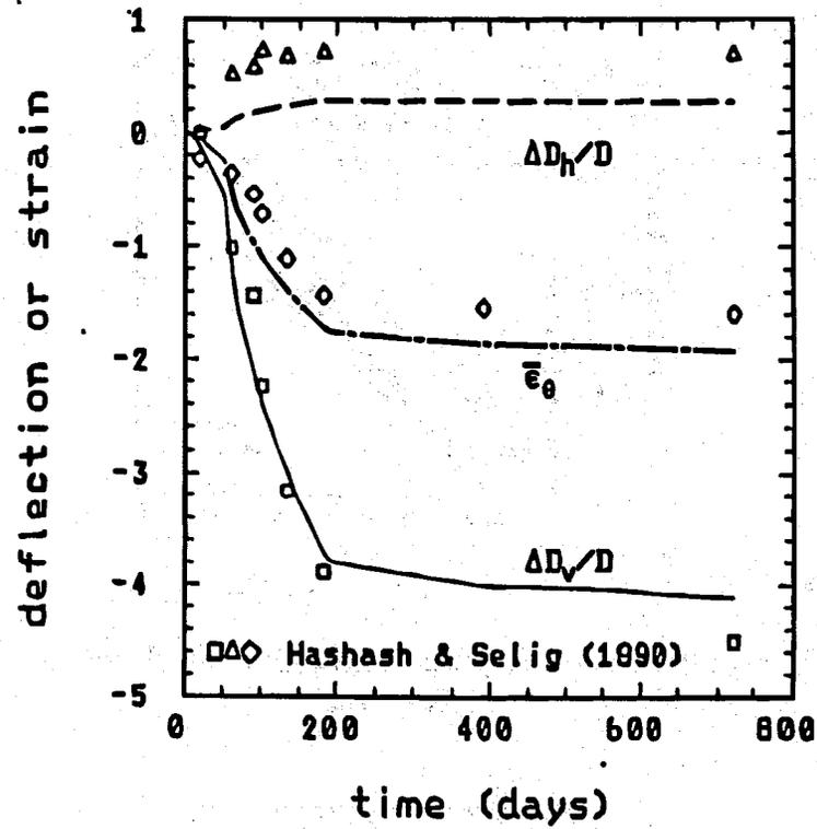
**Fig. 1.8.26 Measurement and Theoretical Prediction of Pipe Deformation and Circumferential Strain**
