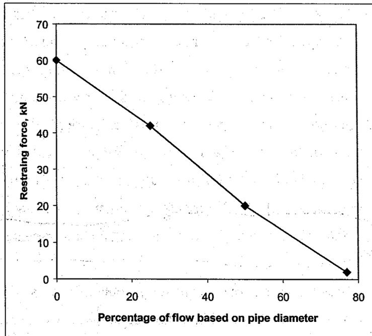
**Fig. 1.1.5b Influence of Flow Condition on Restraining Force**
