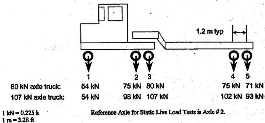
**Fig. 1.2.22 Truck Configuration and Axle Loads**
