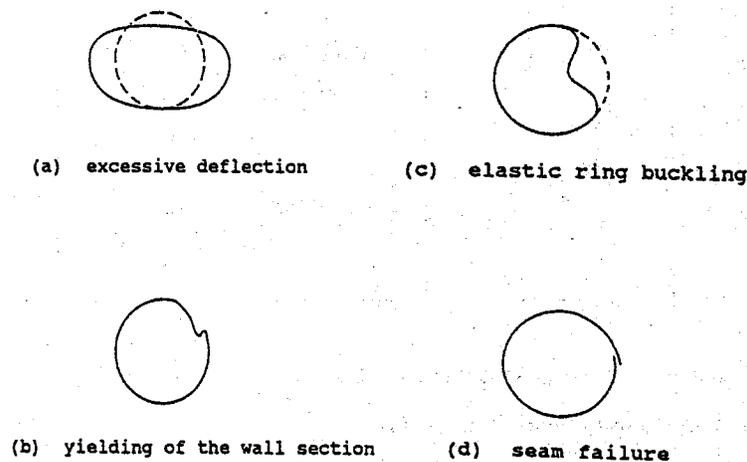
**Fig 1.1.2 Potential Failure Modes**
