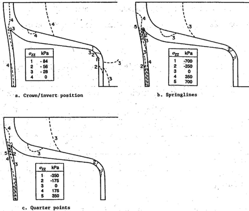
**Fig.1.7.18 Axial Pipe Stresses at Crown/Invert, Springlines and Quarter Points**
