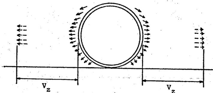
**Fig.1.4.2 Peripheral Soil Movement and  $V_z$  for Small Diameter Pipes**
