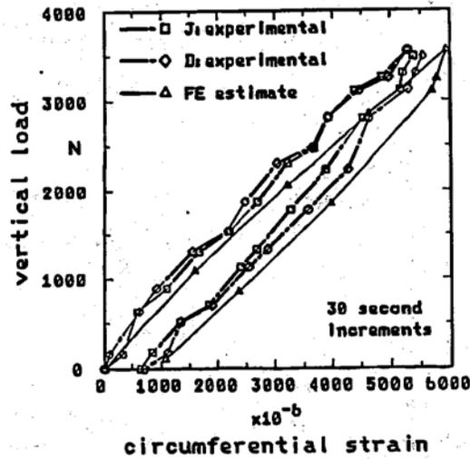
**Fig.1.8.24 Experimental Measurement and Finite Element Predictions for the Parallel Plate Test**
