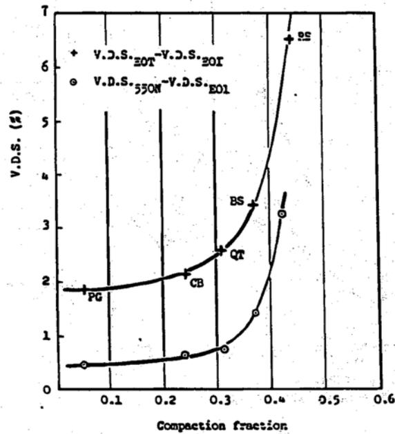
**Fig. 1.6.9 Influence of Empirical Soil Factor, Compaction Fraction**
