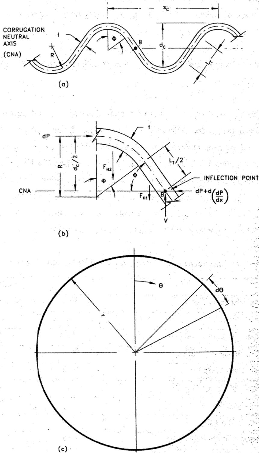
**Fig. 1.5.1 Description Of CMP: (a) Corrugation Detail; (b) Free Body Diagram of One-Quarter Corrugation Cycle; (c) Transverse Cross Section**
