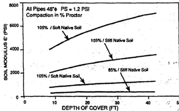
**Fig.1.8.9 Soil Moduli for Different Depths of Cover**
