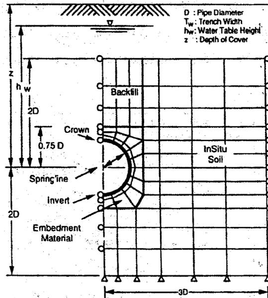
**Fig.1.8.6 Typical Configuration of A Pipe Trench**
