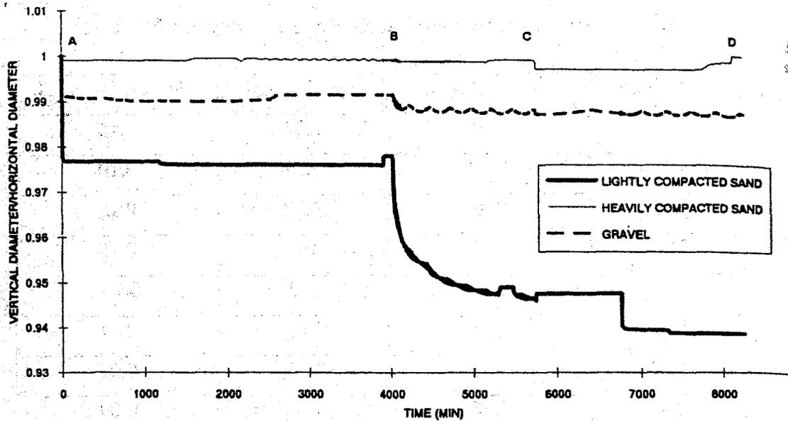
Relative variation of vertical diameter to horizontal diameter for twin-wall pipe during laboratory test.
