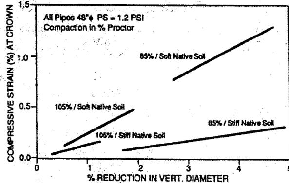
**Fig.1.8.13 Pipe Strains at Crown for Different In Situ Soils**
