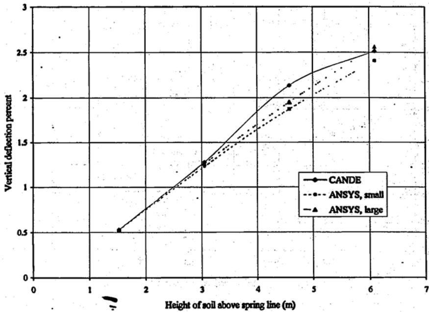
**Fig. 1.7.21 PE Vertical Deflection Percent using Duncan Chang Model for both ANSYS and CANDE (1 foot = 0.305m)**
