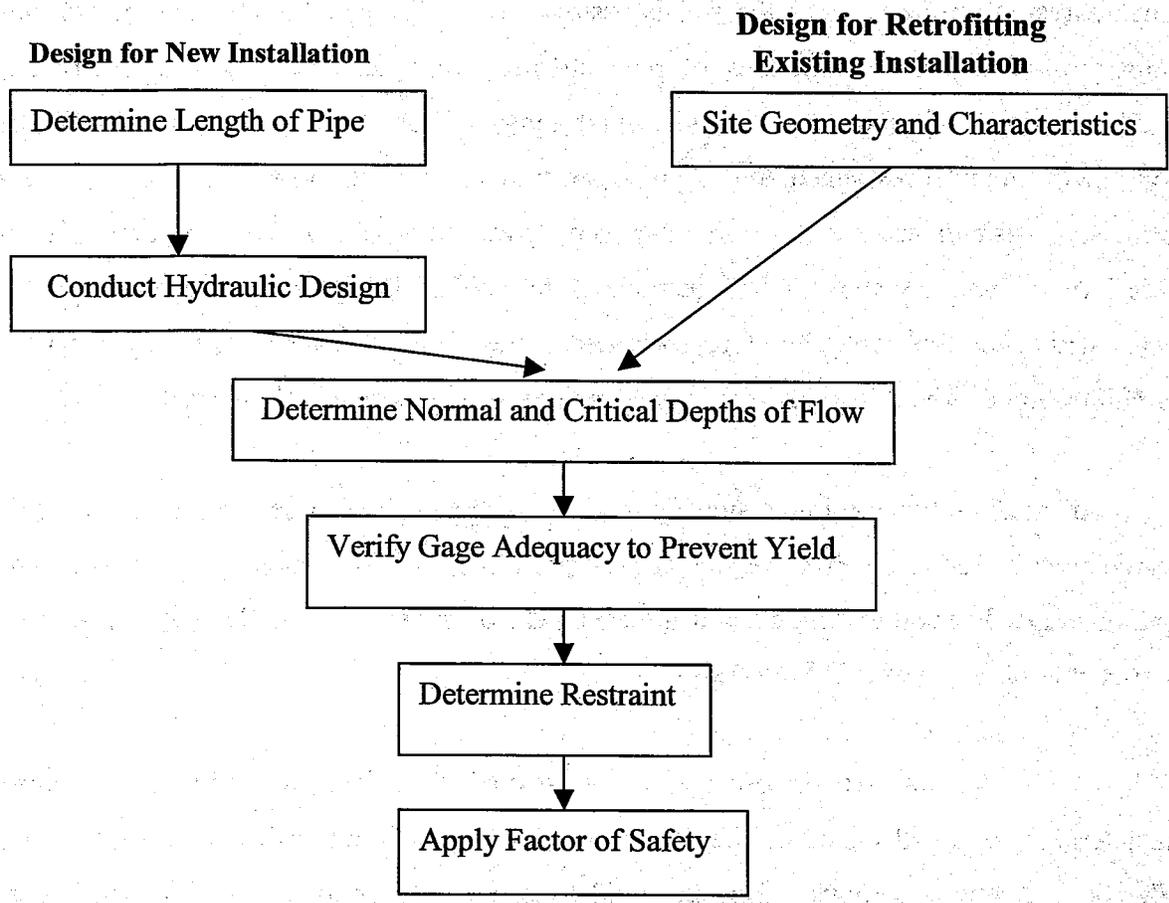
**Fig. 1.1.3 Flowchart for Design Process to Determine Restraining Force**
