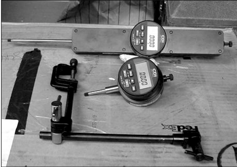
Figure 4.2 Chicago Dial Indicators (Logic Basic Model) and Support Clamp
