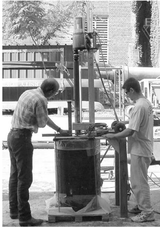
Figure 5.1 C. Kohlhof and C. Cepero Using Hilti Rig to Core Gatorock Sample
