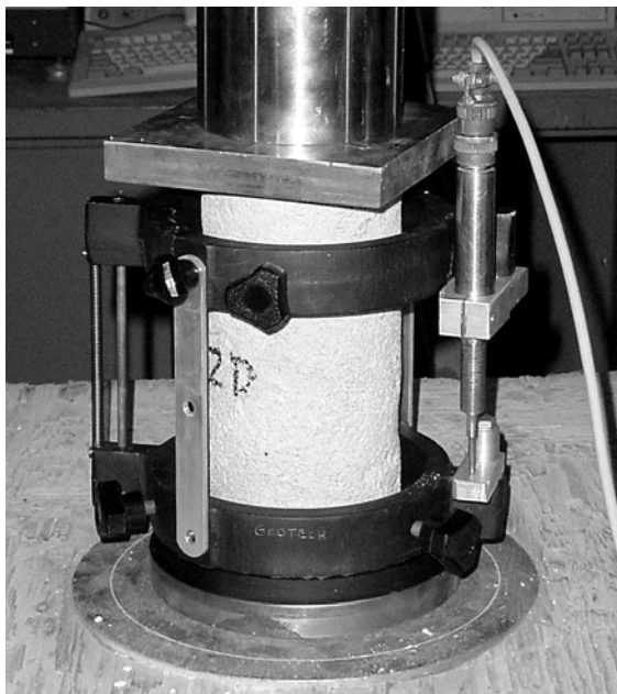
Figure 3.2 Gatorock Sample with Compressometer and LVDT for Deformation
