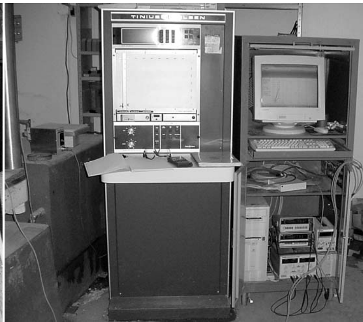
Figure 3.3 Automated Tinius Olsen Load Frame used for Tests of Gatorock Cores
