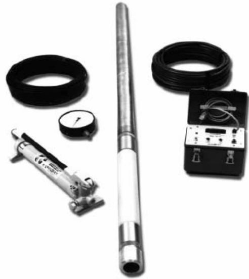
Figure 2.6 Probex-1 Rock Dilatometer (Roctest, Inc.)
