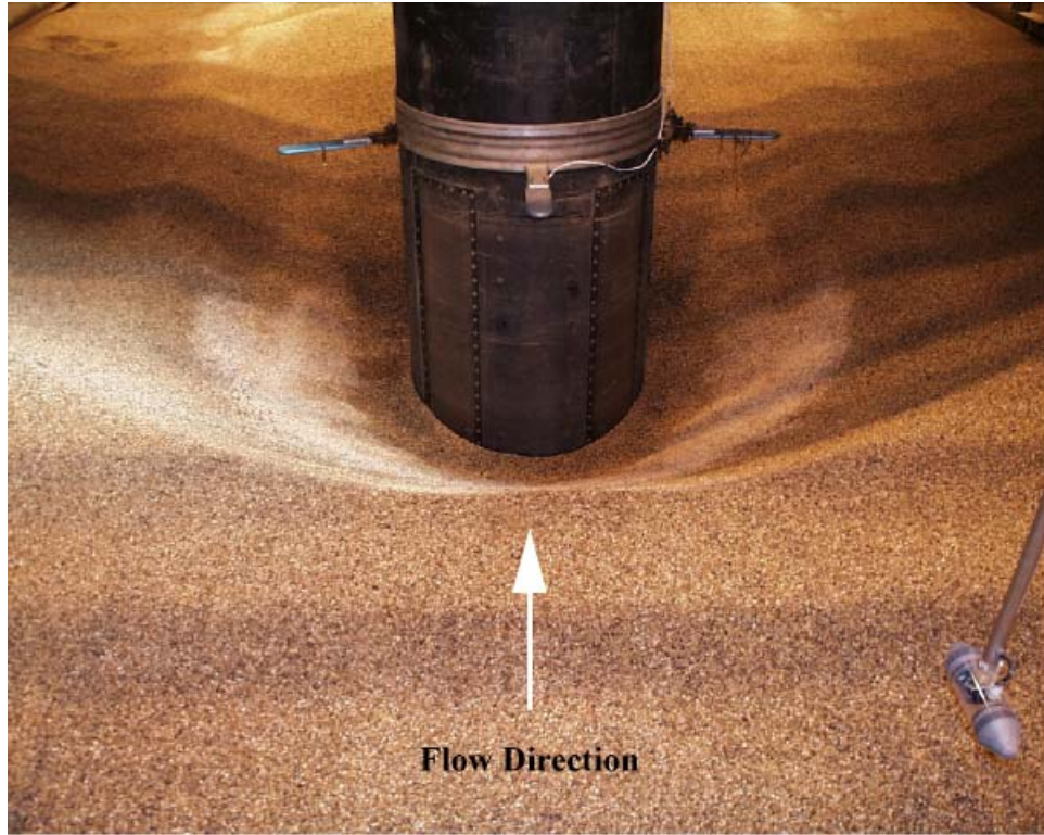
Figure C- 96. Experiment 9 ( D = 0.915 m, D_{50} = 2.90 mm) after test.
