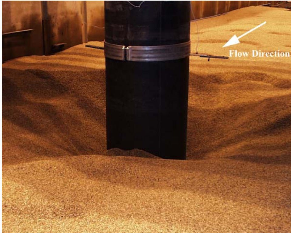
Figure C- 87. Experiment 8 ( D = 0.915 m, D_{50} = 2.90 mm) after test.
