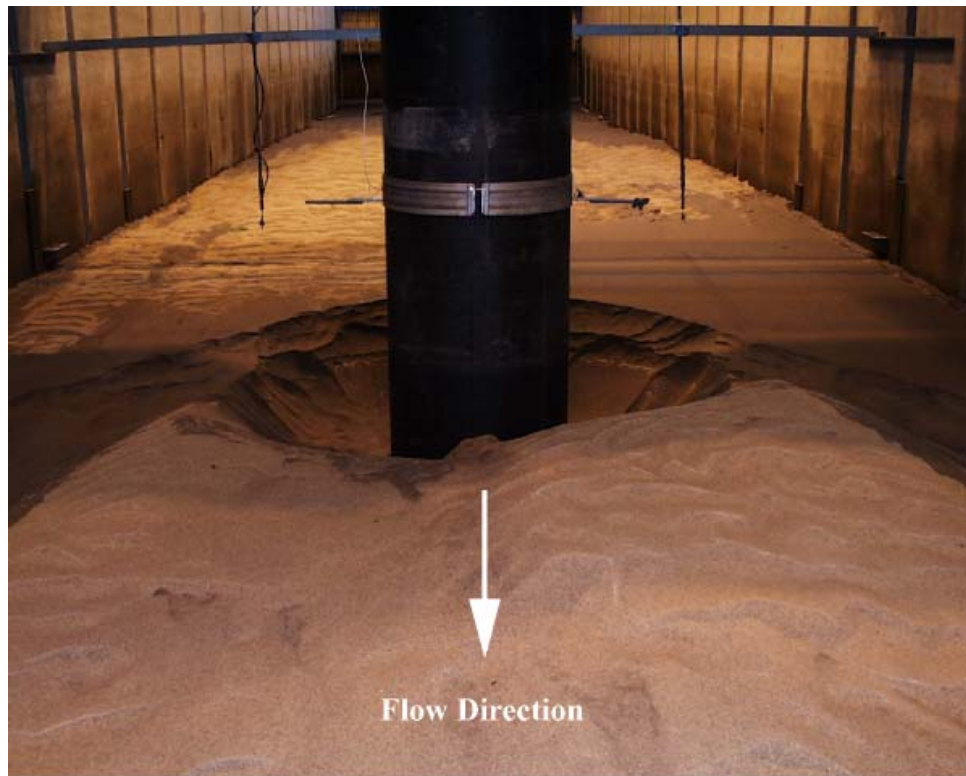
Figure C- 39. Experiment 4 ( D = 0.915 m, D_{50} = 0.80 mm) after test.
