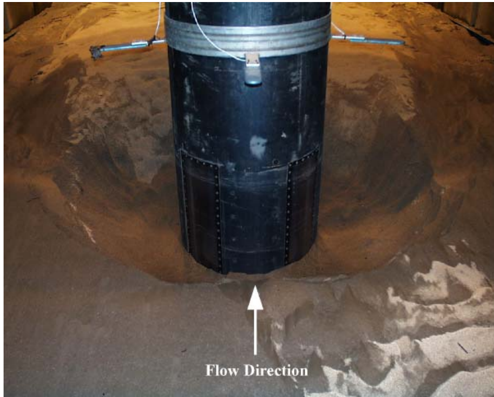
Figure C- 36. Experiment 4 ( D = 0.915 m, D_{50} = 0.80 mm) after test.
