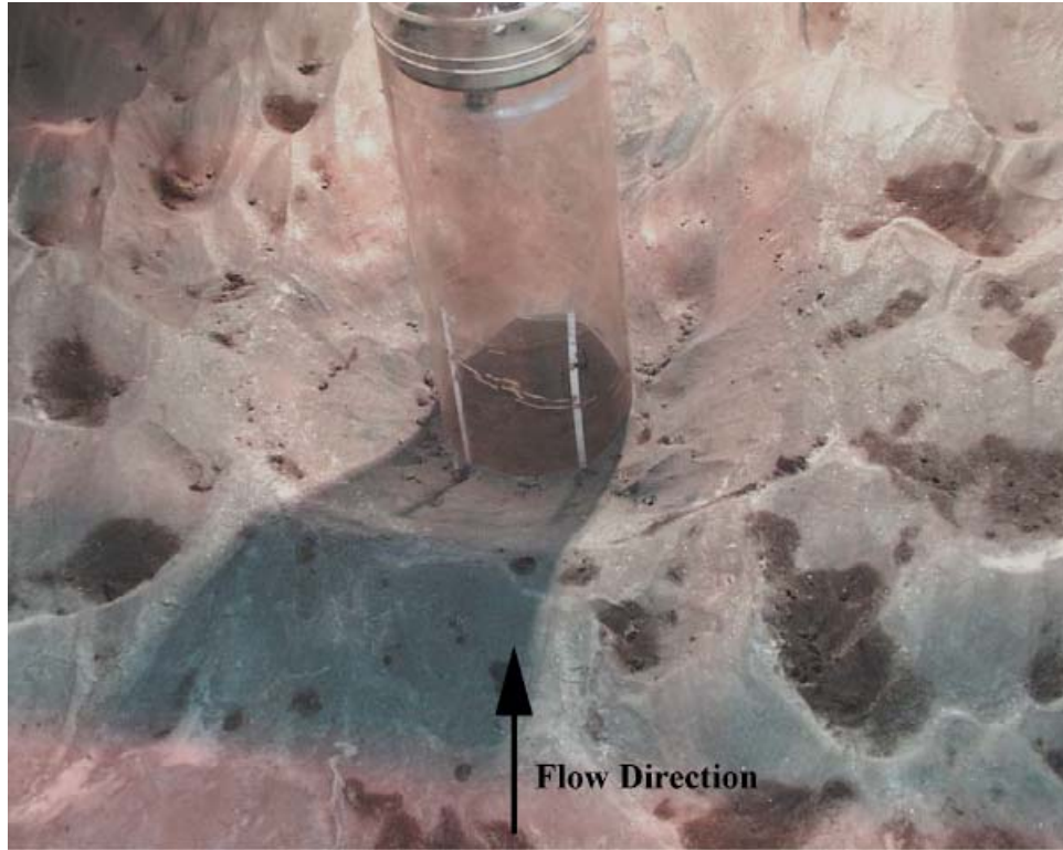
Figure C- 14. Experiment 2 ( D = 0.305 m, D_{50} = 0.22 mm) after test.
