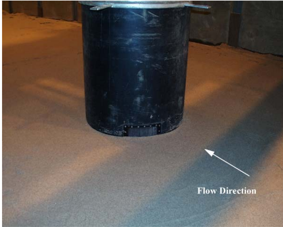
Figure C- 24. Experiment 3 ( D = 0.915 m, D_{50} = 0.80 mm) before test.
