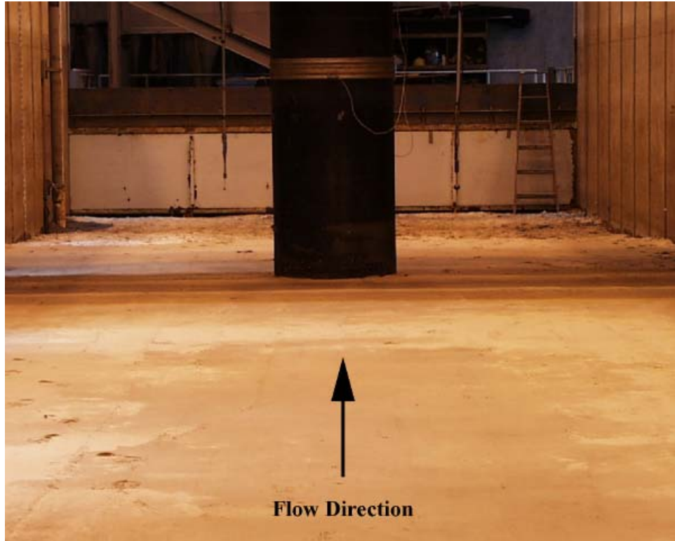
Figure C- 156. Experiment 14 ( D = 0.915 m, D_{50} = 0.22 mm) before test.
