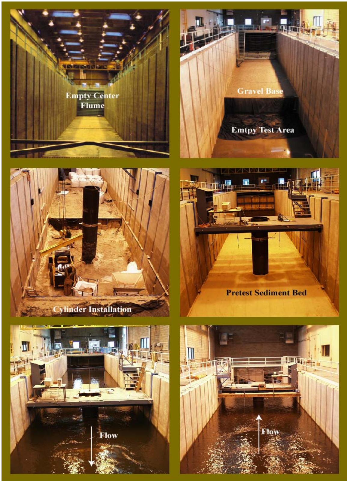
Figure A-4. Photographs of the test flume at various stages of setup and use.
