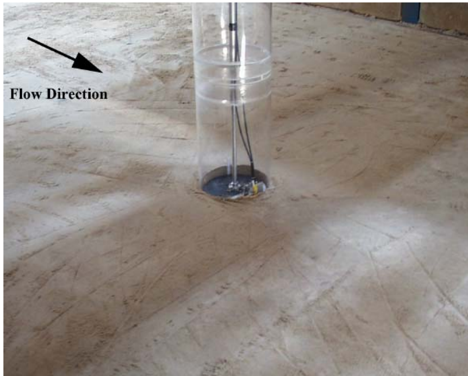
Figure C- 12. Experiment 2 ( D = 0.305 m, D_{50} = 0.22 mm) before test.
