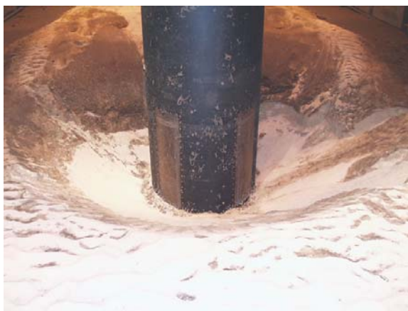
Figure E- 4. Scour hole after low suspended fine sediment experiment (Experiment B) ( D = 0.915 m, D_{50} = 0.22 mm, y_o = 1.8 m, V/V_c = 0.97 ).
