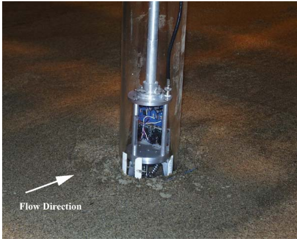
Figure C- 6. Experiment 1 ( D = 0.114 m, D_{50} = 0.22 mm) before test.
