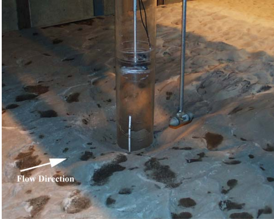
Figure C- 16. Experiment 2 ( D = 0.305 m, D_{50} = 0.22 mm) after test.
