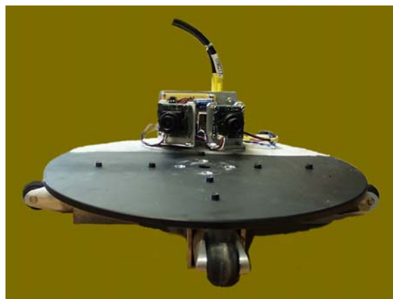
Figure B- 5. The internal cameras for the 0.305 m (1 ft) diameter cylinder.
