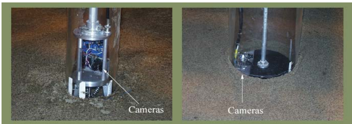
Figure B- 7. Photographs of the forward-looking internal cameras positioned inside the 0.114 m (4.5 in) and 0.305 m (1 ft) diameter watertight cylinders.
