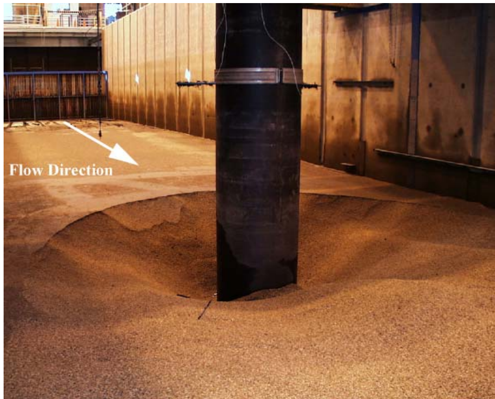
Figure C- 121. Experiment 11 ( D = 0.915 m, D_{50} = 2.90 mm) after test.
