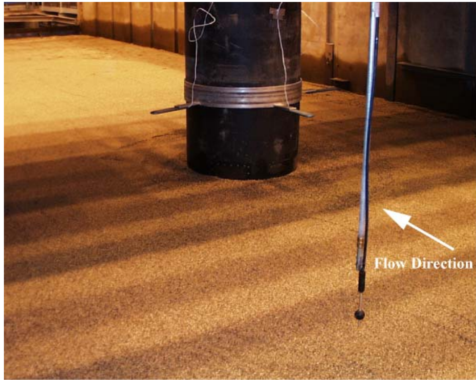
Figure C- 83. Experiment 8 ( D = 0.915 m, D_{50} = 2.90 mm) before test.
