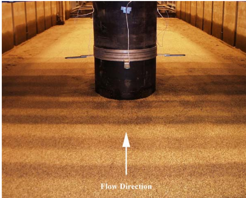
Figure C- 92. Experiment 9 ( D = 0.915 m, D_{50} = 2.90 mm) before test.
