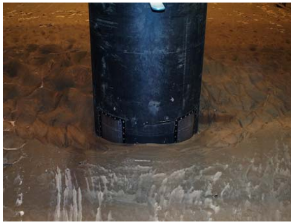
Figure E- 3. Scour hole after high suspended fine sediment experiment (Experiment A) ( D = 0.915 m, D_{50} = 0.22 mm, y_o = 1.22 m, V/V_c = 0.92 ).
