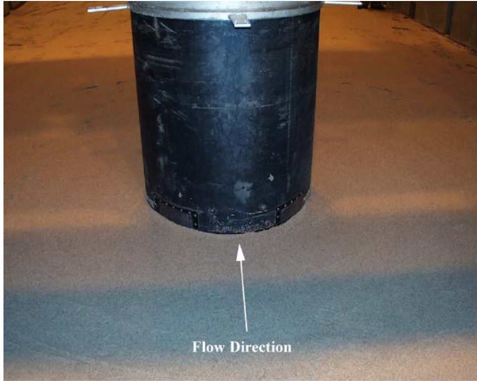
Figure C- 22. Experiment 3 ( D = 0.915 m, D_{50} = 0.80 mm) before test.
