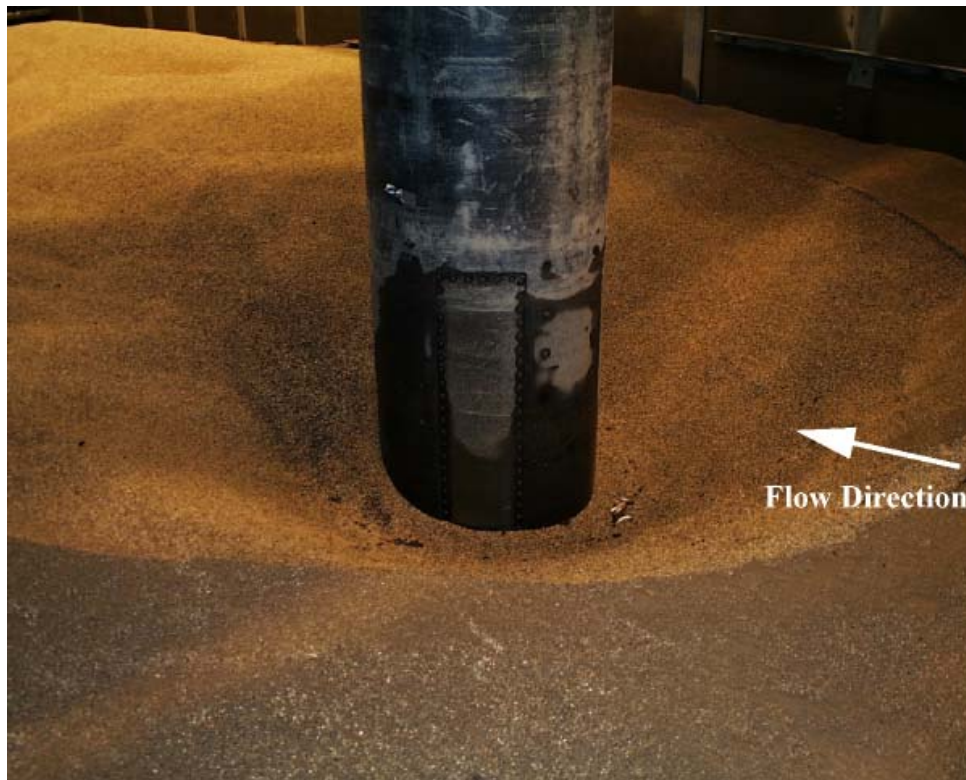
Figure C- 117. Experiment 11 ( D = 0.915 m, D_{50} = 2.90 mm) after test.
