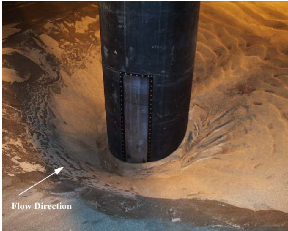
Figure C- 26. Experiment 3 ( D = 0.915 m, D_{50} = 0.80 mm) after test.
