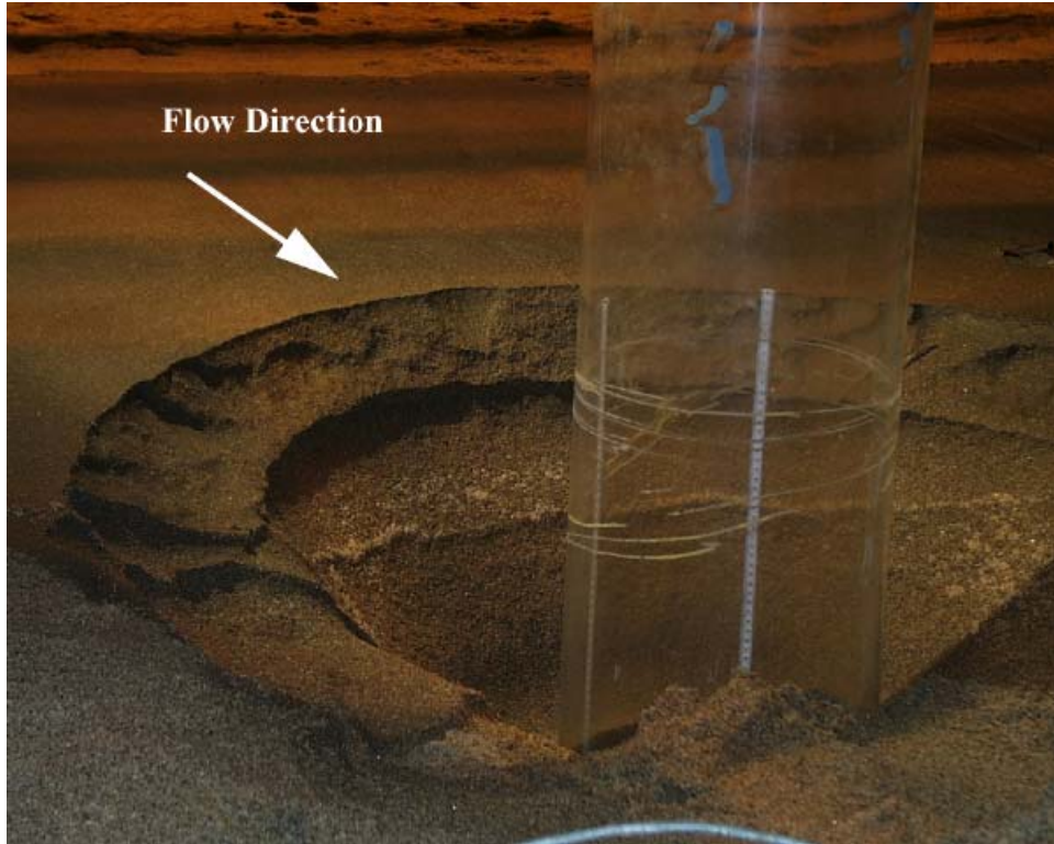
Figure C- 52. Experiment 5 ( D = 0.305 m, D_{50} = 0.80 mm) after test.
