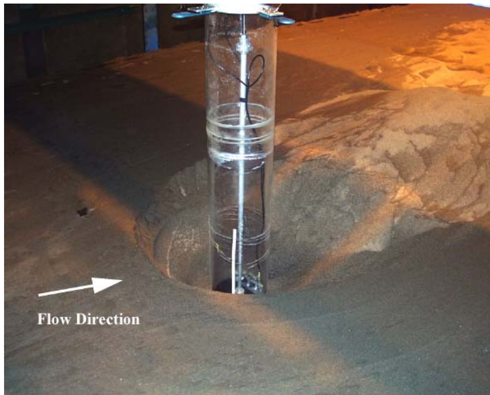
Figure C- 49. Experiment 5 ( D = 0.305 m, D_{50} = 0.80 mm) after test.
