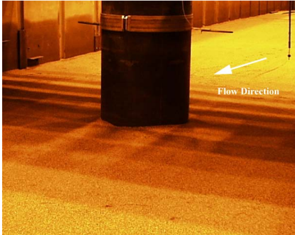
Figure C- 70. Experiment 7 ( D = 0.915 m, D_{50} = 2.90 mm) before test.
