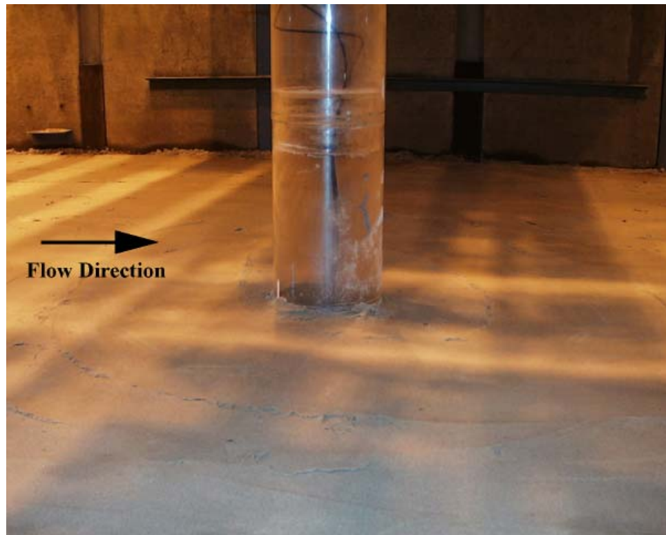
Figure C- 142. Experiment 13 ( D = 0.305 m, D_{50} = 0.22 mm) before the test.
