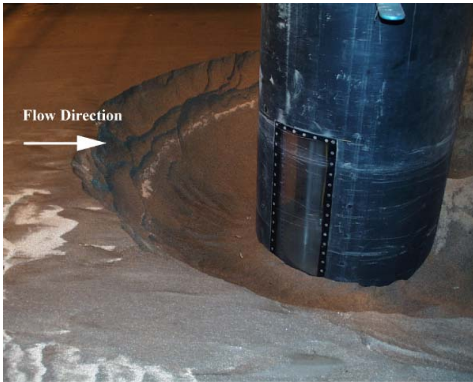
Figure C- 41. Experiment 4 ( D = 0.915 m, D_{50} = 0.80 mm) after test.
