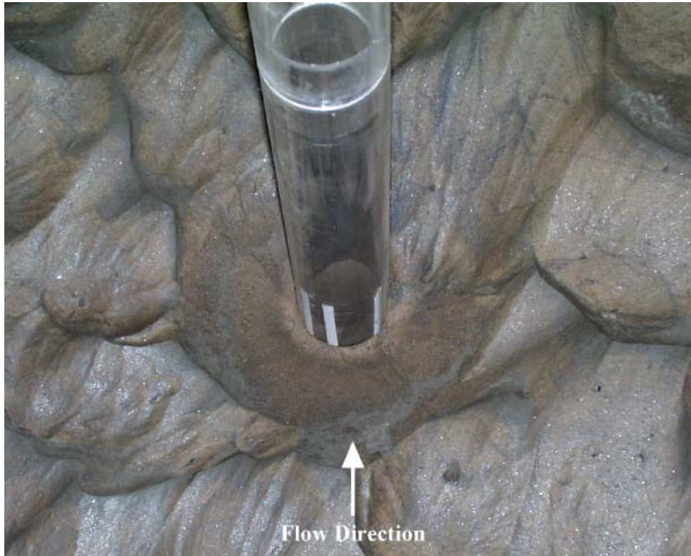
Figure C- 7. Experiment 1 ( D = 0.114 m, D_{50} = 0.22 mm) after test.
