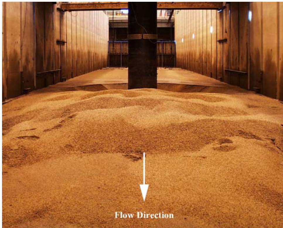
Figure C- 119. Experiment 11 ( D = 0.915 m, D_{50} = 2.90 mm) after test.
