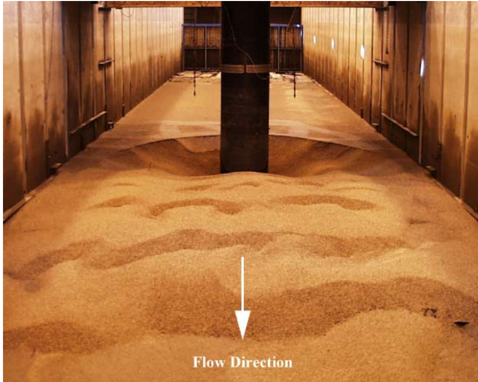
Figure C- 120. Experiment 11 ( D = 0.915 m, D_{50} = 2.90 mm) after test.
