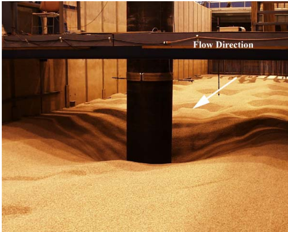
Figure C- 76. Experiment 7 ( D = 0.915 m, D_{50} = 2.90 mm) after test.
