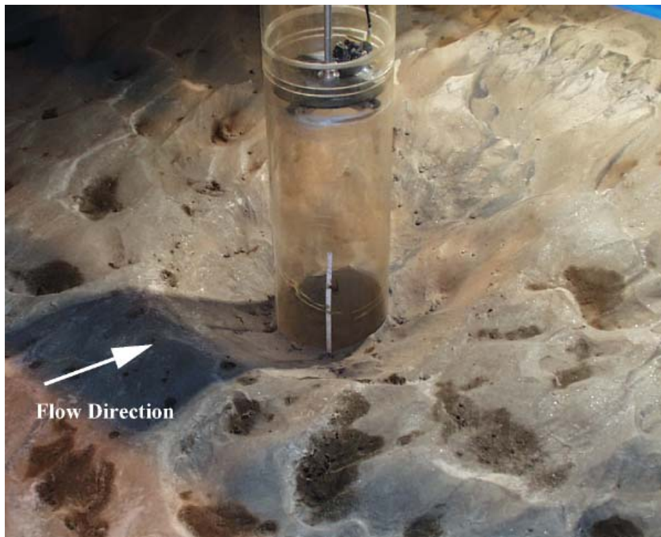
Figure C- 15. Experiment 2 ( D = 0.305 m, D_{50} = 0.22 mm) after test.
