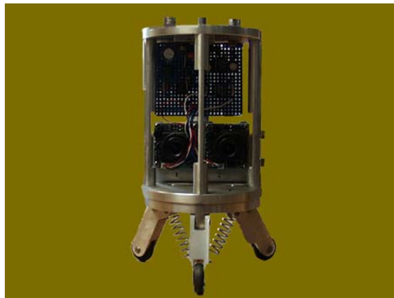
Figure B- 4. The internal cameras for the 0.114 m (4.5 in) diameter cylinder.
