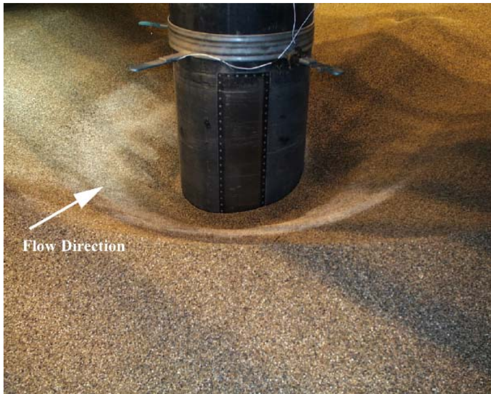
Figure C- 97. Experiment 9 ( D = 0.915 m, D_{50} = 2.90 mm) after test.
