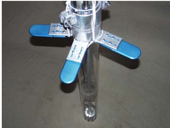
Figure 11. Acoustic transponder arrays on the 0.114 m (4.5 in) diameter cylinder viewed from above.
