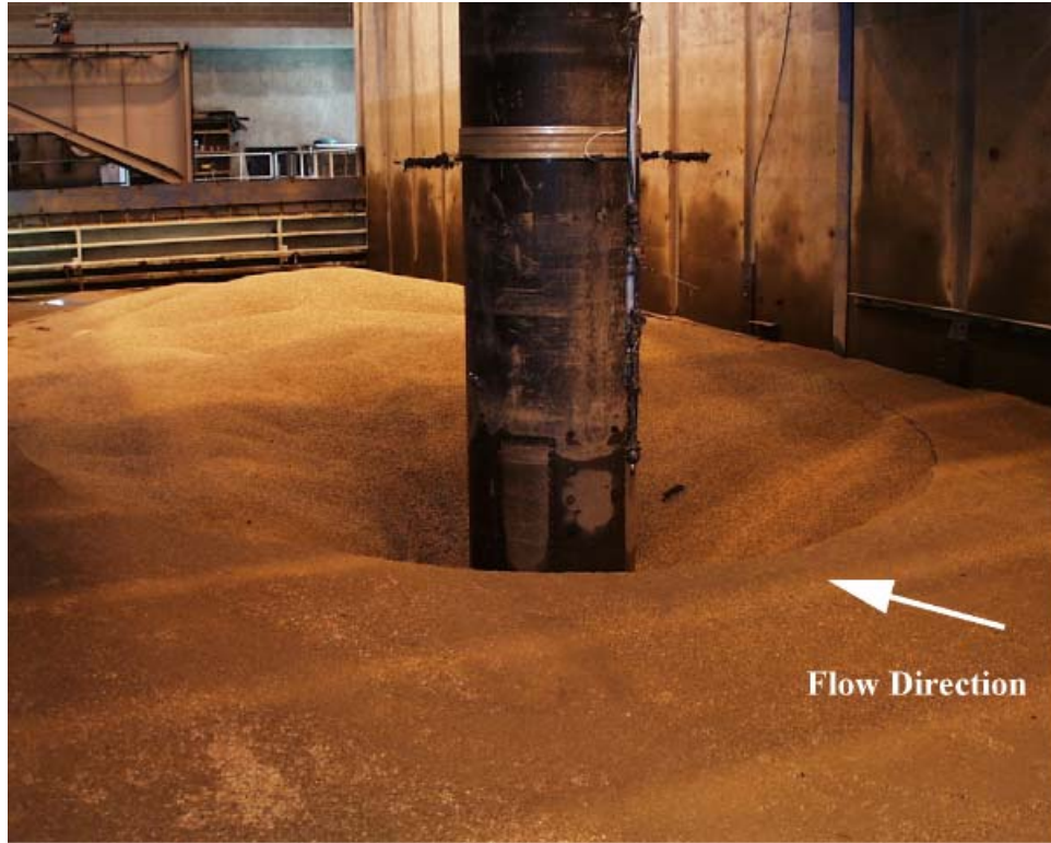
Figure C- 118. Experiment 11 ( D = 0.915 m, D_{50} = 2.90 mm) after test.
