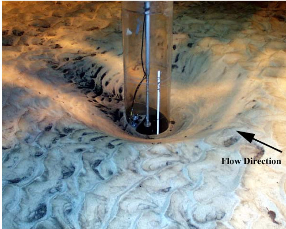
Figure C- 133. Experiment 12 ( D = 0.305 m, D_{50} = 0.22 mm) after test.
