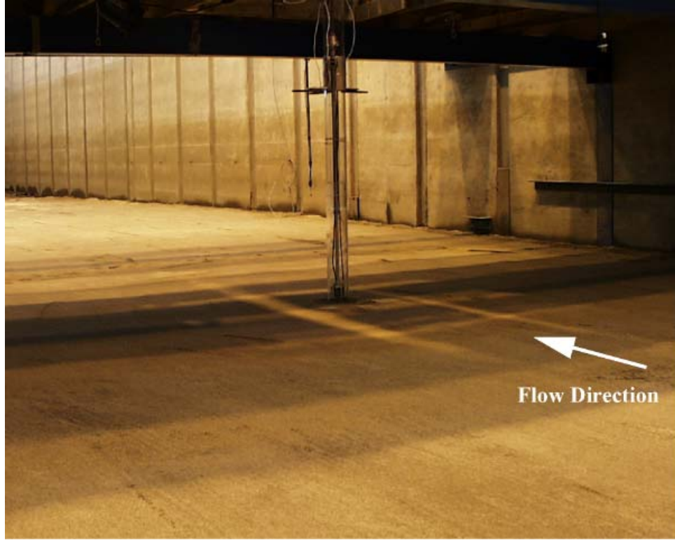
Figure C- 5. Experiment 1 ( D = 0.114 m, D_{50} = 0.22 mm) before test.
