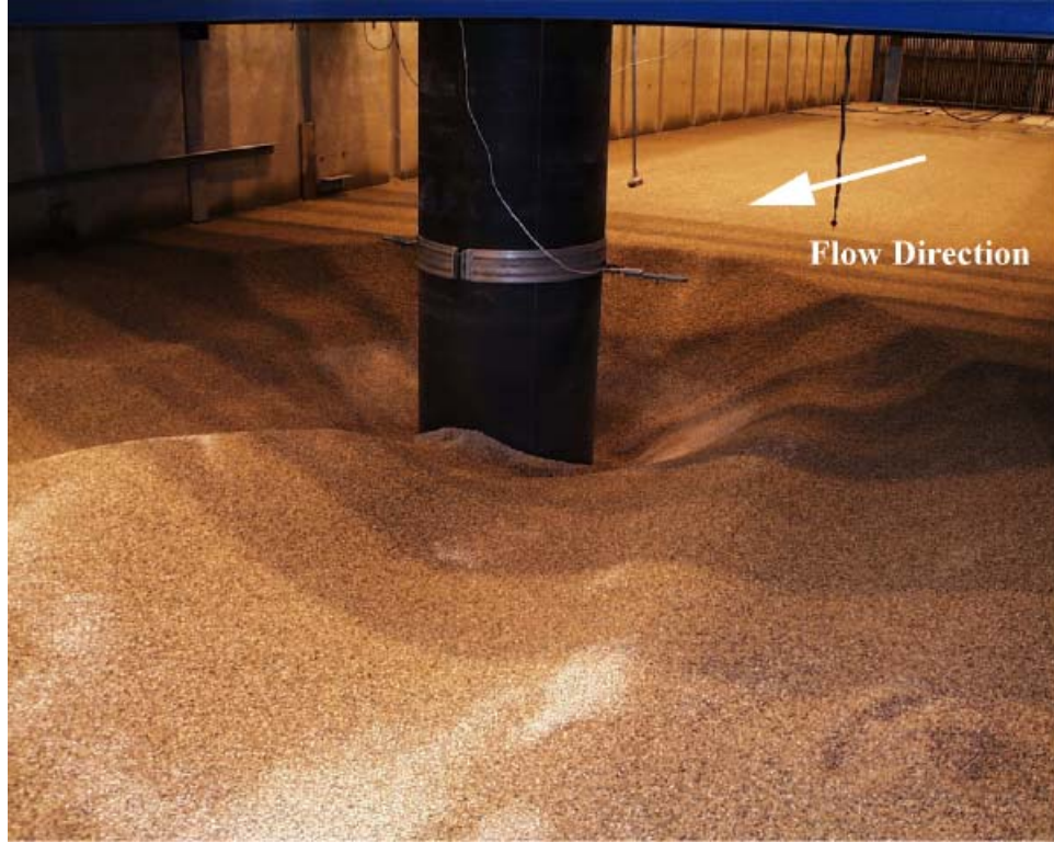
Figure C- 94. Experiment 9 ( D = 0.915 m, D_{50} = 2.90 mm) after test.
