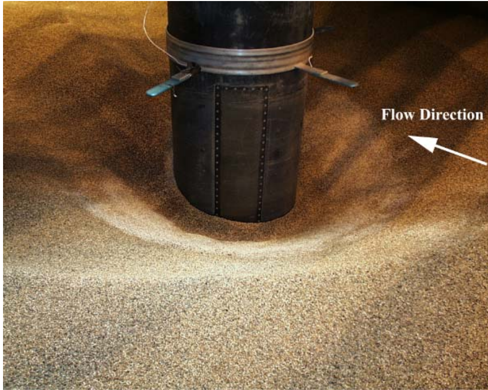
Figure C- 98. Experiment 9 ( D = 0.915 m, D_{50} = 2.90 mm) after test.
