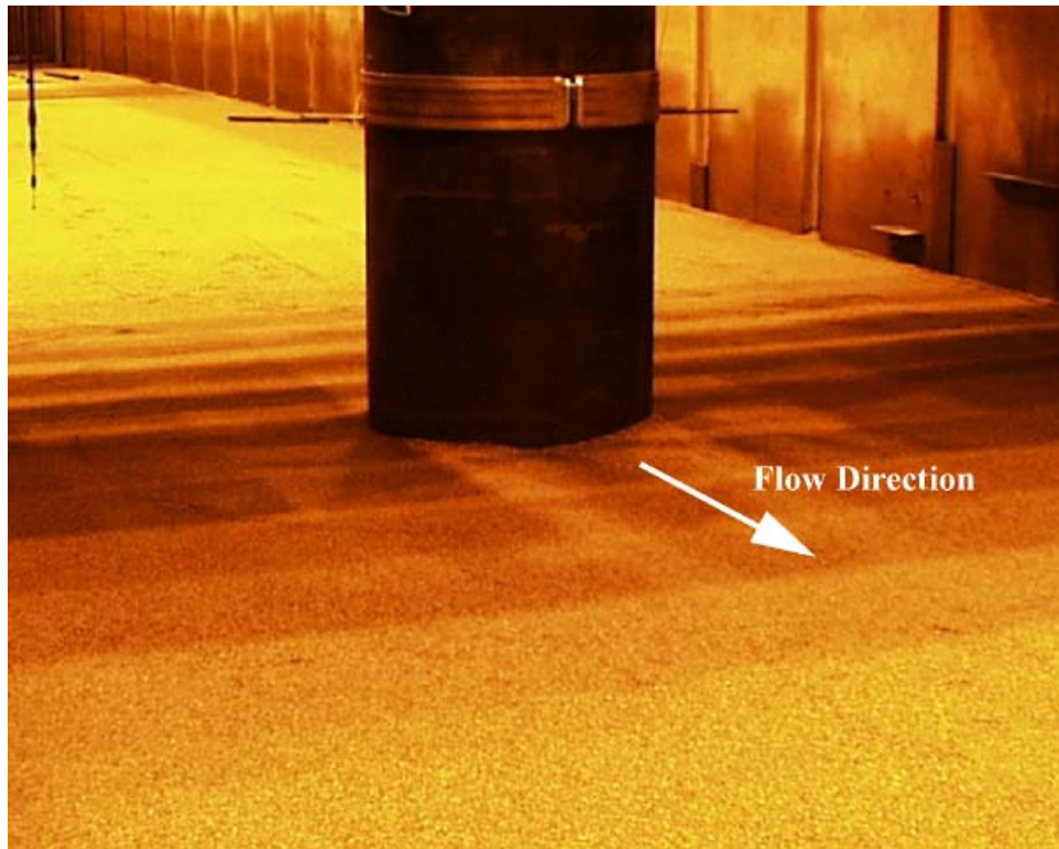
Figure C- 71. Experiment 7 ( D = 0.915 m, D_{50} = 2.90 mm) before test.
