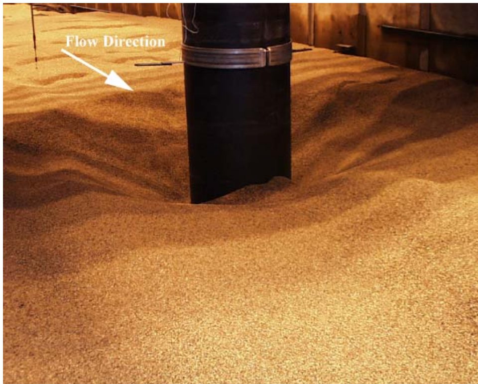
Figure C- 88. Experiment 8 ( D = 0.915 m, D_{50} = 2.90 mm) after test.
