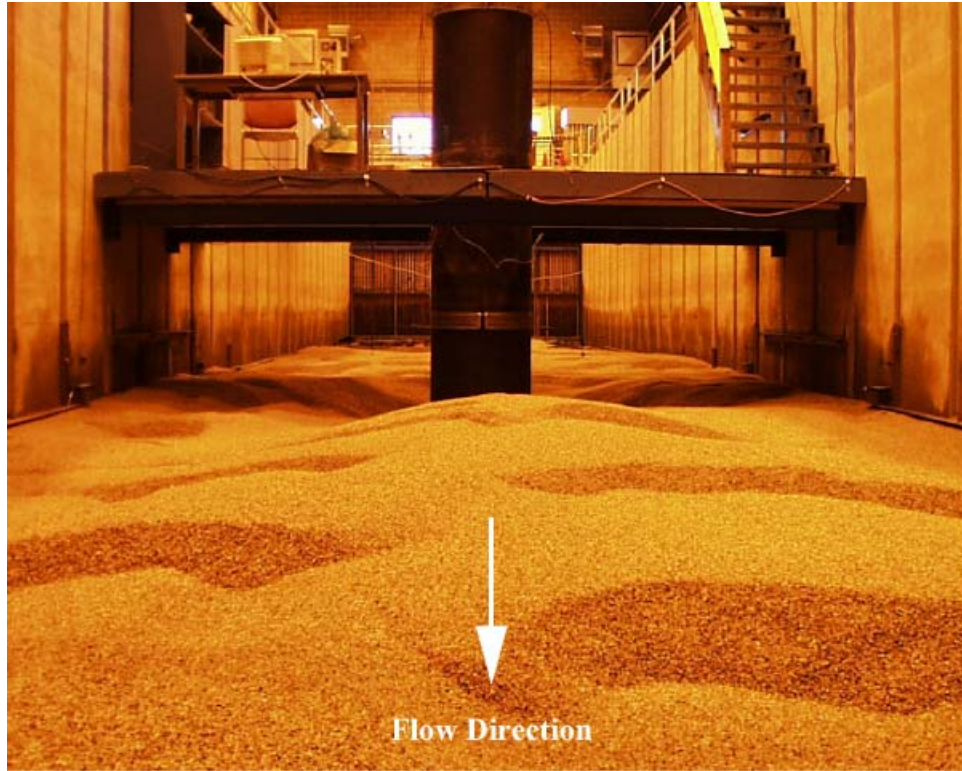
Figure C- 85. Experiment 8 ( D = 0.915 m, D_{50} = 2.90 mm) after test.
