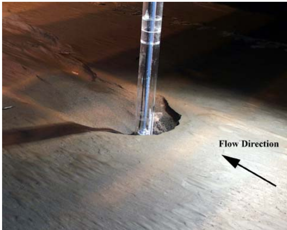
Figure C- 60. Experiment 6 ( D = 0.114 m, D_{50} = 0.80 mm) after test.
