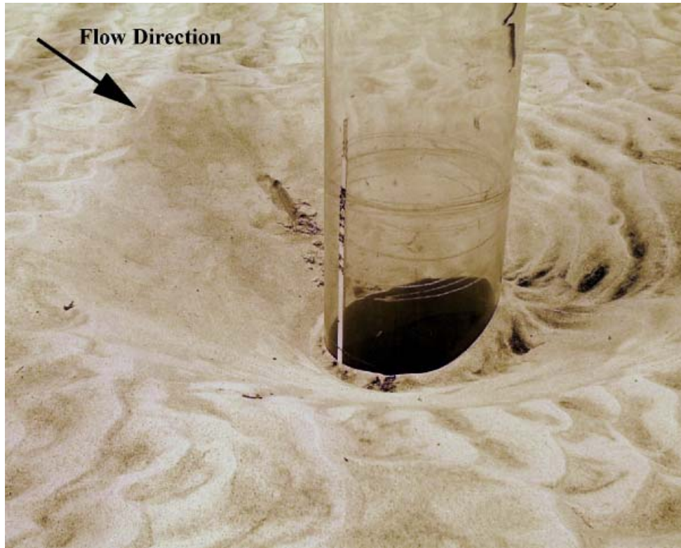
Figure C- 149. Experiment 13 ( D = 0.305 m, D_{50} = 0.22 mm) after the test.
