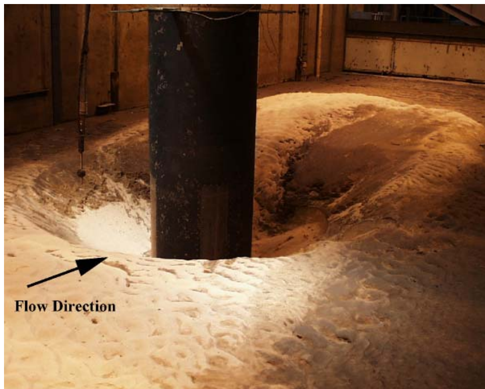
Figure C- 163. Experiment 14 ( D = 0.915 m, D_{50} = 0.22 mm) after the test.
