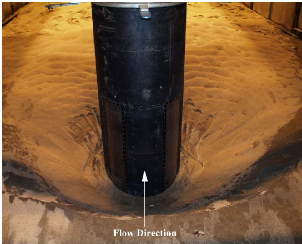
Figure C- 25. Experiment 3 ( D = 0.915 m, D_{50} = 0.80 mm) after test.
