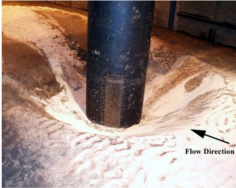
Figure C- 160. Experiment 14 ( D = 0.915 m, D_{50} = 0.22 mm) after test.
