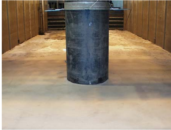
Figure E- 2. Pre-test photograph of test bed ( D = 0.915 m, D_{50} = 0.22 mm).
