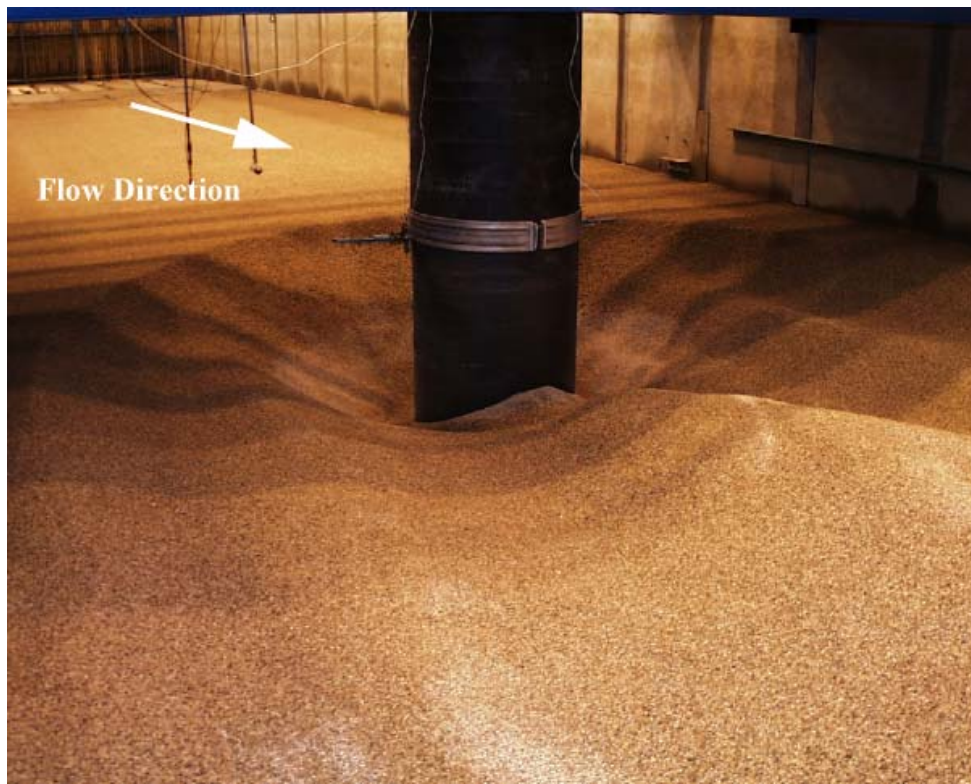
Figure C- 93. Experiment 9 ( D = 0.915 m, D_{50} = 2.90 mm) after test.
