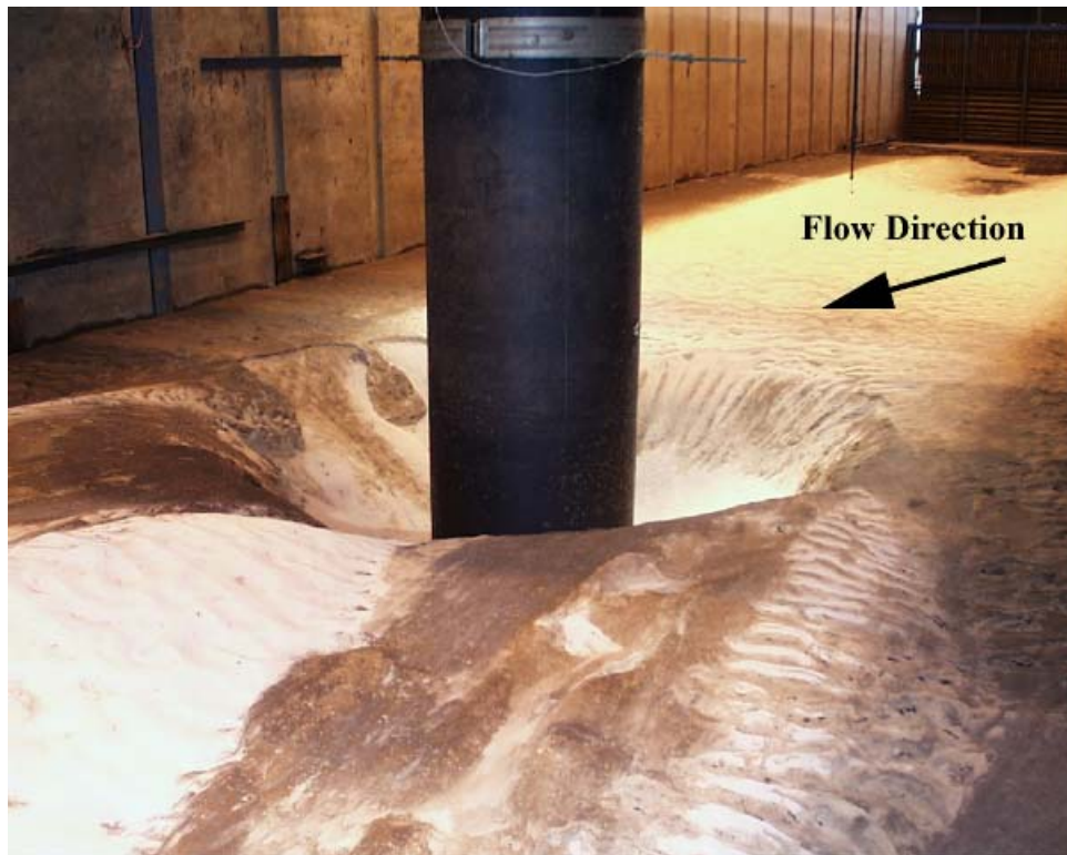
Figure C- 165. Experiment 14 ( D = 0.915 m, D_{50} = 0.22 mm) after the test.
