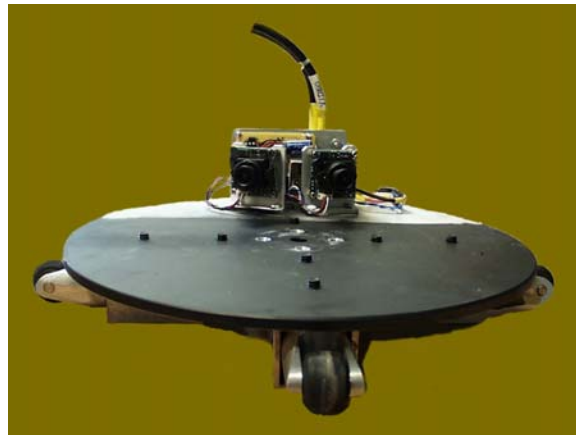
Figure 7. Internal video cameras and housing for the 0.305 m (1 ft) diameter cylinder.
