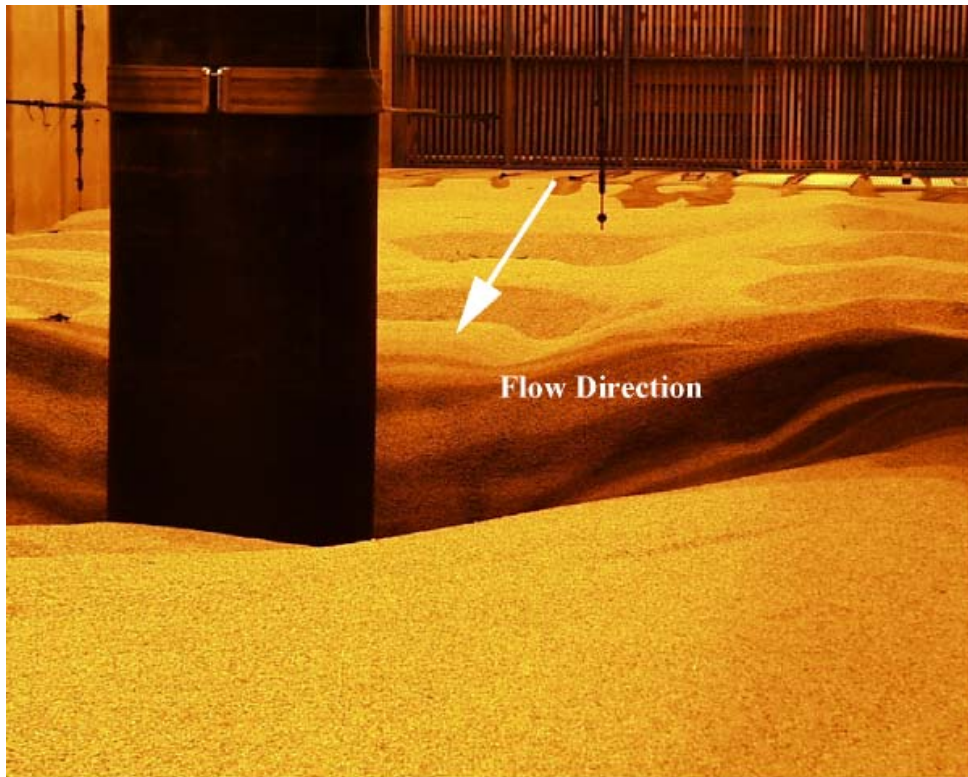
Figure C- 77. Experiment 7 ( D = 0.915 m, D_{50} = 2.90 mm) after test.
