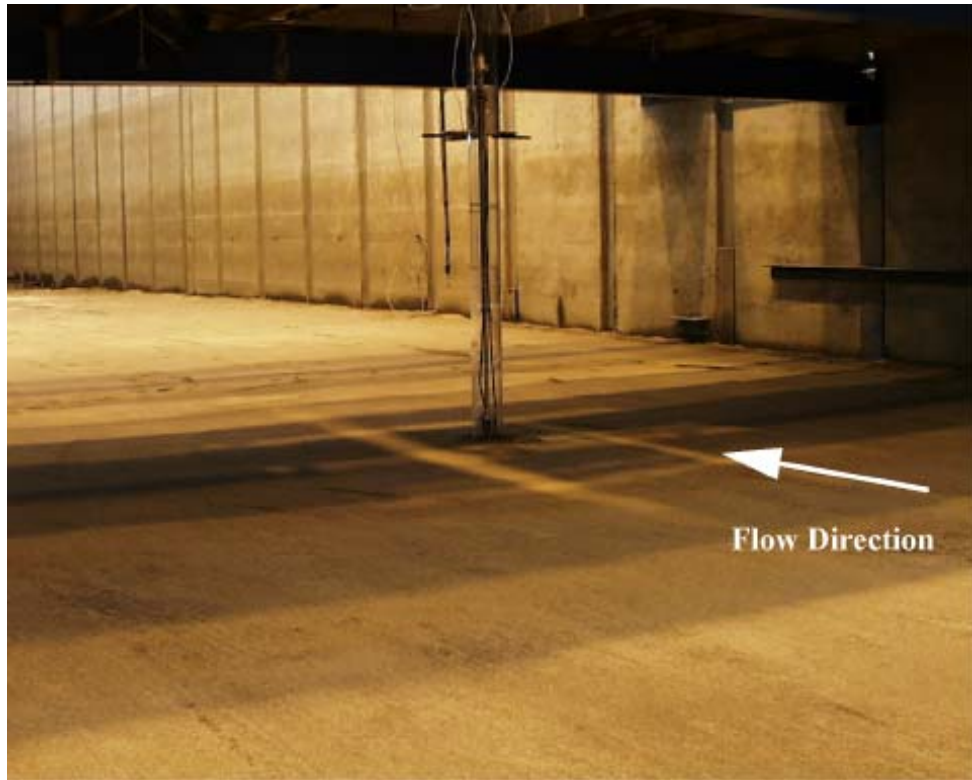
Figure C- 57. Experiment 6 ( D = 0.114 m, D_{50} = 0.80 mm) before test.
