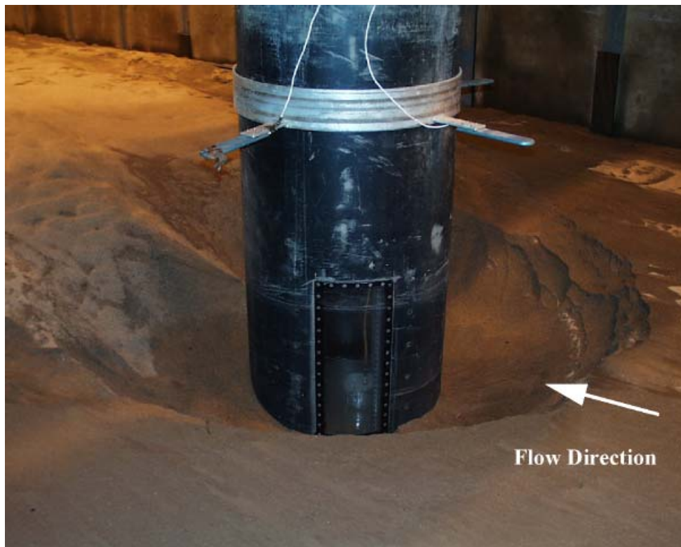
Figure C- 37. Experiment 4 ( D = 0.915 m, D_{50} = 0.80 mm) after test.
