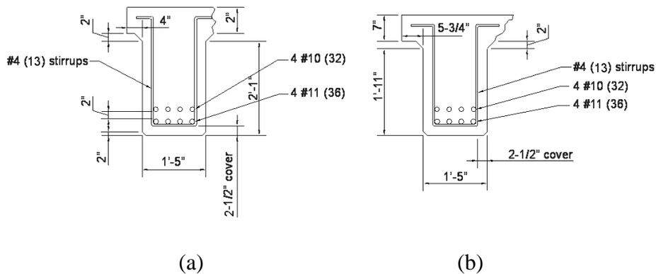
Figure 83—Cross-section of (a) Girder #1, and (b) Girder #2
