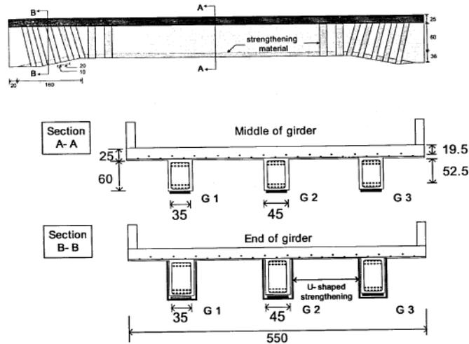
Figure 45—FRP strengthening details (Sim et al., 2006)
