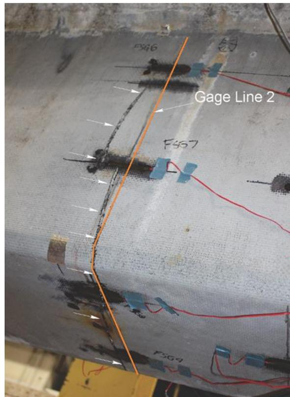
Figure 117—CFRP rupture relative to Gage Line 2 on Girder #1
