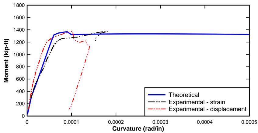
Figure 203—Moment curvature of Girder 4-1
