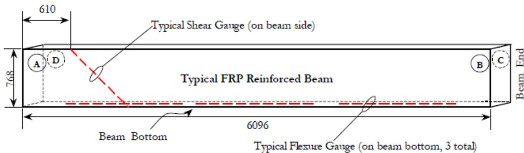
Figure 52—Location of fiber optic strain gauges (Kachlakev and McCurry, 2000)
