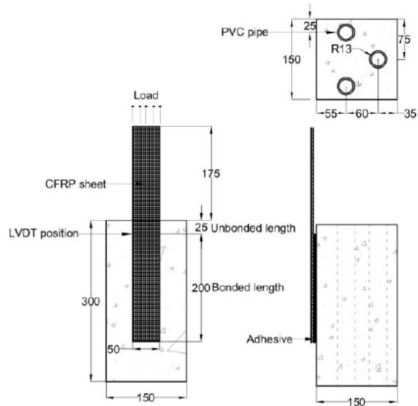
Figure 25—Direct shear test specimen (Srestha et al., 2013)
