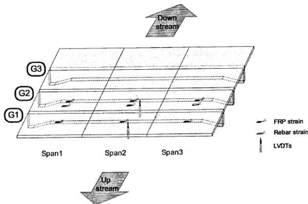
Figure 46—Location of instrumentation (Sim et al., 2006)
