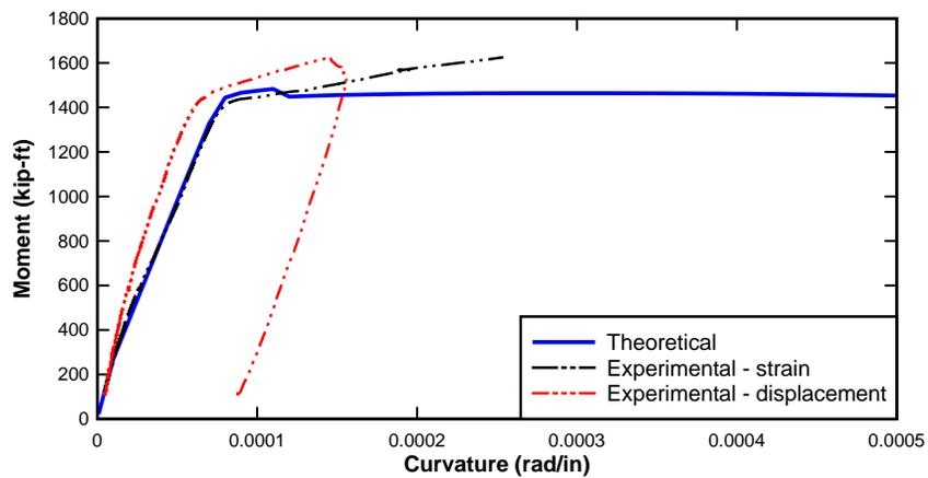
Figure 208—Moment curvature of Girder 4-3
