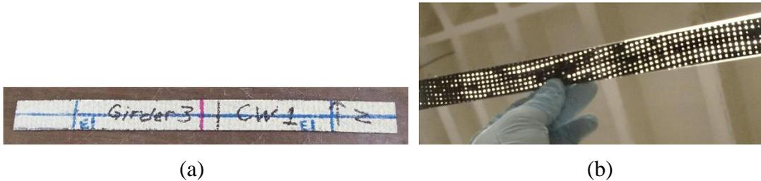
Figure 263—CFRP samples: (a) from east face with coating (b) from west face without coating
