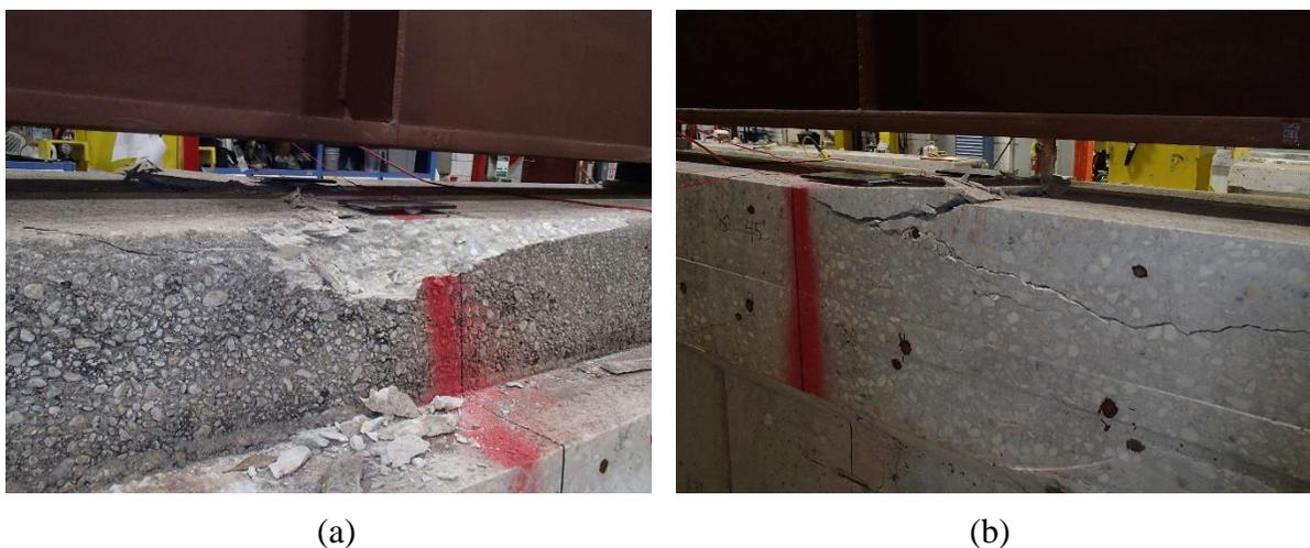
Figure 181—Damage to Girder 4-1 including (a) compression failure on east elevation (b) compression failure on west elevation
