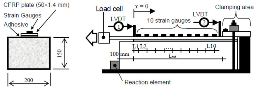
Figure 17—Direct shear test setup (Fava et al., 2007)
