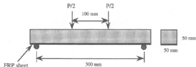
Figure 8—Four-point bending test setup (Toutanji and Gomez, 1997)
