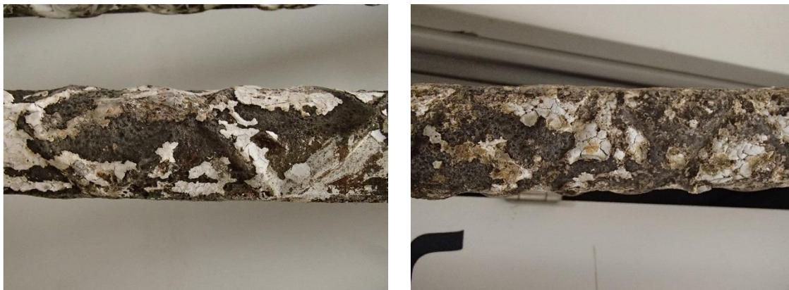
Figure 126—Close-up images of corroded reinforcement
