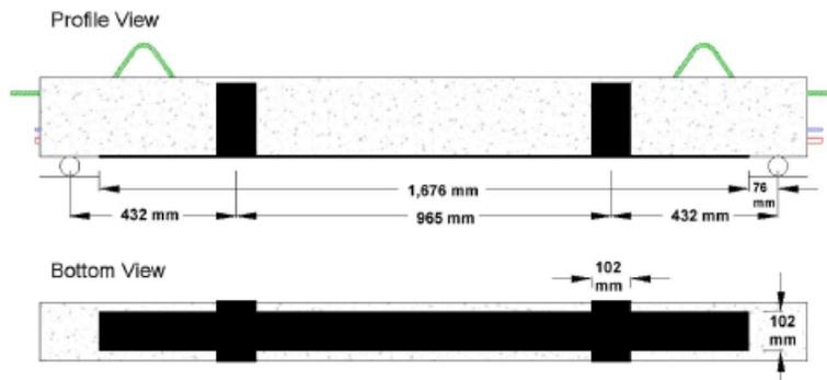
Figure 34—Wrapping scheme 2 (Davalos et al., 2012)
