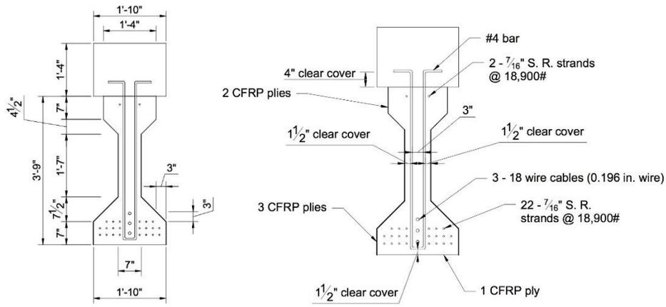
Figure 228—Typical beam section (a) original and (b) with CFRP repair
