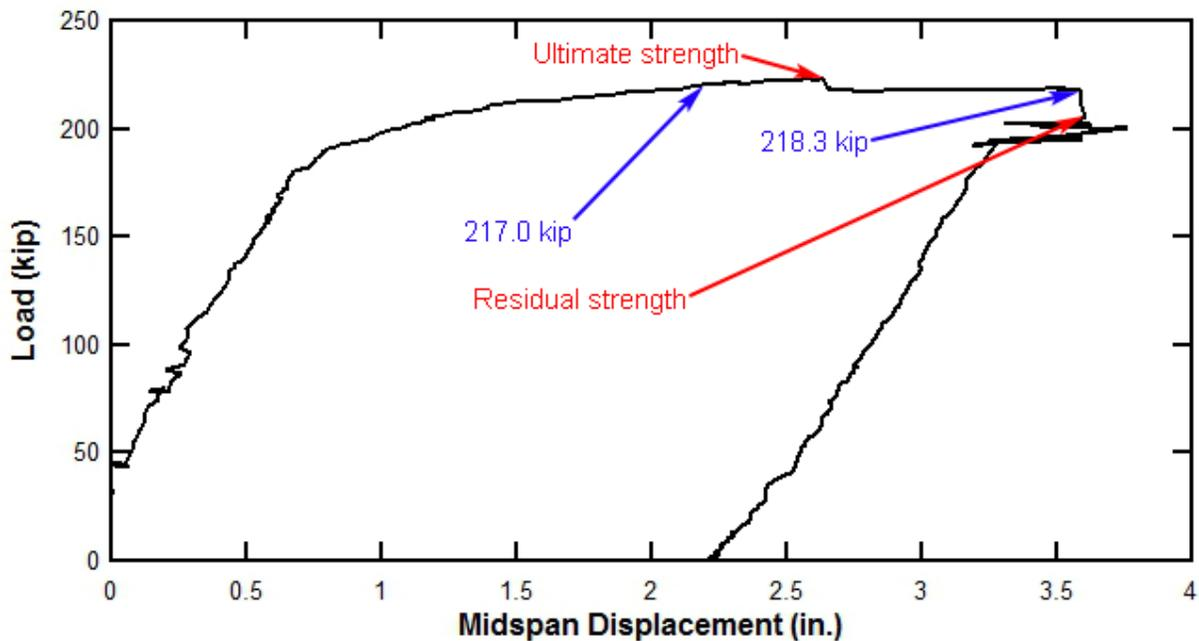
Figure 172—Load vs. displacement plot for Girder 3-4
