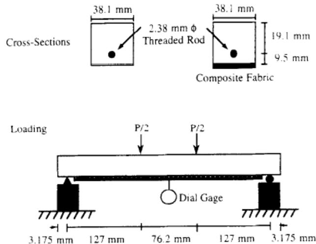
Figure 6—Four-point bending test setup (Chajes et al., 1995)
