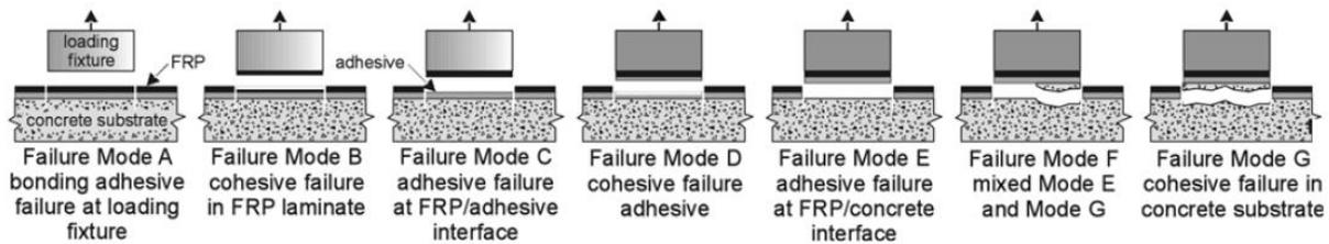
Figure 60—Failure modes for pull-off test (ASTM D7522)
