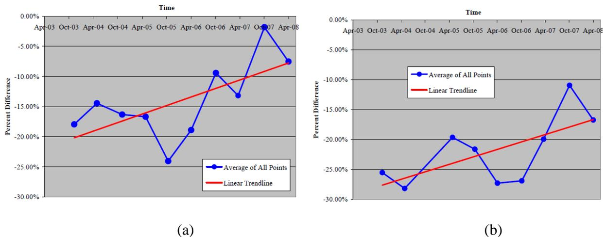
Figure 47—Average deflection percent difference for bridge: (a) P-962 and (b) T-530
