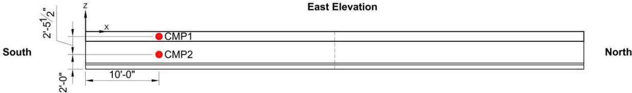
Figure 230—Typical coring locations for compression cores
