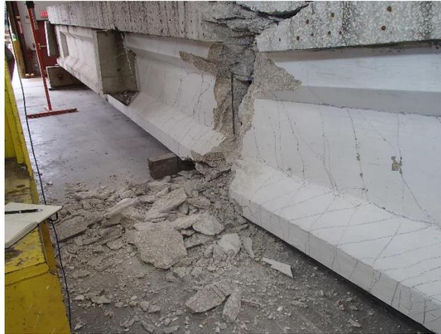
Figure 247—Girder 1 failed at the end of the repaired region
