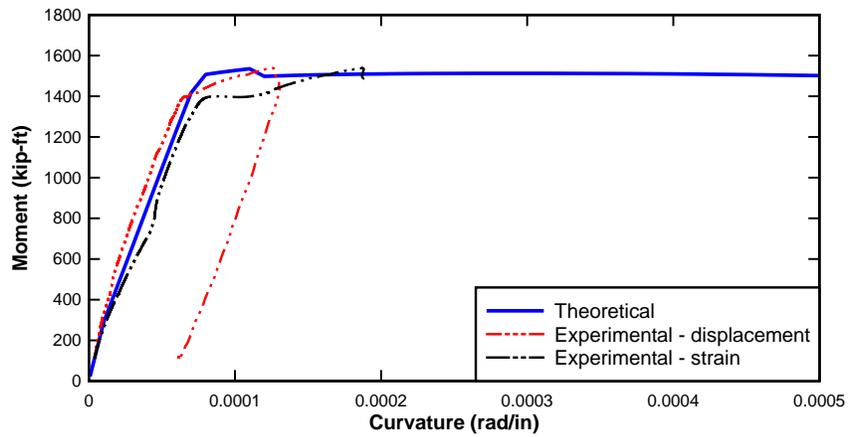
Figure 207—Moment curvature of Girder 4-2
