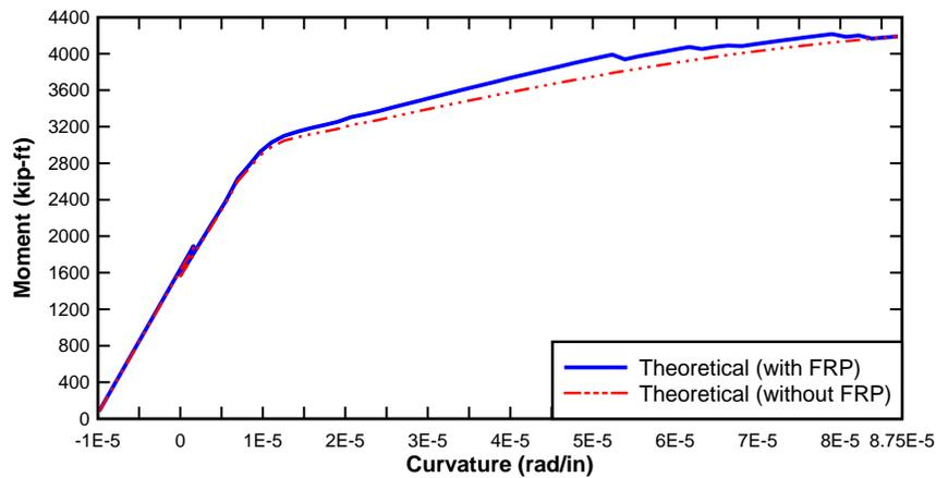
Figure 260—Girder 3 comparison of the theoretical ultimate capacity with and without FRP
