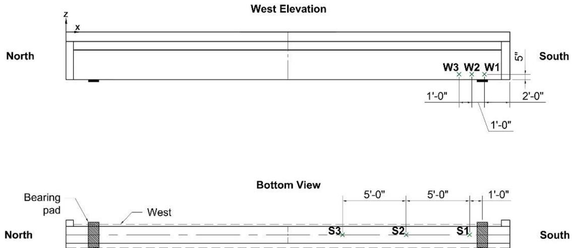
Figure 141—Typical potential testing locations for interior girders
