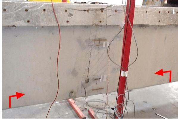
Figure 191—Red arrows indicate the span of debonded CFRP strip (Girder 3-2)
