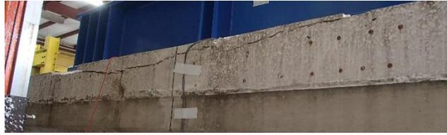
Figure 246—Concrete crushing in compression zone
