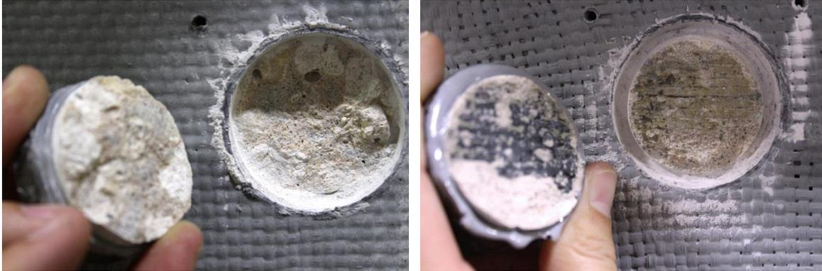
Figure 102—Failure mode: (a) cohesive and (b) adhesive
