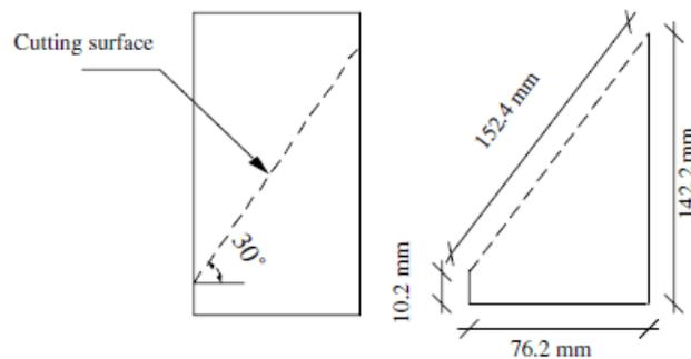
Figure 16—Slant shear test specimen (Frigione et al., 2006)
