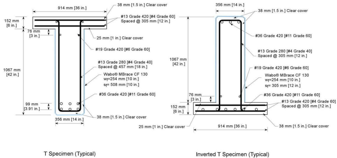
Figure 56—Typical T and inverted-T specimen design (Higgins et al., 2009)
