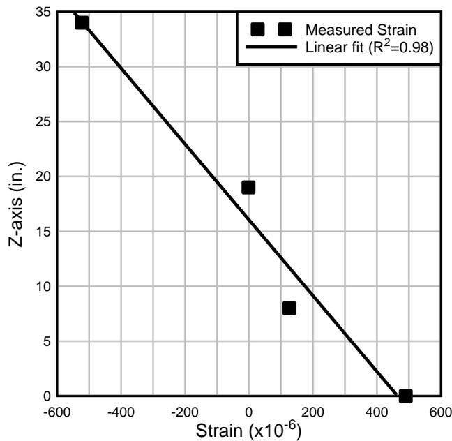
Figure 114—Typical strain profile along the girder depth
