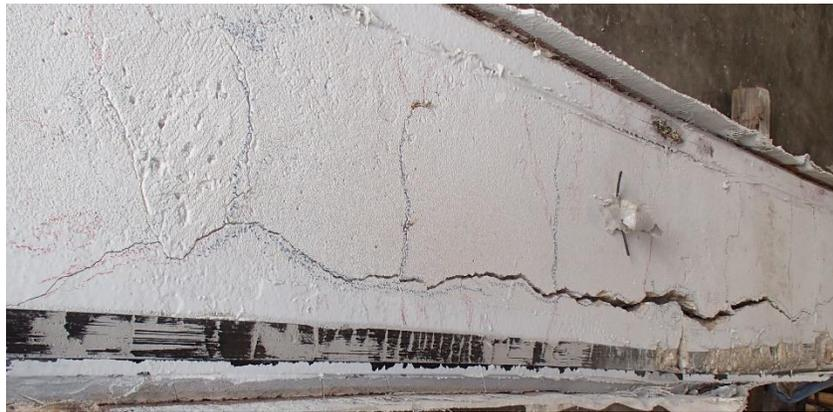
Figure 199—Longitudinal cracking on the tension face of Girder 4-3
