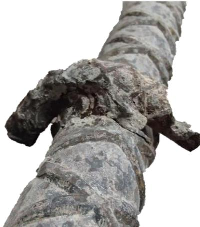
Figure 147—Stirrup remaining on steel reinforcement sample
