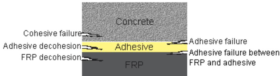
Figure 1—Possible failure modes in FRP-concrete bond system
