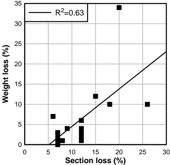
Figure 148—Correlation between weight loss and section loss
