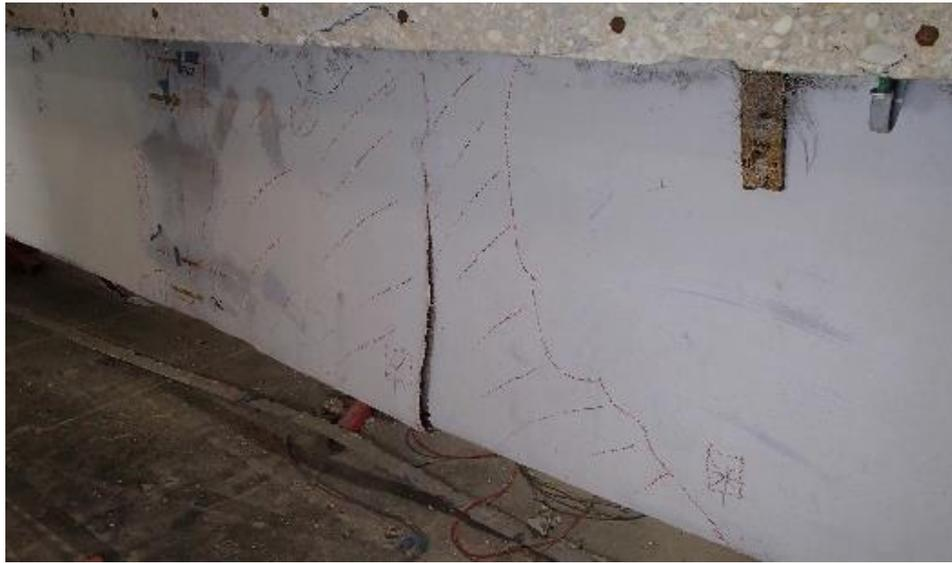
Figure 174—GFRP rupture (Girder 3-4)
