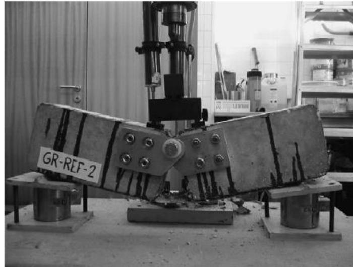
Figure 19—Hinged beam specimen (Silva and Biscaia, 2008)
