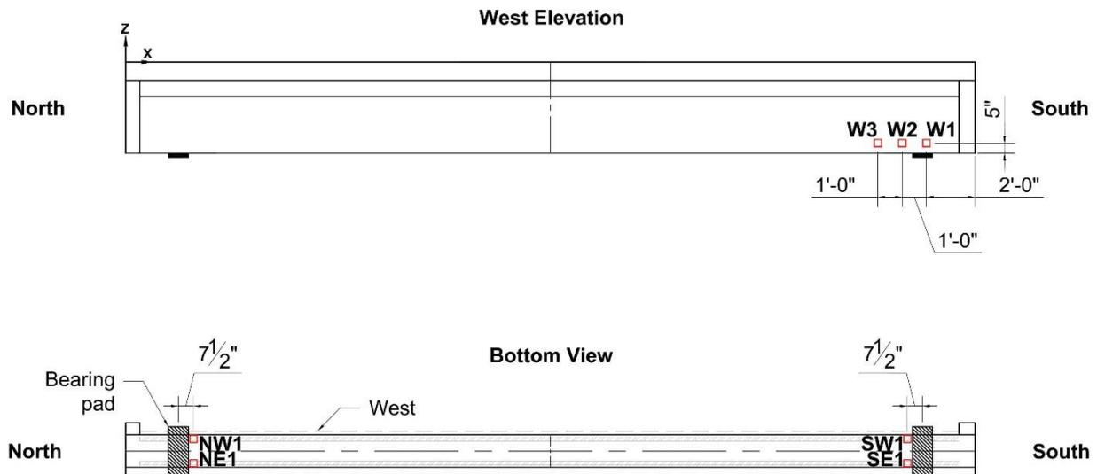
Figure 154—Direct pull-off testing locations for interior girders
