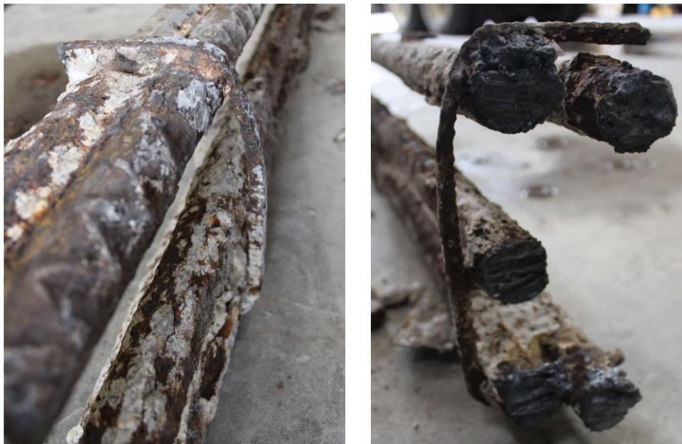
Figure 145—Steel reinforcement welded together with stirrups
