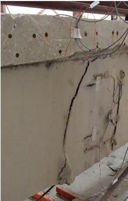
Figure 197—GFRP rupture on east elevation (Girder 4-3)
