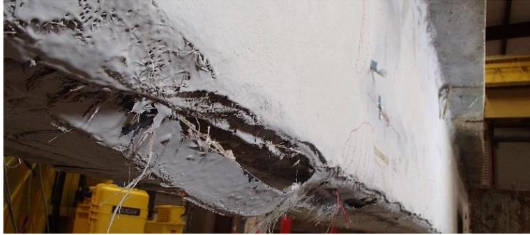
Figure 173—CFRP debonding (Girder 3-4)
