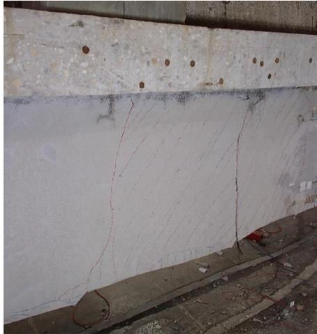
Figure 184—GFRP rupture (Girder 4-4)
