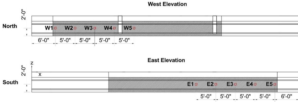
Figure 235—Direct pull-off testing locations for Girder 2
