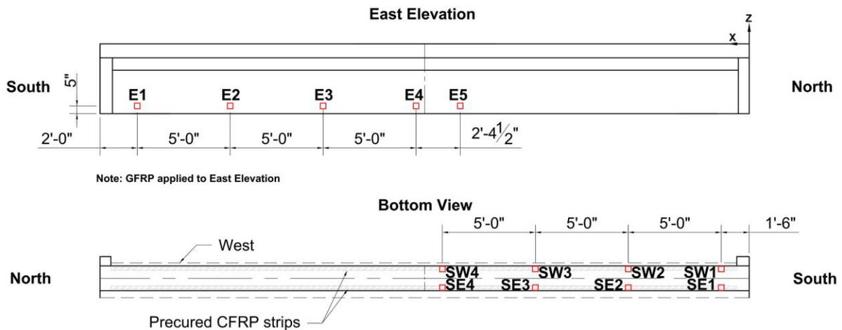
Figure 151—Direct pull-off testing locations for Girder 3-1
