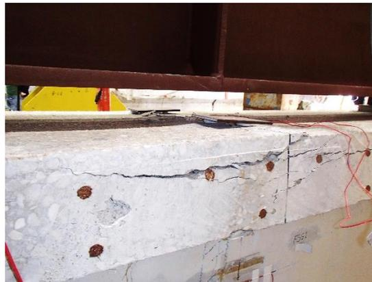
Figure 190—Crushing of concrete in compression (east elevation view of Girder 3-2)
