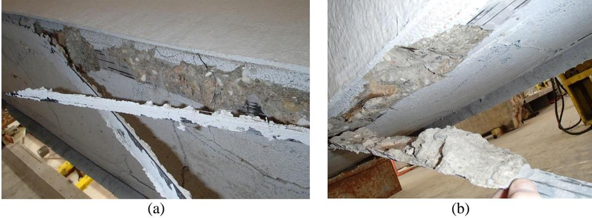
Figure 198—CFRP on east elevation (Girder 4-3): (a) ruptured (b) debonded
