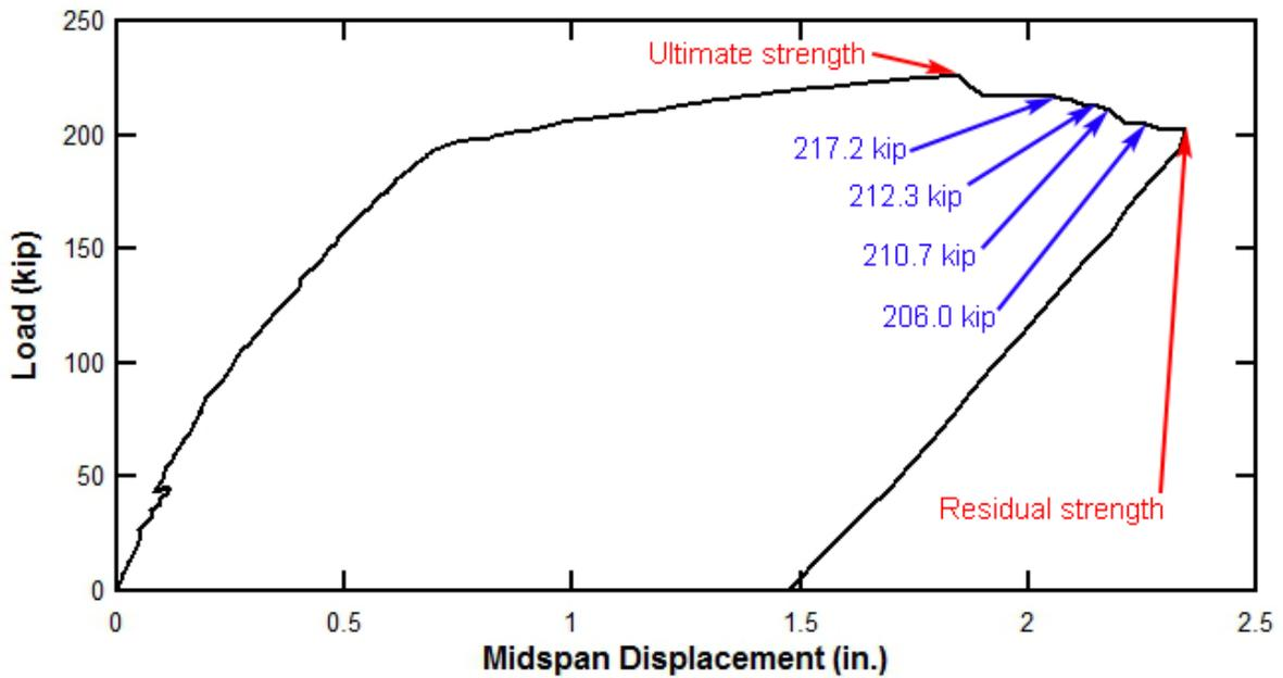
Figure 182—Load vs Displacement plot for Girder 4-4
