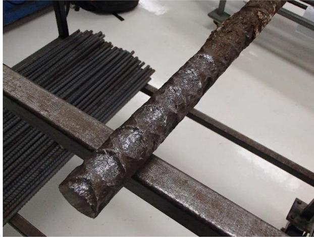
Figure 144—Reinforcement with bare metal exposed
