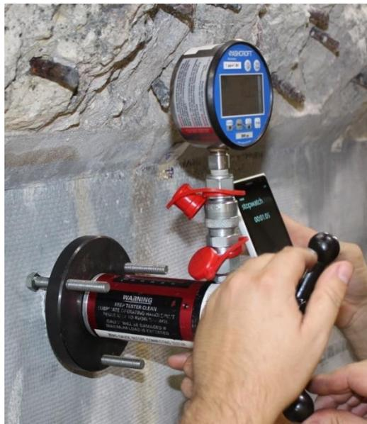
Figure 101—Direct pull-off test setup
