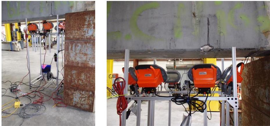
Figure 85—Heating of CFRP surface with halogen lamps
