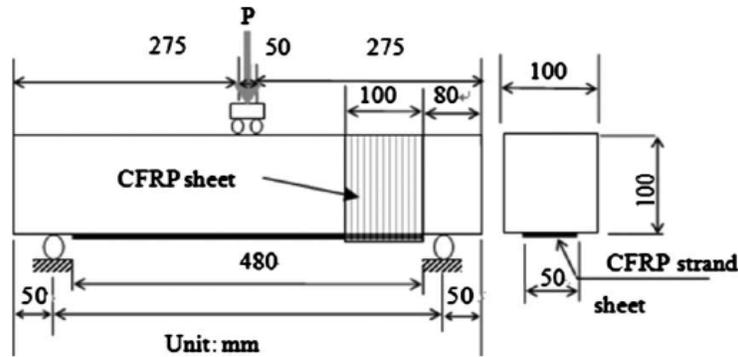
Figure 21—Three-point bending test setup (Dai et al., 2010)
