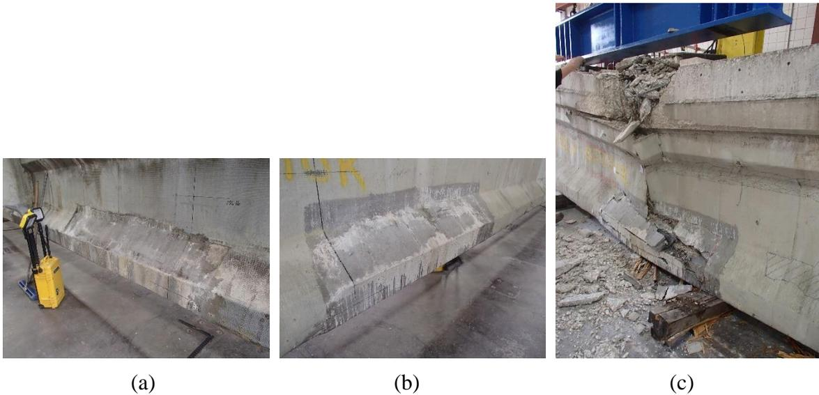
Figure 249—Repaired region of Girder 2: (a) west face initially before testing (b) east face initially before testing (c) east face after failure
