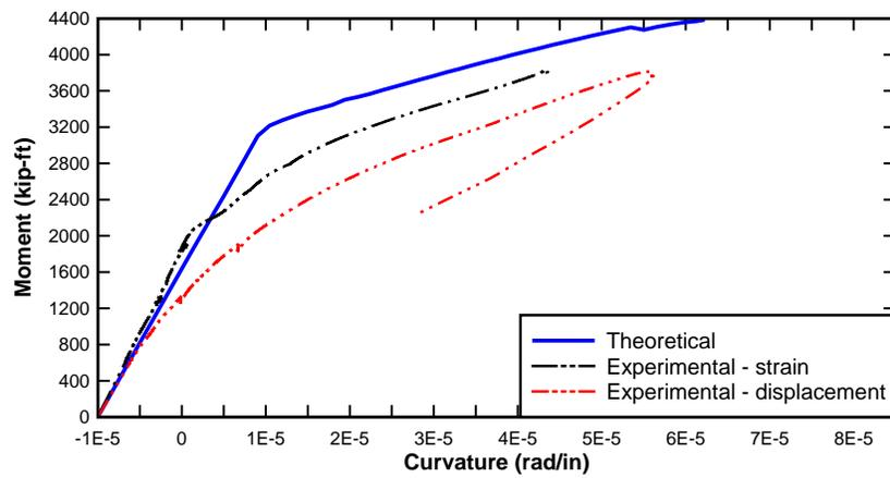
Figure 254—Moment curvature of Girder 2
