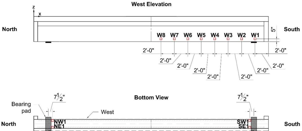
Figure 152—Direct pull-off testing locations for exterior girders
