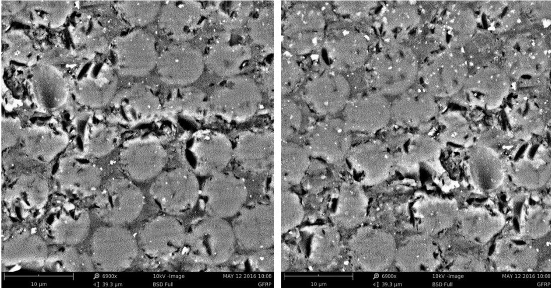
Figure 161—Examples of damage distributed within the CFRP
