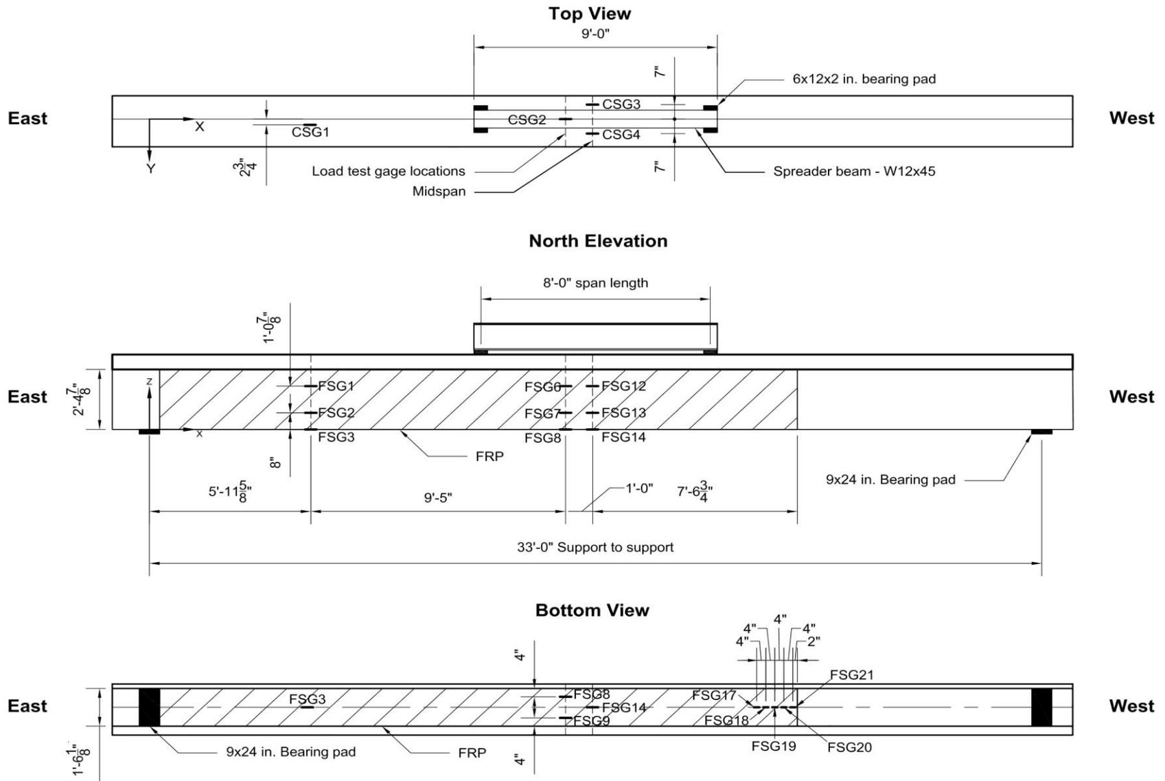
Figure 109—Girder #2 – Instrumentation plan representing the locations for the strain gages
