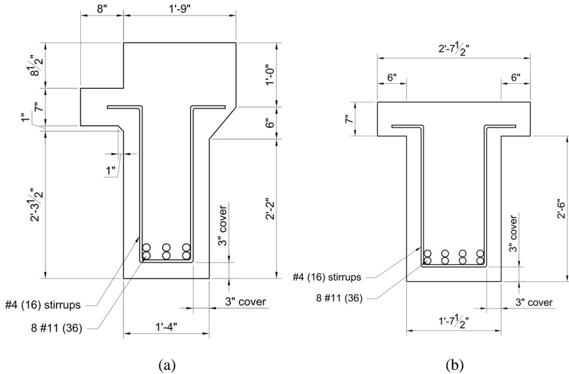
Figure 134—Typical cross-section for (a) Girders 3-1, 3-4, 4-1, 4-4, and 5-1 and (b) Girders 3-2, 4-2, 4-3 and 5-2
