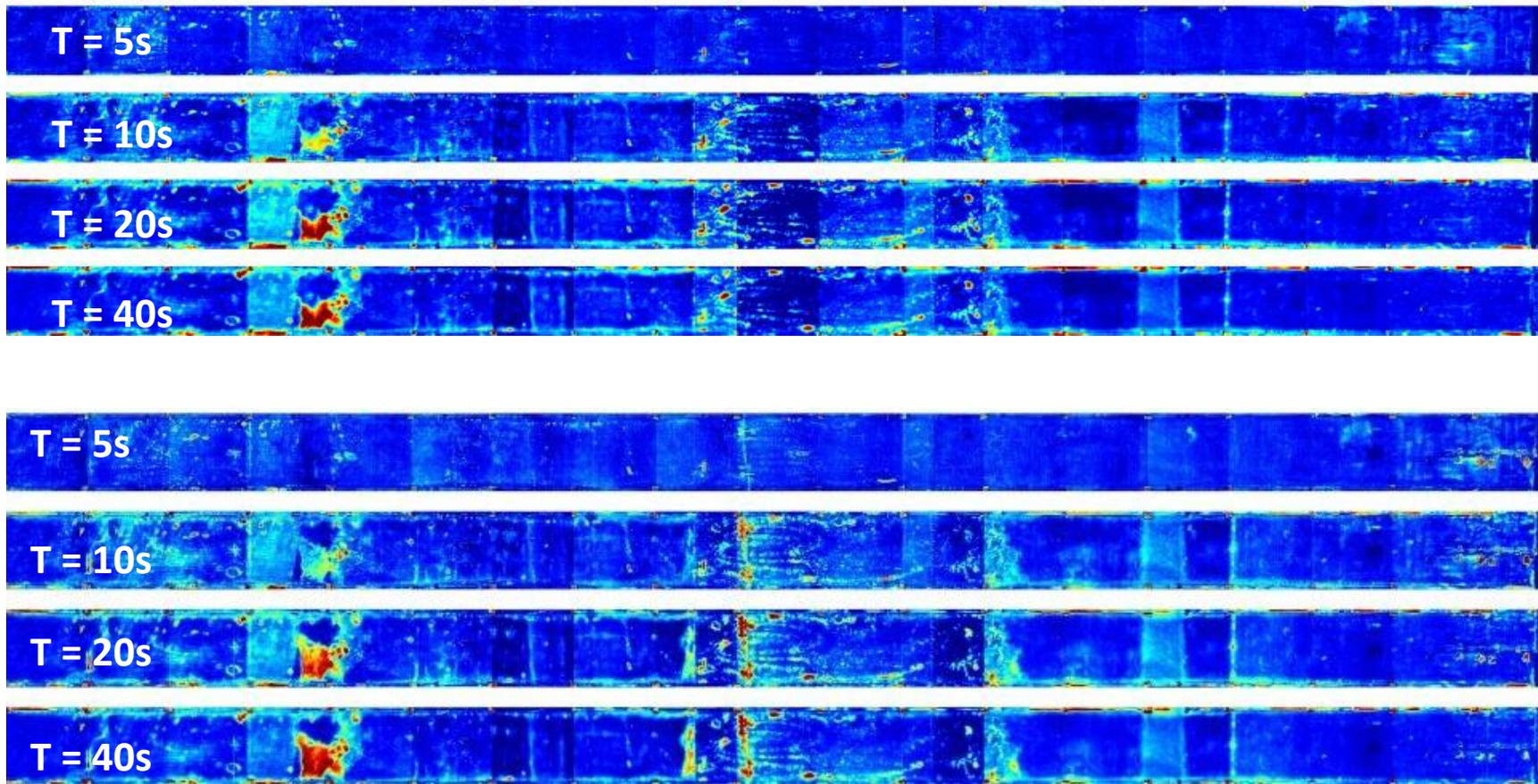
Figure 91—Girder #2 – bottom: prior to structural test (top), and after structural test (bottom)
