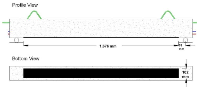
Figure 33—Wrapping scheme 1 (Davalos et al., 2012)
