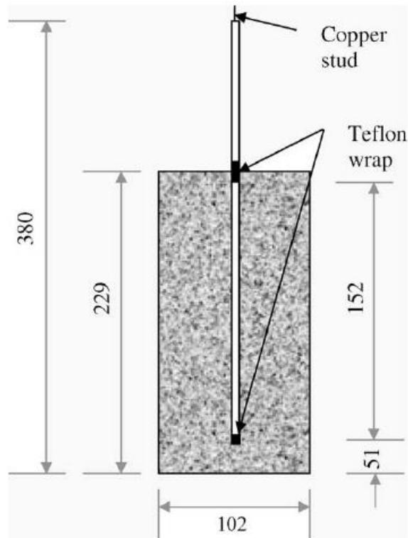
Figure 267—Gadve et al. (2009): Cylindrical reinforced concrete specimen
