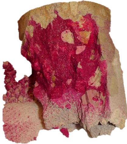
Figure 95—Concrete carbonation examined on a concrete cylinder following the compression test
