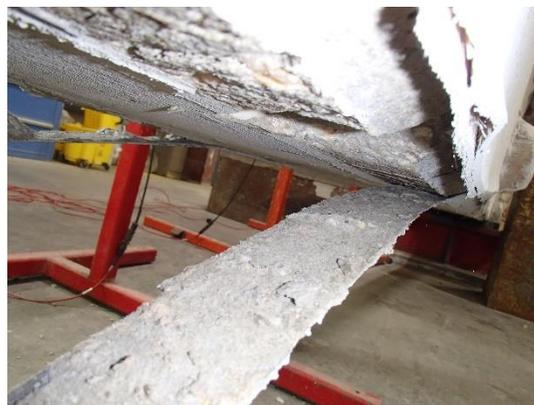
Figure 177—Debonded CFRP strips (Girder 4-1)
