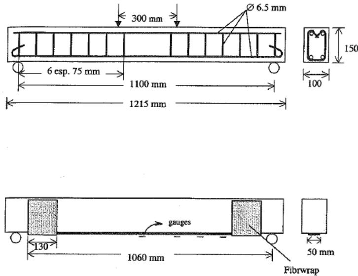
Figure 9—Four-point bending test setup (Beaudoin et al., 1998)
