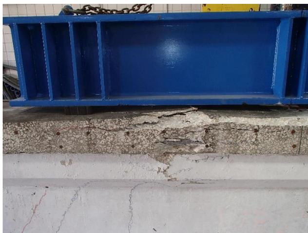
Figure 252—Concrete crushing in the compression zone
