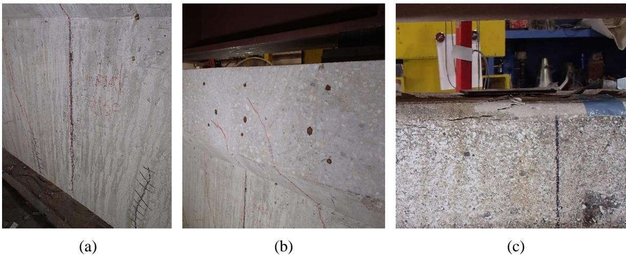
Figure 185—Damage to Girder 4-4 including (a) cracking at formwork joint (b) crack at formwork joint extended to compression zone in east elevation (c) crushing of concrete in west elevation
