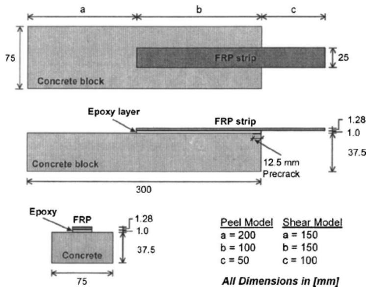
Figure 14—Direct shear/peel test specimen (Au and Buyukozturk, 2006)
