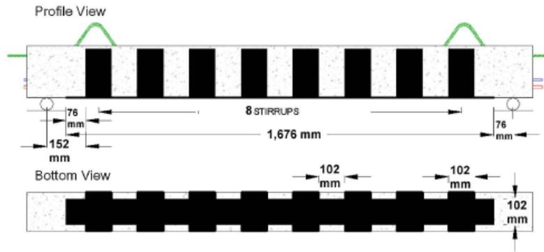
Figure 35—Wrapping scheme 3 (Davalos et al., 2012)
