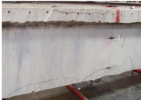
Figure 195—GFRP debonding by midspan on west elevation (Girder 4-2)
