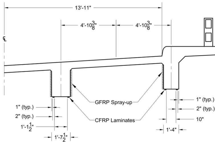
Figure 135—Typical partial cross-section of the bridge span with FRP installed
