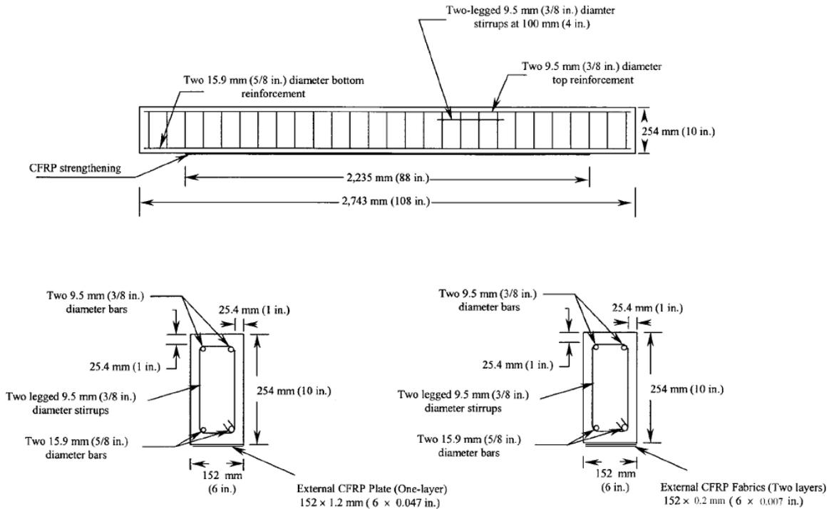
Figure 12—Drawings of test specimen (Grace and Singh, 2005)
