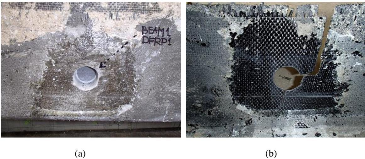
Figure 123—Evidence of delaminated bond surface along the CFRP-epoxy interface on: (a) the girder and (b) CFRP wrap
