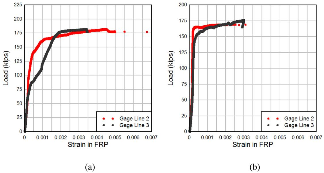
Figure 116—Development of strain in CFRP at the bottom of (a) Girder #1, and (b) Girder #2
