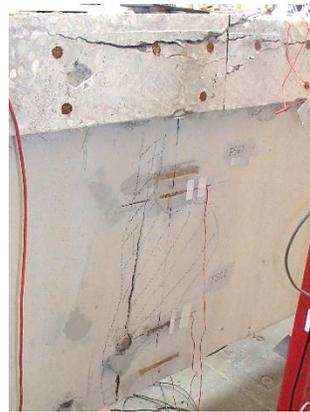
Figure 192—GFRP rupture and GFRP debonding indicated in hatch (Girder 3-2)
