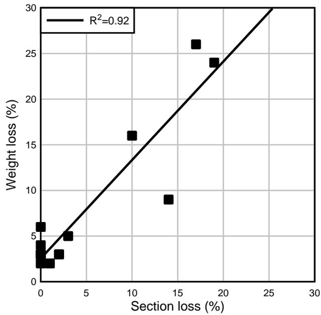
Figure 99—Correlation between weight loss and section loss
