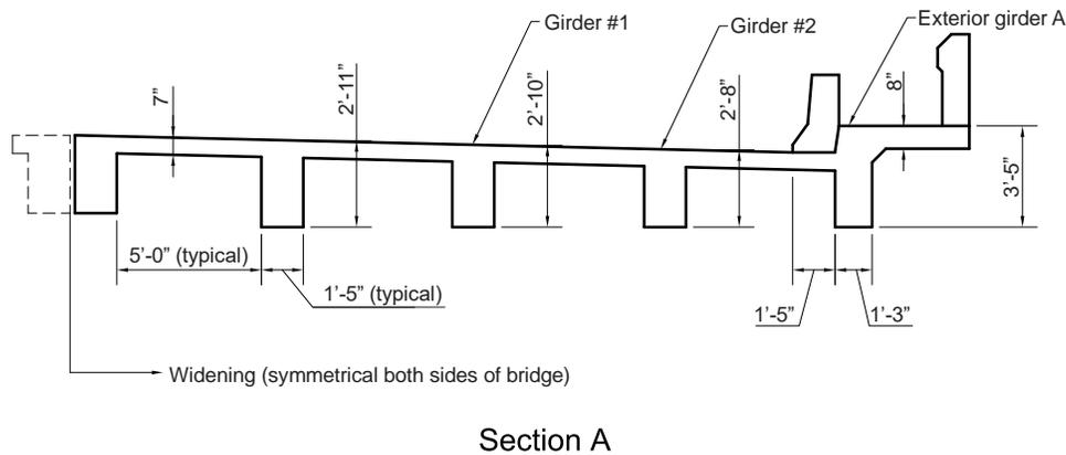
Figure 79—Cross-section view of widened portion of Indian River Bridge
