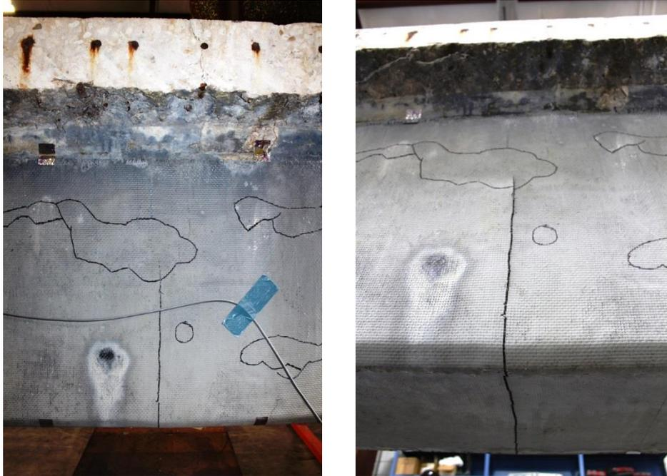
Figure 113—Rupture of CFRP near midspan
