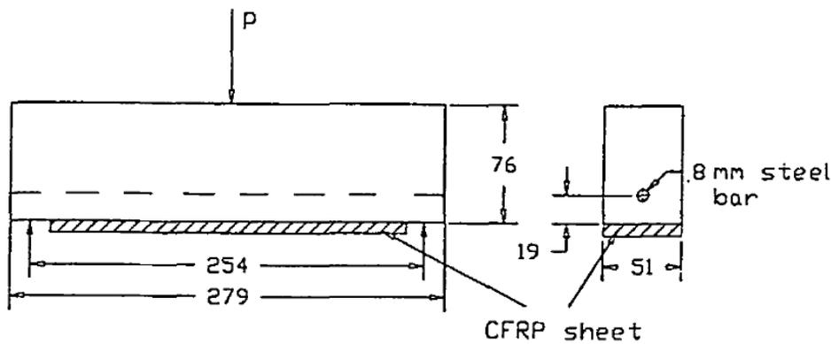
Figure 5—Three-point bending test setup (Xie et al., 1995)
