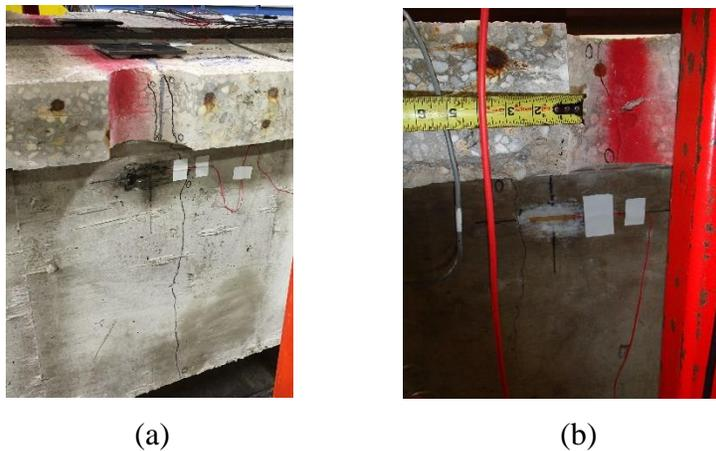
Figure 200—Reduced cross-section at midspan (Girder 5-2): (a) west elevation (b) east elevation
