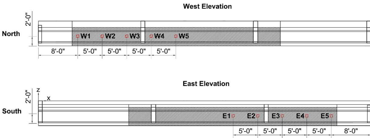
Figure 236—Direct pull-off testing locations for Girder 3
