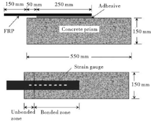
Figure 20—Direct shear test specimen (Pan et al., 2010)
