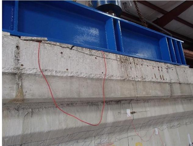
Figure 250—Concrete crushing in the compression zone
