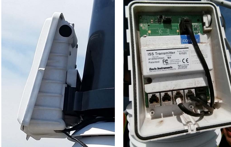
Figure 3-22. Davis Vantage Pro2 weather station sensor interface module.
