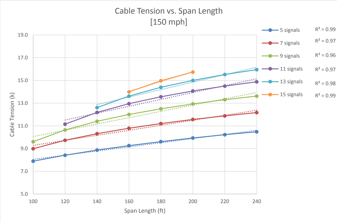
Figure 24 – GTS: 3 Headed Polycarbonate Signals, 150 mph, with Backplates
