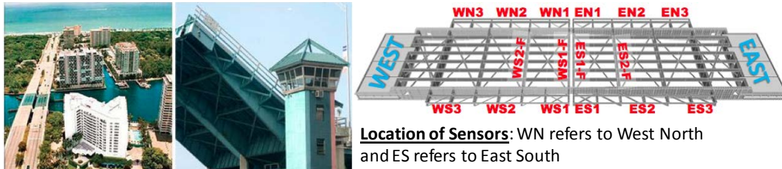
Figure 30-Sensor locations for structural components of Sunrise Boulevard Bridge
