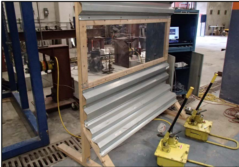
Figure 4-17. Hydraulic hand pumps used for torsion loading
