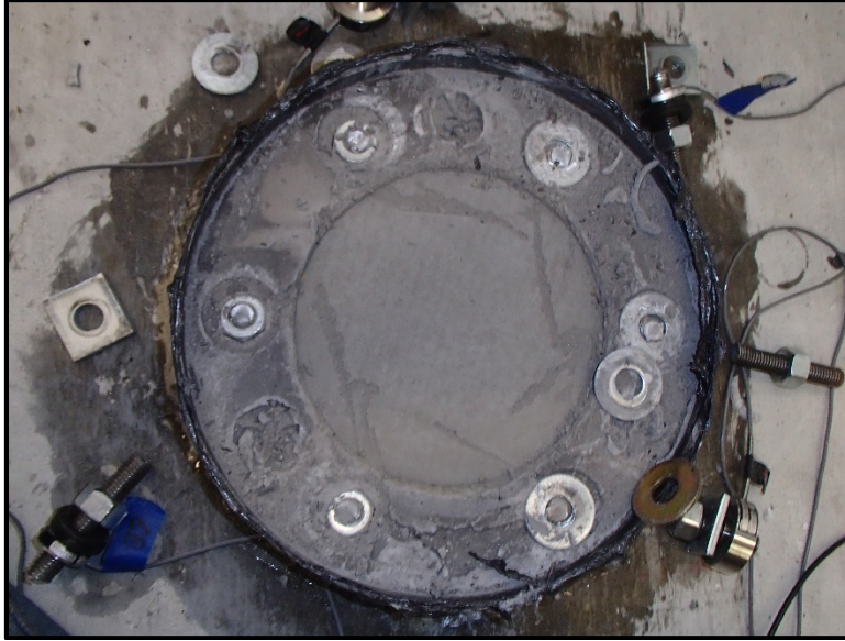
Figure 5-6. Post-test grout surface for T7 (FRP-retrofitted 4d_b base plate stand-off)
