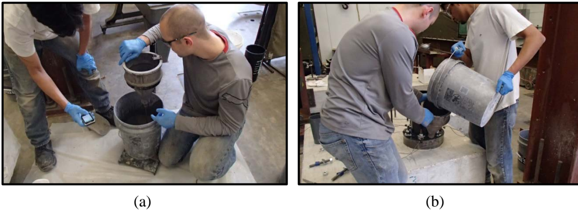
Figure 4-2. Performing the ASTM C939 flow cone test (a) and grout pad placement (b)
