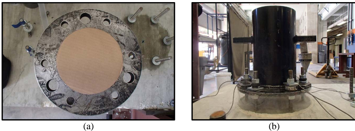
Figure 4-1. Cardboard separator (a) and Plexiglas formwork (b) for grouted tests
