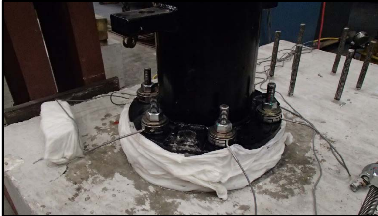
Figure 4-3. Grout pad and 2 in. cubes after wet-wrapping
