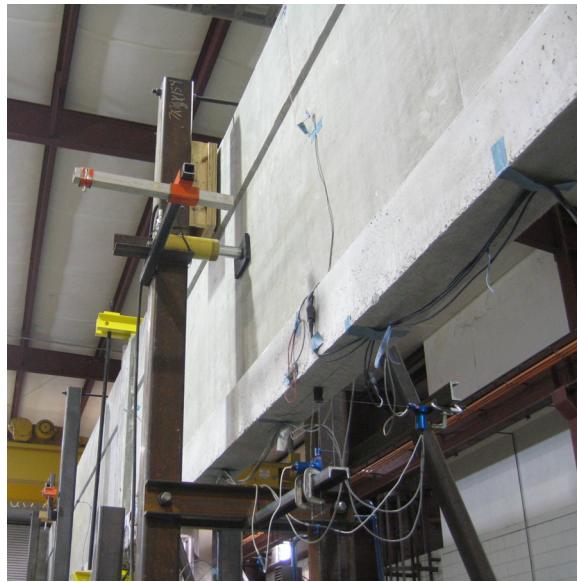
Figure 12.9. Jack used to straighten test girder
