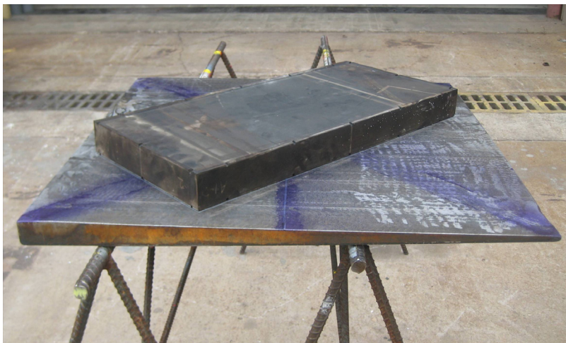
Figure 12.4. Beveled plate used to impose slope angle on bearing pads
