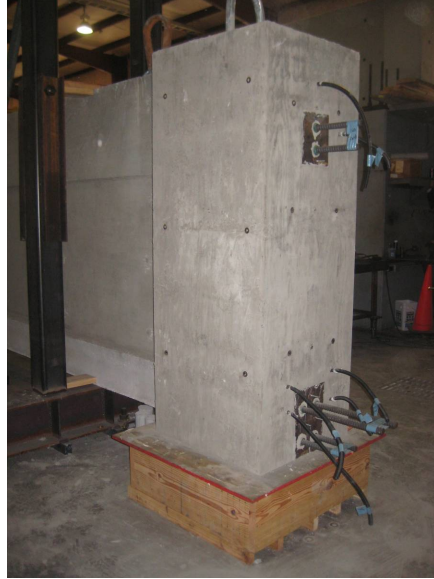
Figure 10.19. End block after removal of formwork
