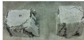
Figure 3.9 Block Batches after Failure
