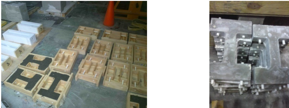
Figure 3.19 Fatigue Specimens during and after Casting
