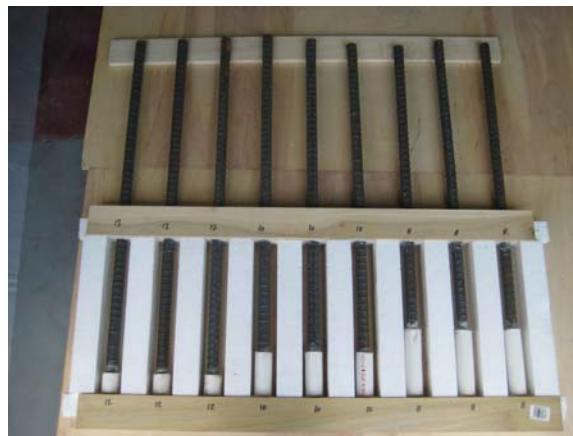
Figure 2.12 Pullout Test: (a) Schematics of Specimens and (b) Specimens Ready for Casting
