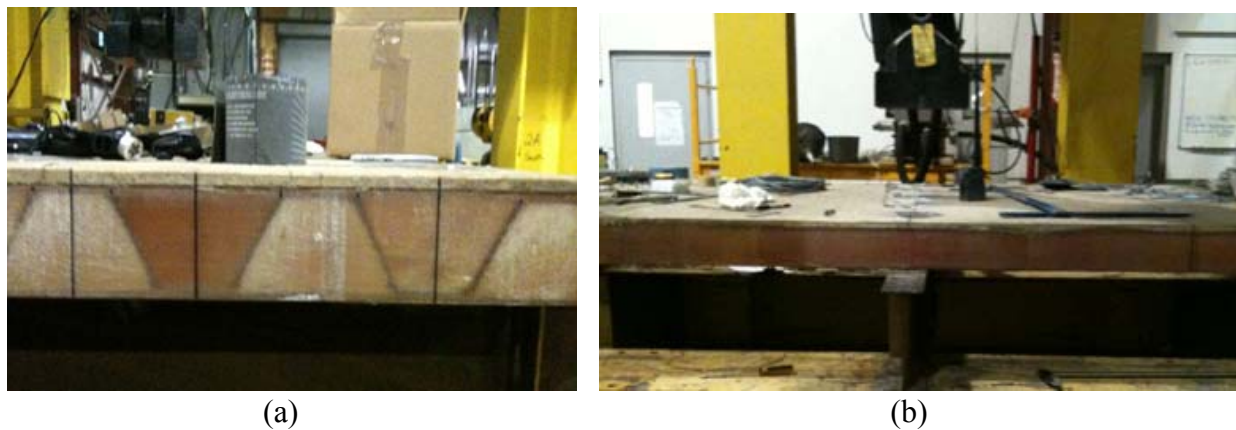
Figure 4.4 Tested FRP Deck System: (a) Cross-Section and (b) Elevation View
