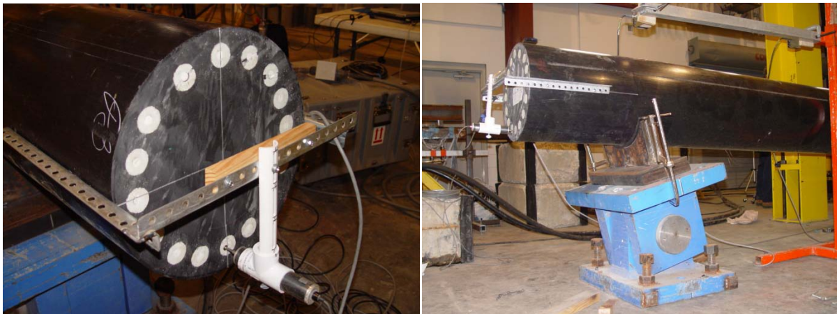
Figure 20: Deflection Gauge Setup for Detecting Slip of Reinforcement for CP Specimens
