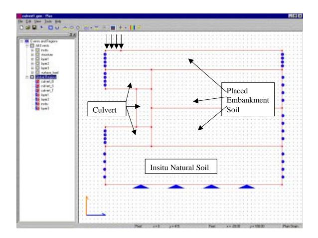
Figure 5.7 Concrete Culvert with Embankment and Surface Loading
