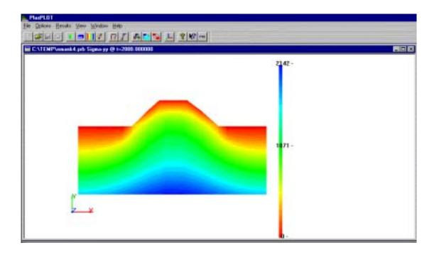
Figure 4.16 Plot of Vertical Stress for Event Three
