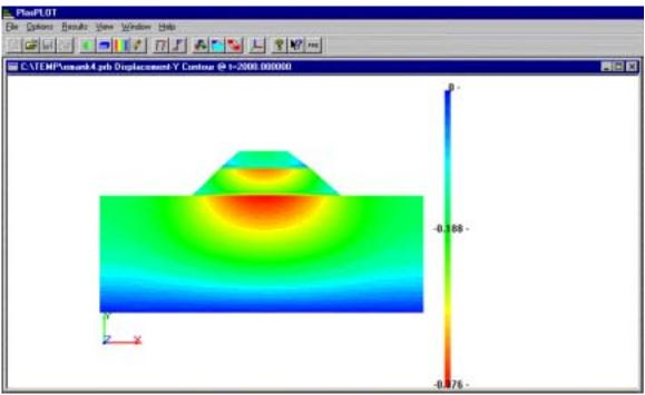
scale (color) for magnitude of settlement. The magnitude scale will always show the maximum and minimum identified in the "Contour Option", Figure 4.10.
