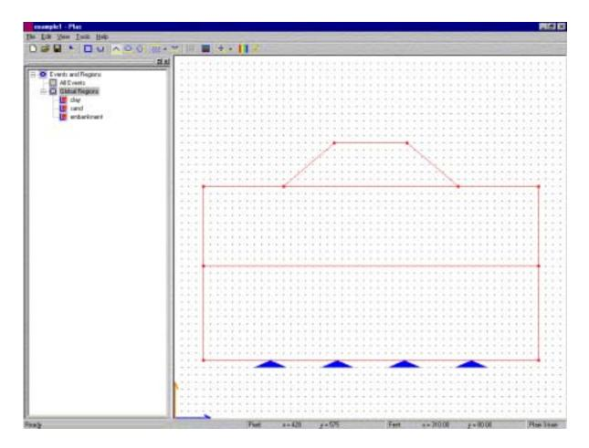
Figure 3.16 Placing Pins, Vertical and Horizontal Deformation Restraint
