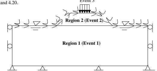
Figure 2.15 Modeling Consolidation with Boundary and Initial Conditions
