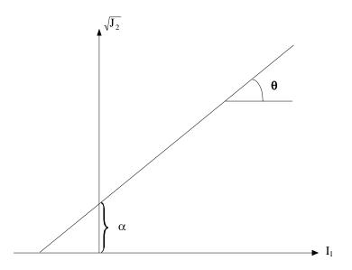
Figure 2.9 Elastic Perfectly Plastic with Straight Failure Surface
