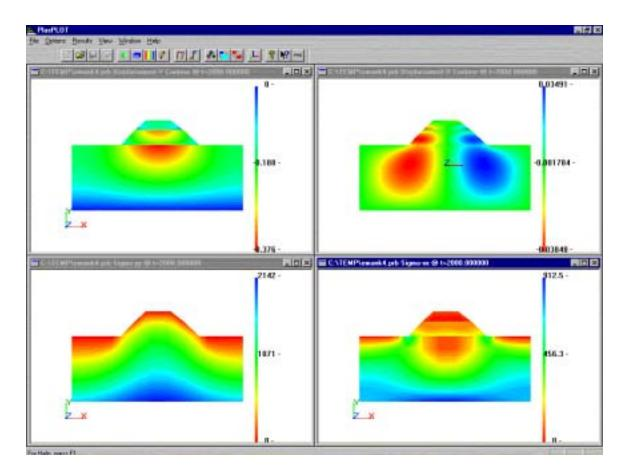
Figure 4.33 Multiple Displays of Displacements and Stresses
