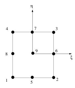
Figure 2.2 Variable 4 to 9 Node Plane Strain or Axisymmetric Element
