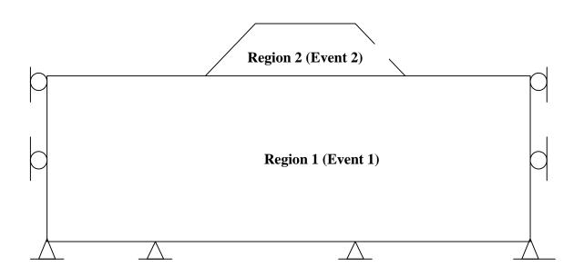
Figure 2.7 Embankment (Region 2) to be Placed in Event 2.
