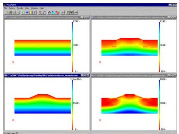
the placement of the second layer (70 days) or the complete embankment. The bottom left figure is the pore pressure in the soil mass at 70 days.
