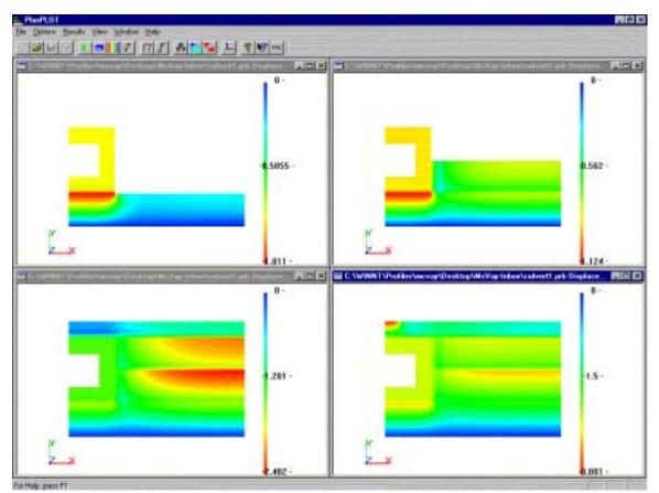
and culvert after a surface pressure of 45 psi is applied to the centerline of the culvert.
