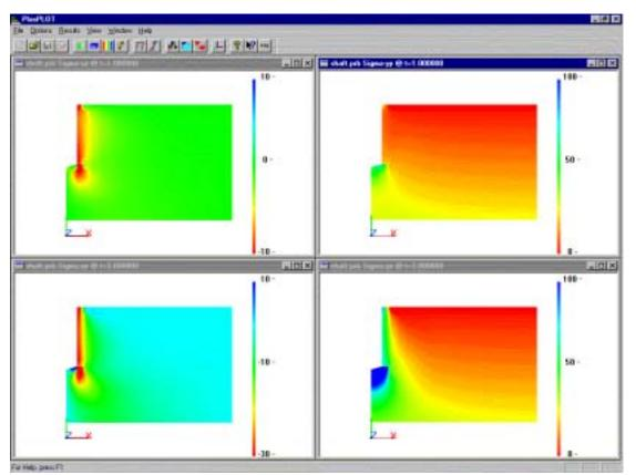
Figure 5.12 Shear and Vertical Stress in Soil Mass
