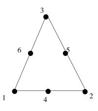
Figure 2.3 Six Node Plane Strain or Axisymmetric Element
