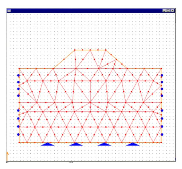
Figure 3.40 Triangular Mesh Generation
