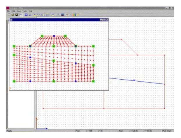
Figure 3.44 Meshed Regions with Inclusion of Water Table
