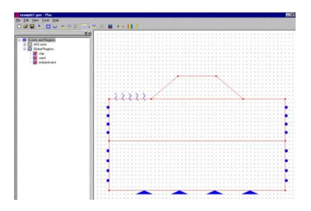
Figure 3.18 Assigning Flow or Zero Pore Pressure at Boundary
