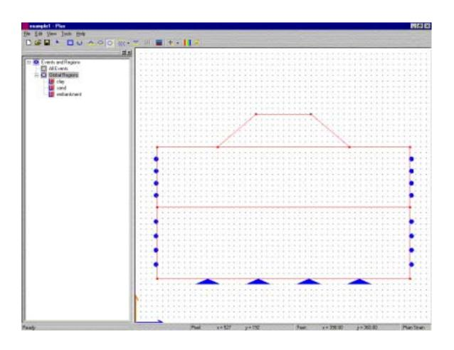
Figure 3.17 Placing Vertical Rollers (Zero Lateral Movement) on Right Boundaries
