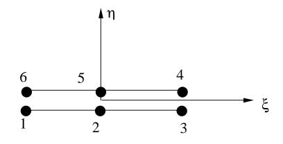
Figure 2.5 Six-Node Interface Element
