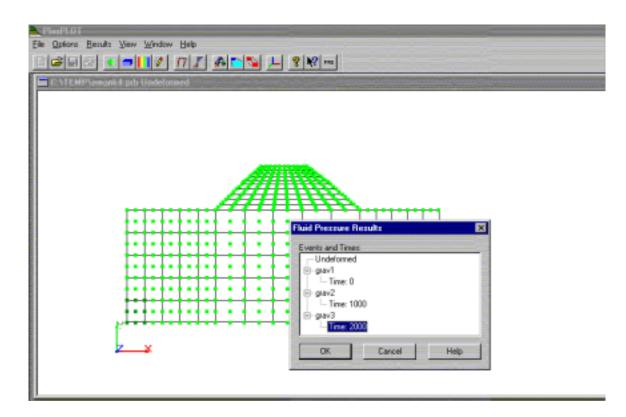
Figure 4.18 Selecting Pore Pressures to View
