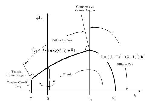
Figure 2.11 Sandler-DiMaggio Model (Elastic-Plastic)
