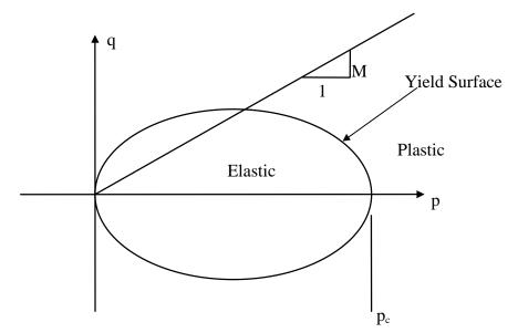
Figure 2.12 Yield Surface (i.e., Elastic vs. Plastic Strains)
