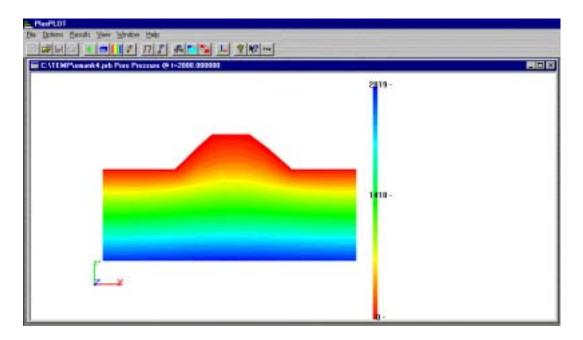
Figure 4.19 Pore Pressure Distribution and End of Construction
