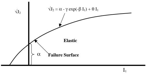
Figure 2.10 Elastic Perfectly Plastic- Curved Failure Surface
