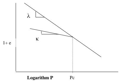
Figure 2.14 Relation between Void Ratio and Mean Stress
