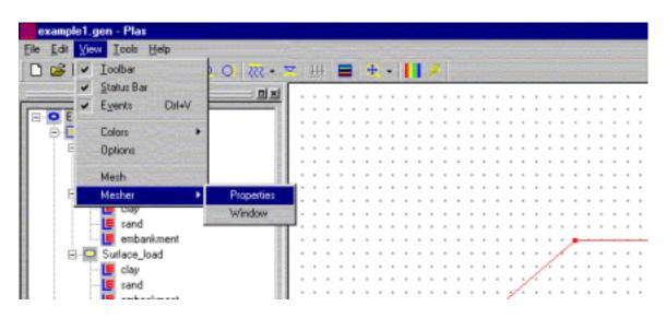
Figure 3.33 Selecting Quadrilateral or Triangular Mesh
