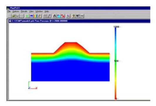
Figure 4.20 Changing Scale on Pore Pressure Distribution
