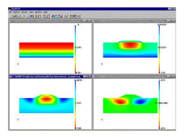
Figure 5.3 Embankment Displacement Results
