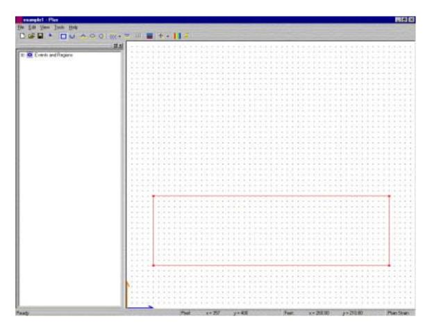
Figure 3.8 Using Rectangle Option to Construct a Soil Layer
