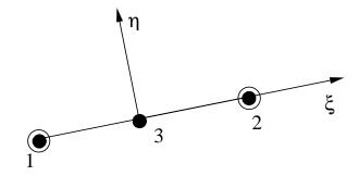
Figure 2.1Variable 2 or 3 Node Truss Element
