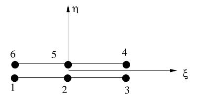
Figure A.7 Six-node Interface Element
