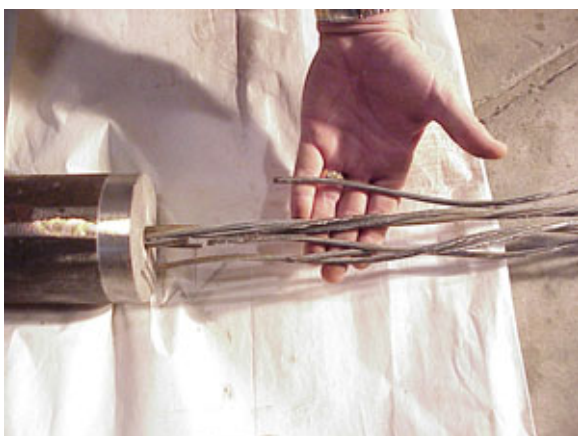
Photo 17 – Failure of Corroded Specimen #6
