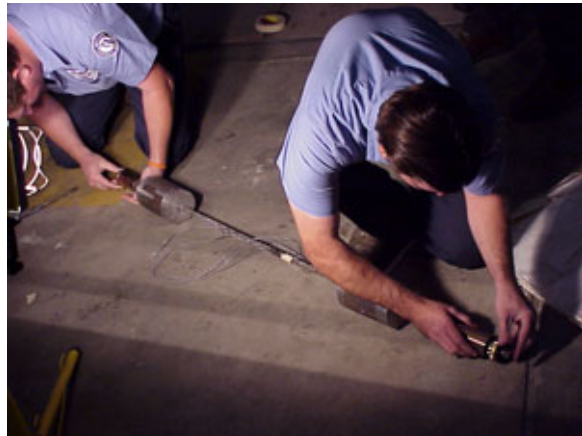
Photo 8 – Insertion of Specimen in Chucks
