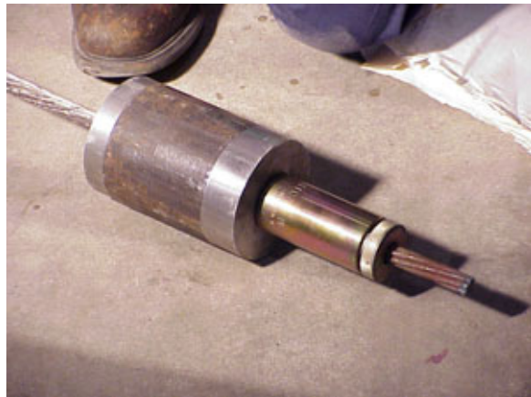
Photo 10 – Chucked Specimen With Blocking Sleeve Installed
