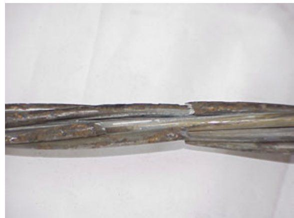
Photo 16 – Failure of Corroded Specimen #5
