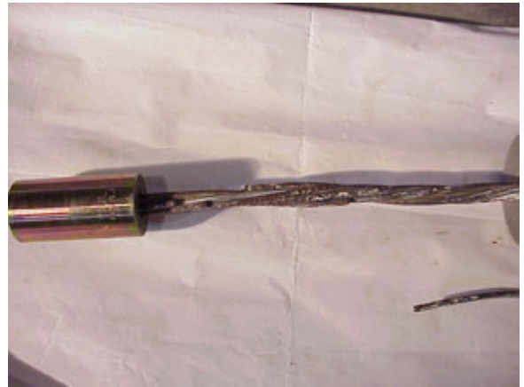
Photo 14 – Failure of Corroded Specimen #2
