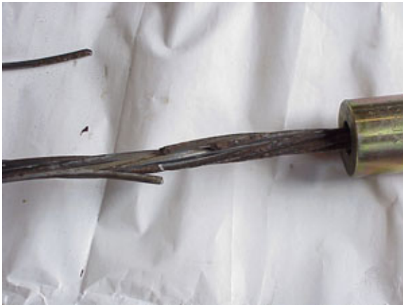
Photo 13 – Failure of Corroded Specimen # 1
