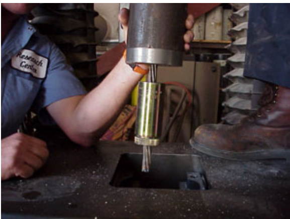
Photo 11 – Blocking Sleeve Being Placed Into V-Grips
