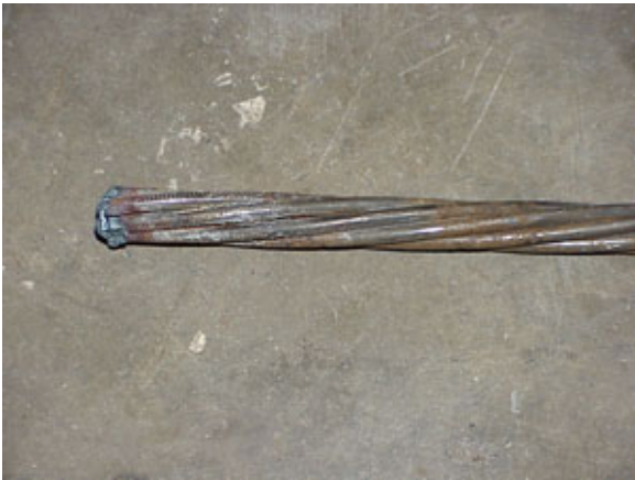
Photo 7 – Strand After Removal From Wedge
