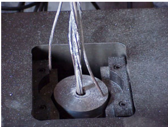
Photo 15 – Failure of Corroded Specimen #3
