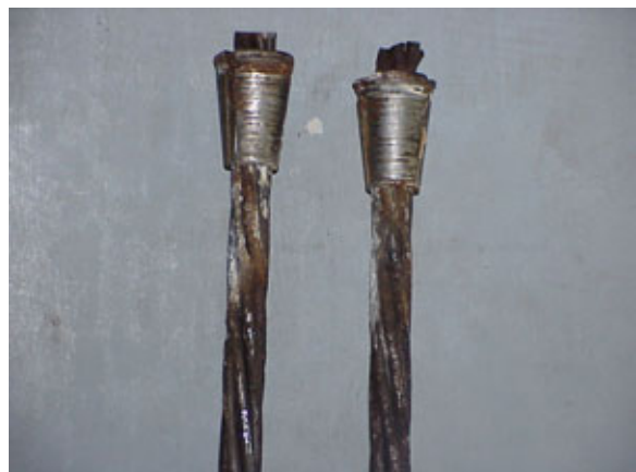
Photo 6 – Strand Ends After Removal From Anchor
