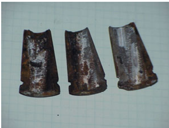
Photo 3 – Anchor Wedges With Corrosion
