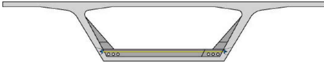
Figure 2.18 – Transverse Post-Tensioning in Deviation Ribs
