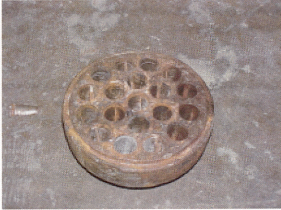
Photo 1 – End View of Anchor Plate
