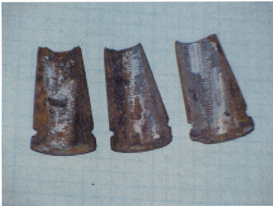
Photo 3 – Anchor Wedges With Corrosion
