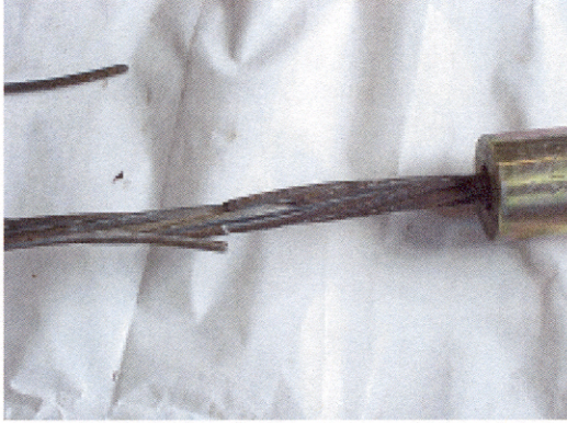
Photo 13 – Failure of Corroded Specimen #1
