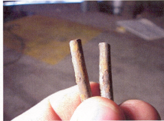
Photo 4 – Close-up Of Pitting Corrosion
