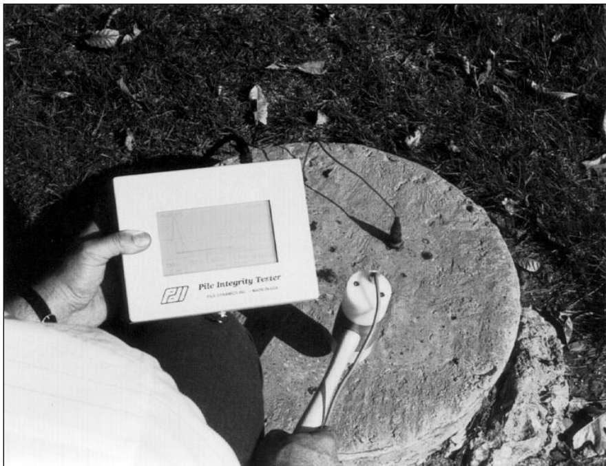
Figure 39, Pile Integrity Tester (After PDI, 1993)
