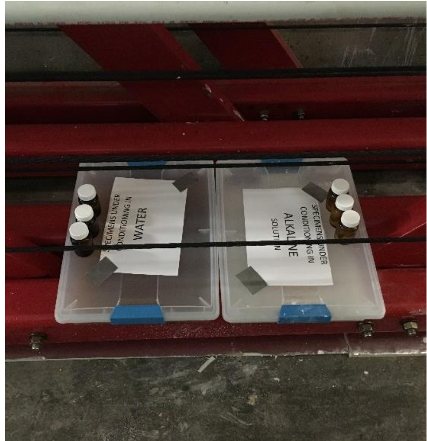
Epoxy coupons and fibers subjected to water and alkaline solution at high temperature.
