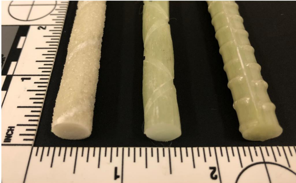
Helical Wrap + Sand (type A), Helical Wrap (type B), Helical Rib (type C)
