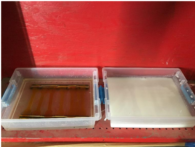
Epoxy coupons and fibers subjected to water and alkaline solution at 77 °F.
