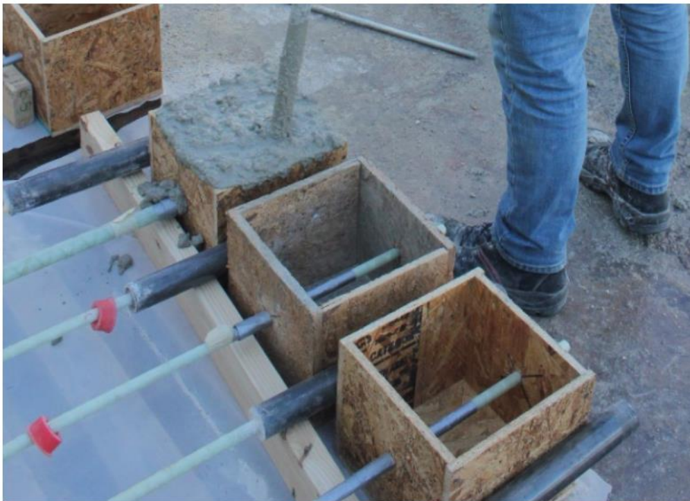
Figure 2: Concrete casting (left) and grip installation (right)
