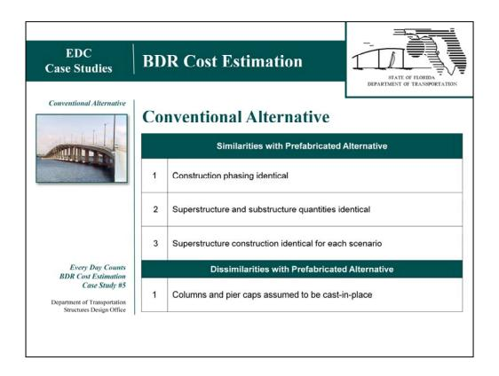
> This slide will detail the conventional construction alternative. For comparison with prefabricated construction, the following assumptions will be made:
