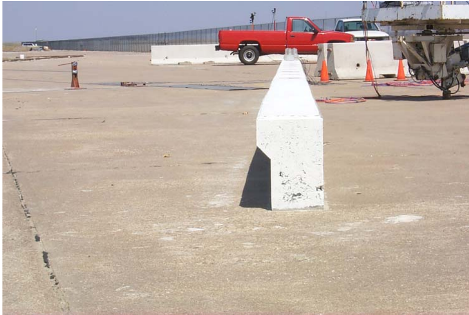
FIGURE 110 Two low-profile concrete barriers have passed NCHRP Report 350 test-level 2 (45 mi/hr) crash testing.
