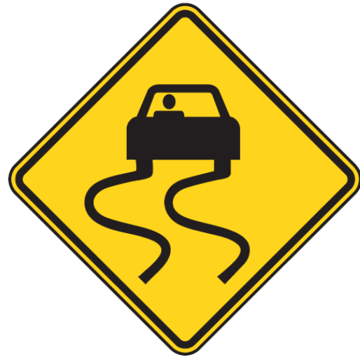
FIGURE 61 SLIPPERY WHEN WET sign.
