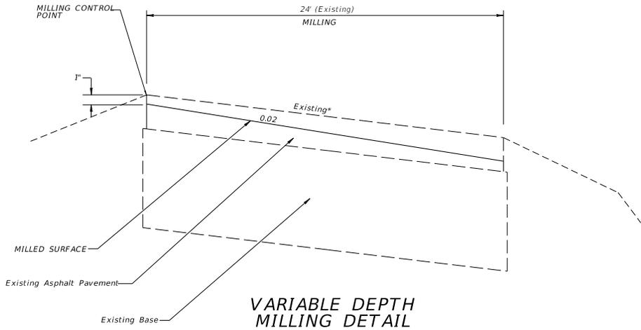
**VARIABLE DEPTH MILLING DETAIL**
