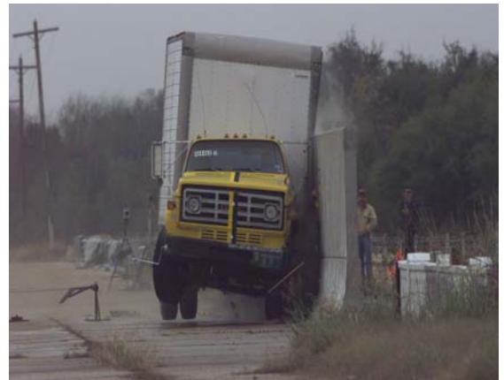
Test Level 4 (TL-4) Crash Test of the Florida Bridge Sound barrier
