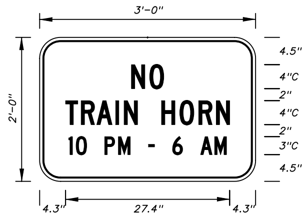
FTP-61-06 3' X 2' 3" Radii 3/4" Border 4" and 3" Series C Legend Yellow Background Black Legend and Border Design Project Manager or Transit Administrator will supply correct 1-8XX number.
