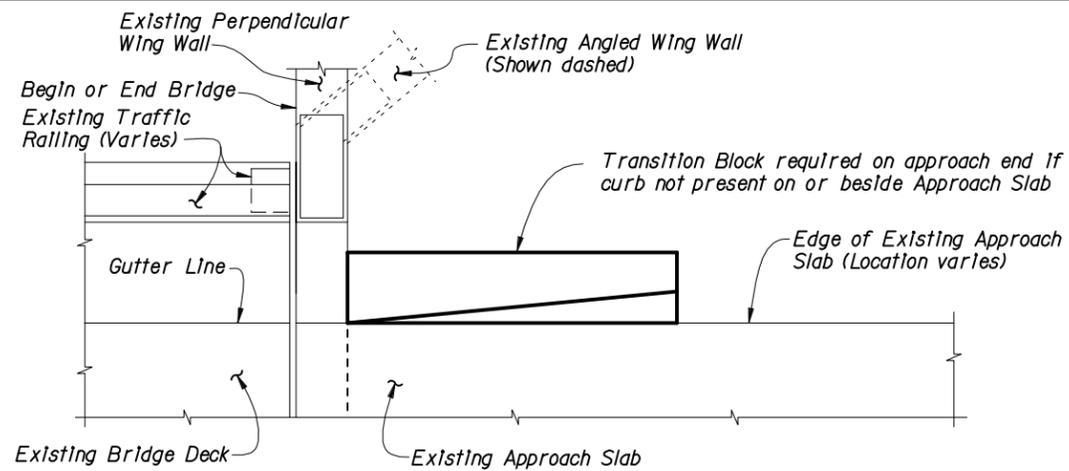
**PARTIAL PLAN VIEW OF EXISTING BRIDGE WITH PERPENDICULAR OR ANGLED WING WALLS**
