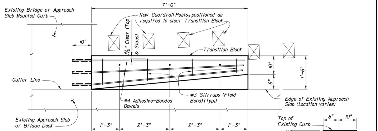
**PLAN VIEW OF TRANSITION BLOCK (GUARDRAIL NOT SHOWN FOR CLARITY)**
