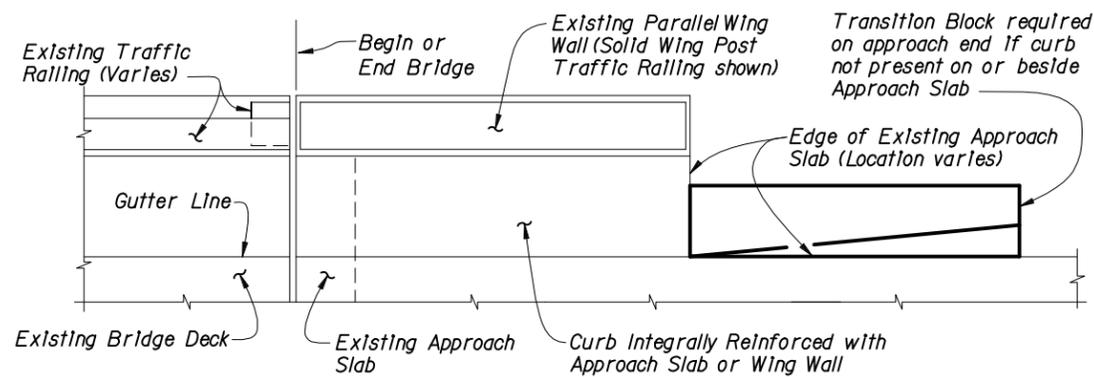
**PARTIAL PLAN VIEW OF EXISTING BRIDGE WITH PARALLEL WING WALLS AND INTEGRALLY REINFORCED APPROACH SLAB CURBS (APPROACH SLAB WITH DETACHED CURBS OR SIDEWALK SIMILAR)**
