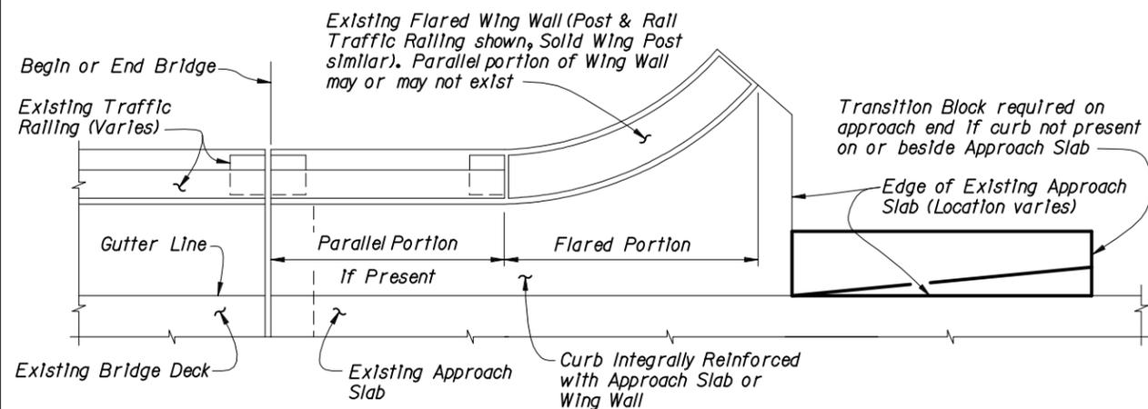
**PARTIAL PLAN VIEW OF EXISTING BRIDGE WITH FLARED WING WALLS AND PARALLEL INTEGRALLY REINFORCED APPROACH SLAB CURBS (APPROACH SLAB WITH DETACHED CURBS OR SIDEWALK SIMILAR)**
