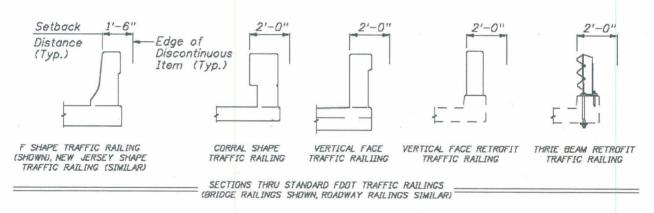
Fender access ladders are exempt from this requirement. Sign panels may be placed within the given setback distances, however the setback to the sign support may have to be increased to assure sign panels do not extend past the top inside face of the traffic railing. Motorist aid call boxes may be placed within the setback distances to allow for proper access and to meet ADA requirements, however the call box must not extend past the top inside face of the traffic railing.
