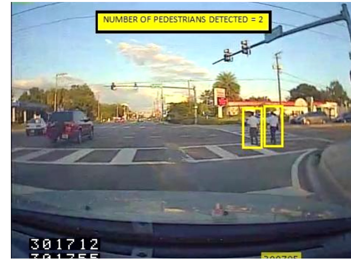
The Automatic Video Processing Tool (AVPT) identifies pedestrians (left) and red traffic signals (right) in segments of video from the NDS. These segments will be flagged for review and analysis by the researchers.
