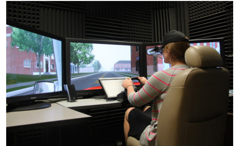
A participant wearing an eye-tracking device in the driving simulator portion of the project navigates the how-to tutorial before tackling the countermeasure scenarios.
