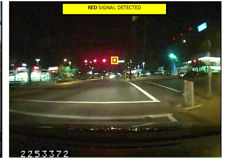
The Automatic Video Processing Tool (AVPT) identifies pedestrians (left) and red traffic signals (right) in segments of video from the NDS. These segments will be flagged for review and analysis by the researchers.
