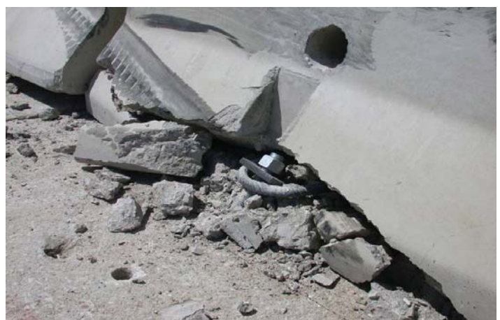
Above: Close-up view of K-barrier damaged in the MwRSF crash test.
